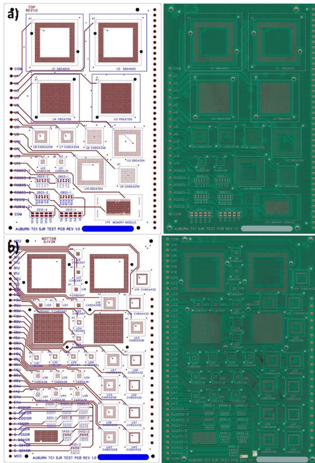
**Figure 1.** Test Vehicle Design: a) Top-Side and b) bottom-side of the TC1-SRJ test vehicle.
