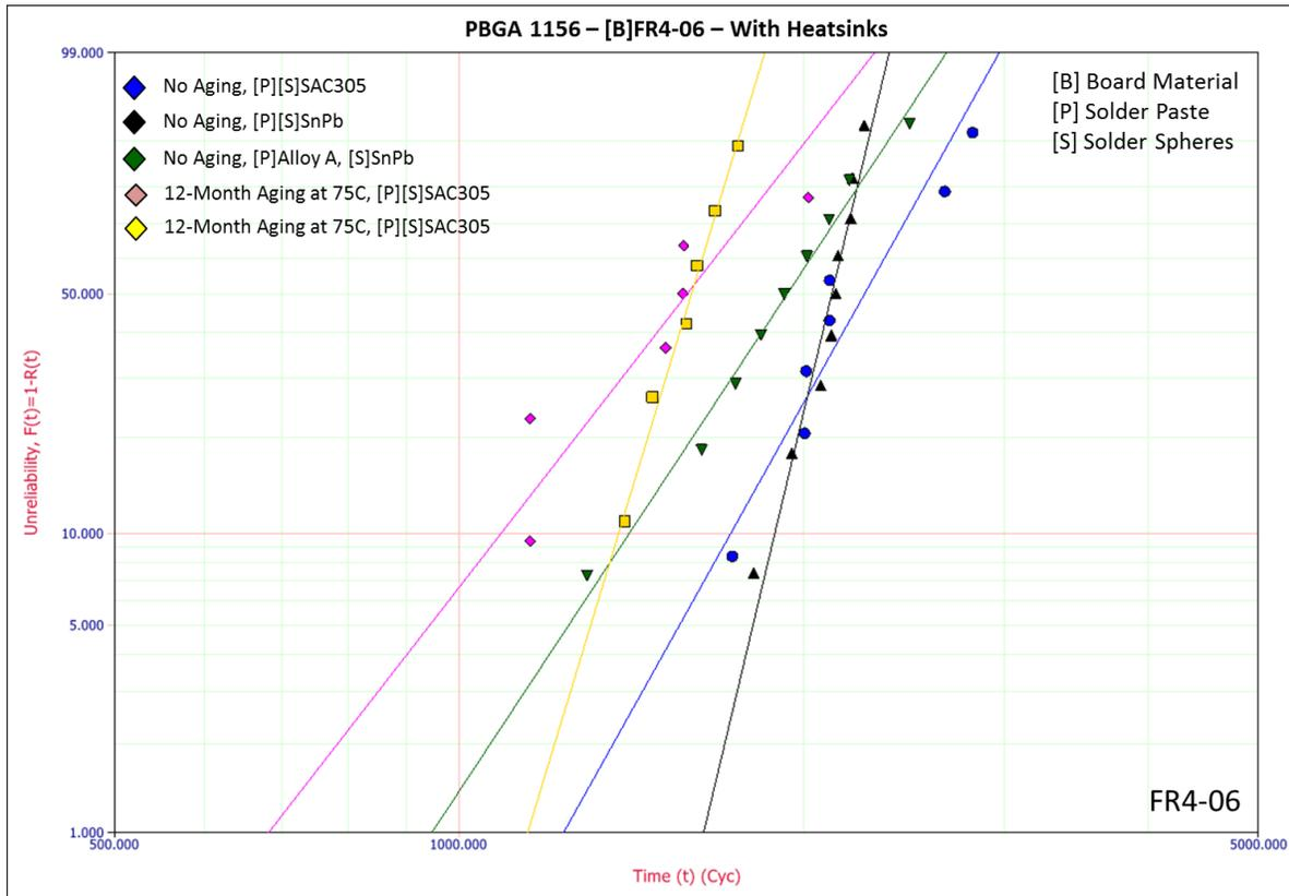
**Figure 12.** Weibull Plot: PBGA1156 – No Aging and 12-Month (75°C)
