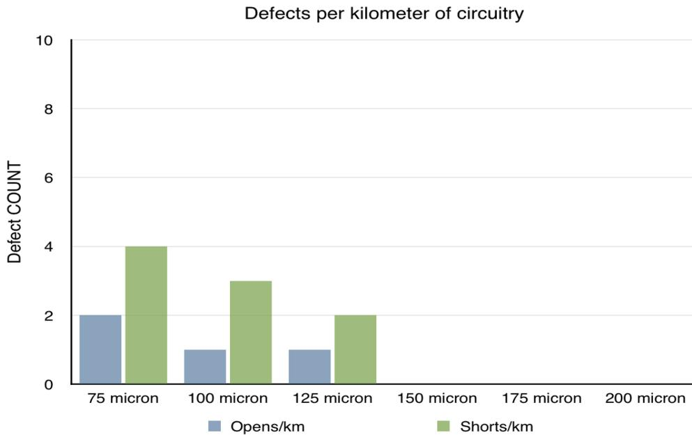
**Fig 26 – Defect per kilometer of circuitry on CAT test patterns**
