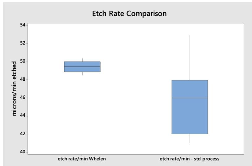
Figure 21 – Etch Rate Comparison (Recycled versus Traditional Alkaline Etch)
