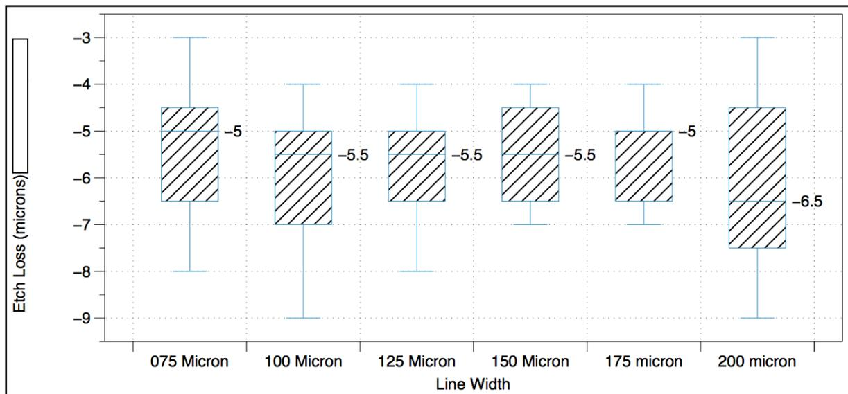
Fig 25 – Range of average etch loss on CAT test patterns by conductor width
