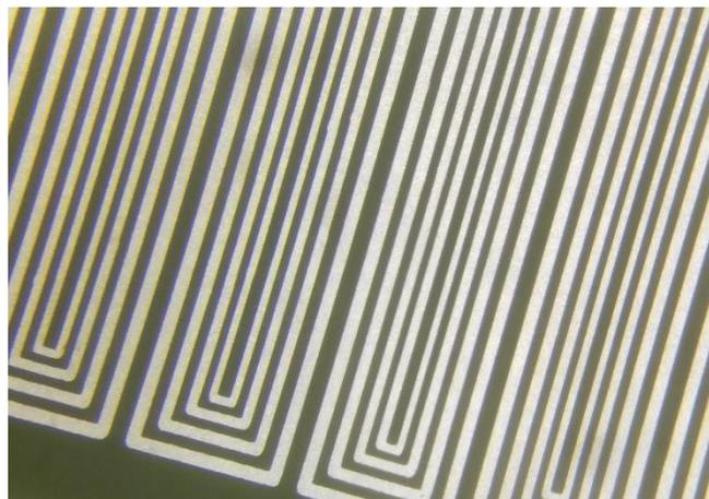
**Fig 27 – Example of Etched CAT test vehicle**
