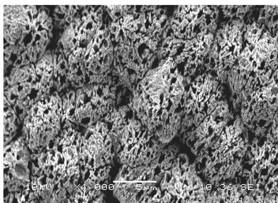
4000x ED Cu treated with micro etch
