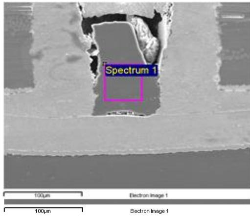
Figure 23: Example of dry film chip plugging a via filled hole.
