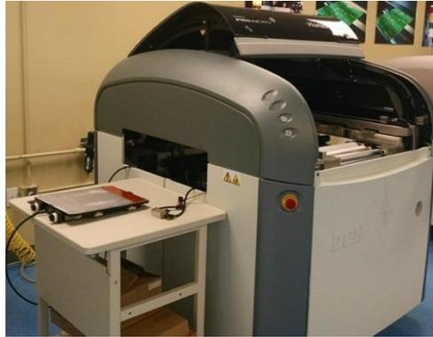
Figure 3: Production screen printer.
