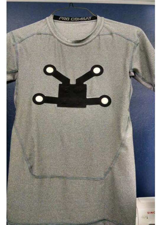
Stretchable ECG Sensor laminated to compression shirt (Source: Company)
