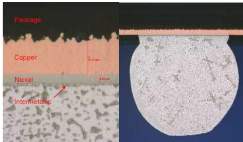
**Figure 16 - Cross Section SN 47, Reballed 10 X**
