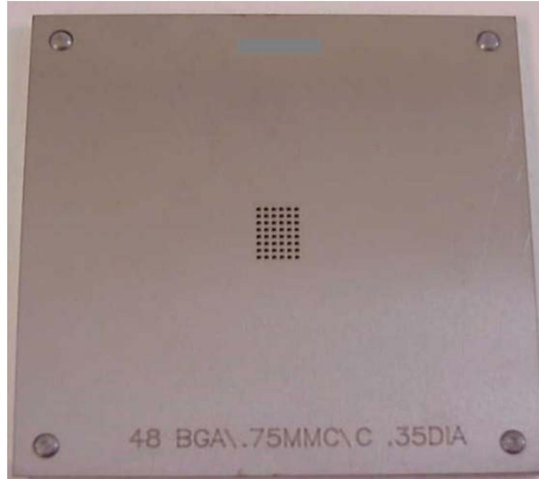
Laser etched stencil secured to mobile platform. Spheres corralled perfectly to pad centers though the reflow process. Process speed can be easily increased by the ability to scale platform as desired to reball multiple units simultaneously. There is no need for solder paste due to existing deposit.
