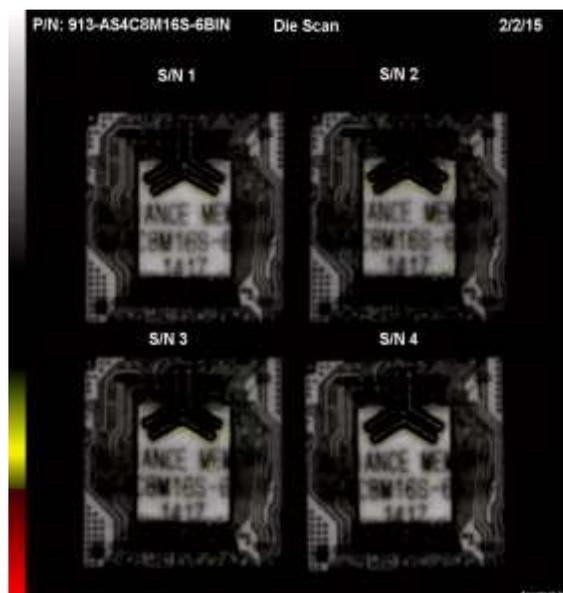
**Figure 13- Pre process view, Top of Die, C-mode image**
