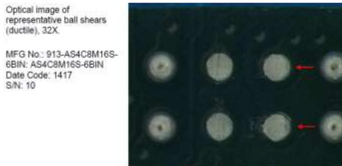
Figure 19 – Example of Sheared Balls
