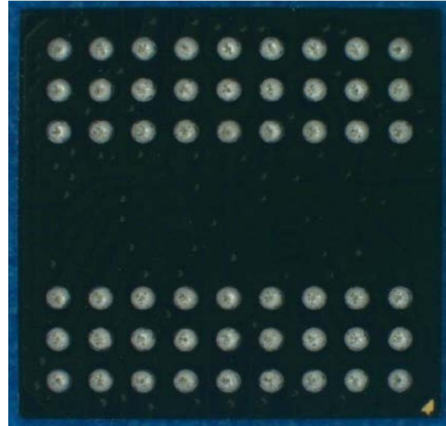
54 Ball TFBGA (Thin and Fine Pitch Ball Grid Array). BT Substrate with mold encapsulated die and bonds. Original balls SAC 305, 0.018 inch (0.45MM) width at receipt. Replacement balls Sn63Pb37. Pads are nickel over copper. Parts reballed. Tests conducted follow.
