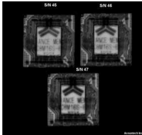
**Figure 14- Post process view, Top of Die, C-mode image**
