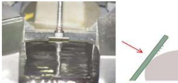
**Figure 5 – Solder Ball Removal at the Edge of Wave**
