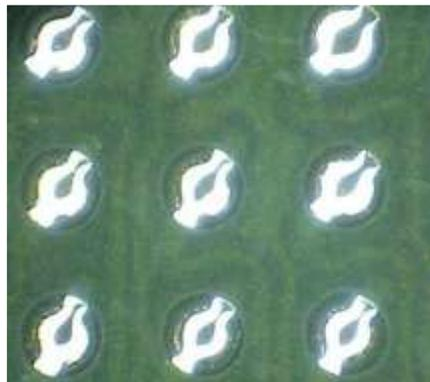
**Figure 7 – Pad Surfaces Post Robotic Solder Dip**
