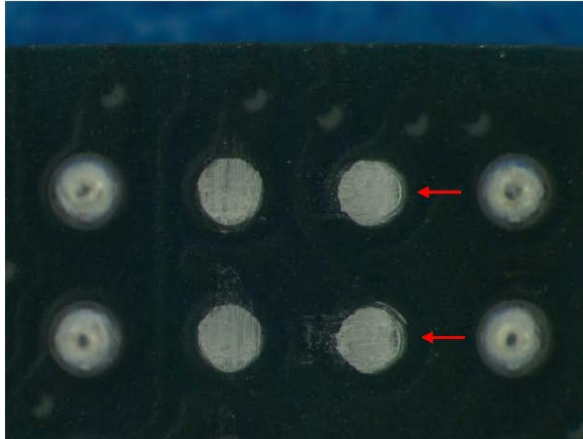
**All Shear Test Results Ductile (Required Result)**
