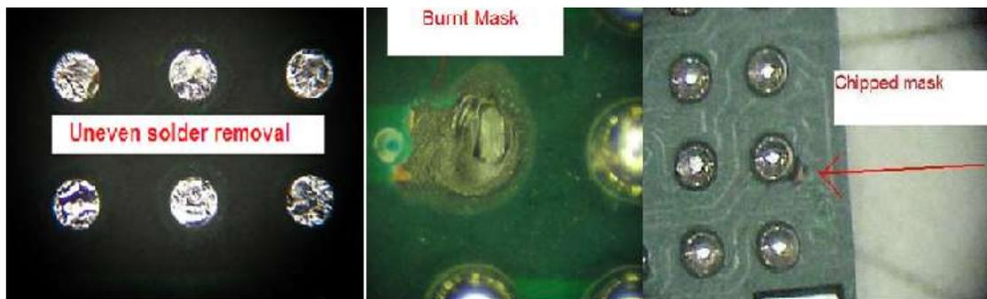
Figure 3 – Damage from Hand-Held Tools.
