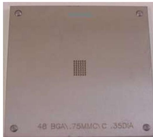
**Figure 9 – Laser Etched Stencil in Place to Align Solder Spheres to Component Pads**
