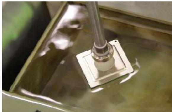
**Figure 6 – Water Wash - Flux Removal**
