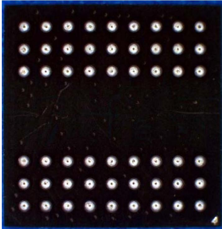
After multiple reballs cycles, ball luster is unchanged
