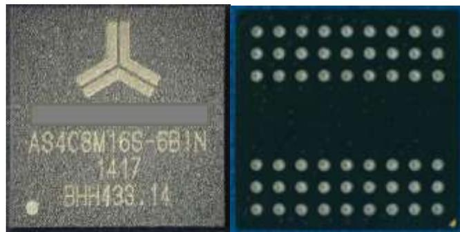
Figure 1–Top Side of Reball Vehicle    Figure 2- Bottom Side of Reball Vehicle
