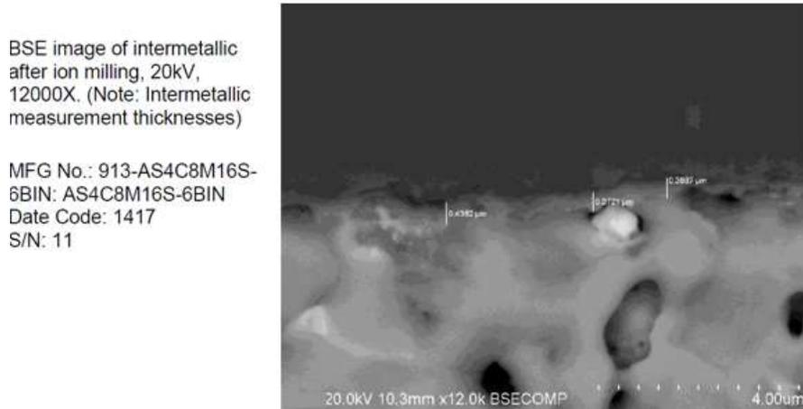
**Figure 17 – Close up Image of Intermetallic.**
