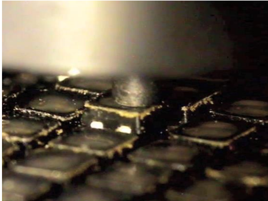
Single LED Desoldered and Removed
