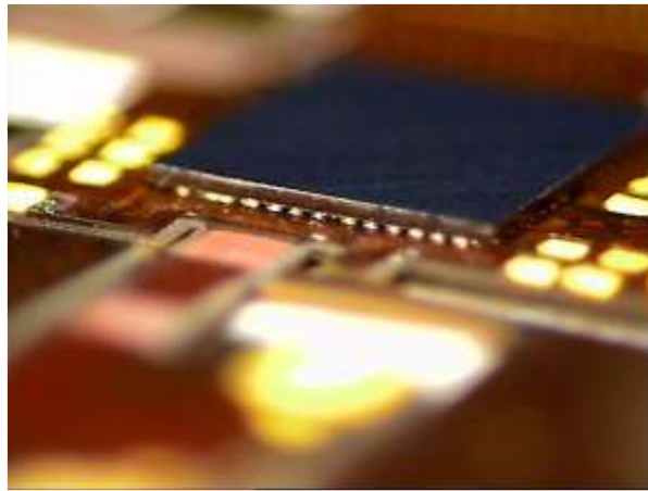
Figure 14 - C4 Flip chip soldered to a flex circuit
