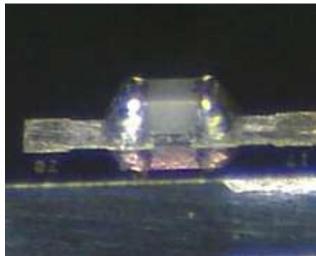
Figure 9 – Assembled beam lead diode
