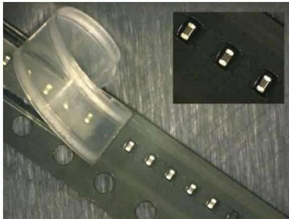
Figure 5 – Micro-passives housed in peel-away tape
