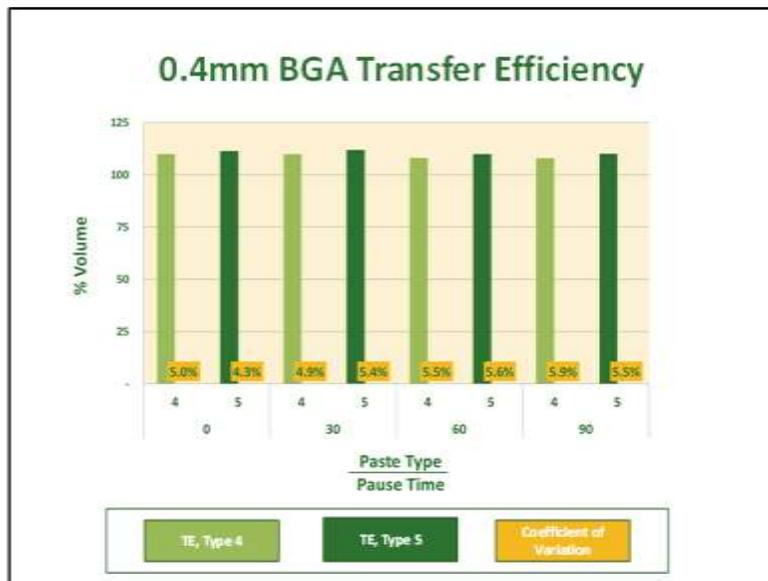
**Figure 10 - 0.4 mm device TE and CV by paste type over Time for copper defined pads**
