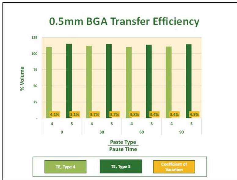
**Figure 8 - 0.5 mm device TE and CV by paste type over time on copper defined (NSMD) pads**
