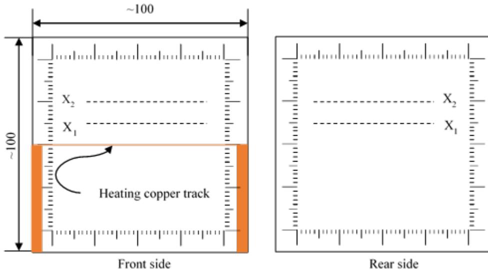
**Figure 6: Transient fin sample design**
