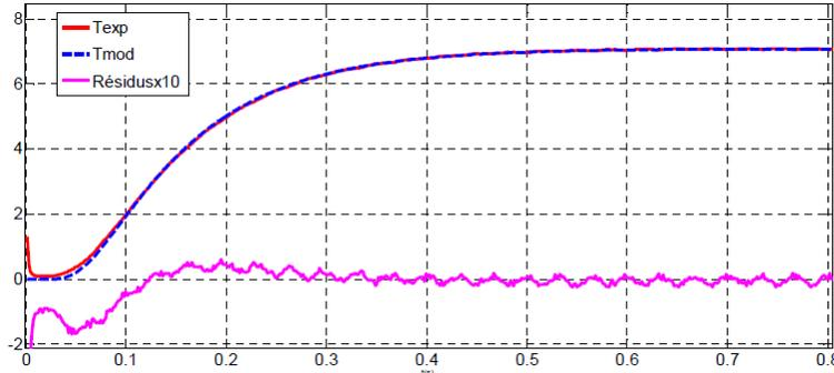
Figure 9 : Example of the theoretical and experimental thermogram by the flash method
