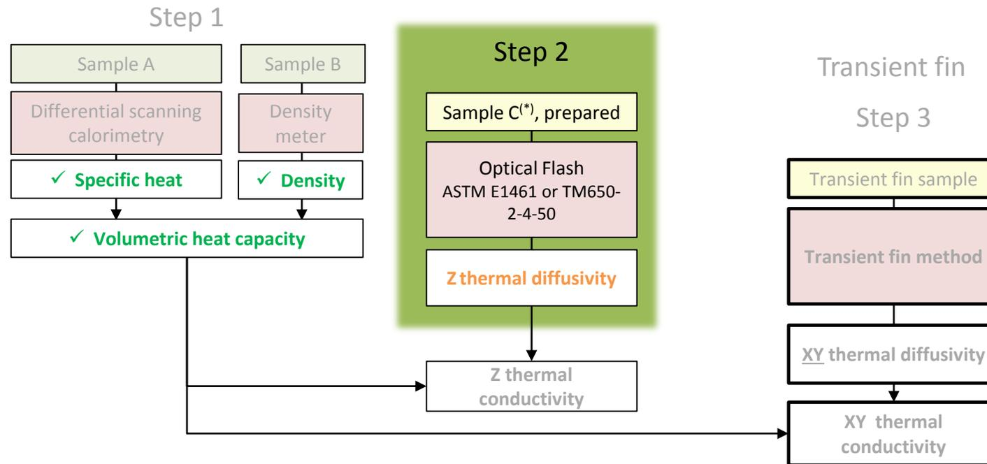
(\* ) Sample C to be prepared according to ASTM E1461 or TM650-2-4-50
