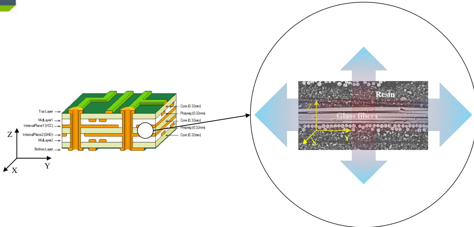
Note: From a mechanical and thermal prospective, laminates and prepregs are **anisotropic** materials
