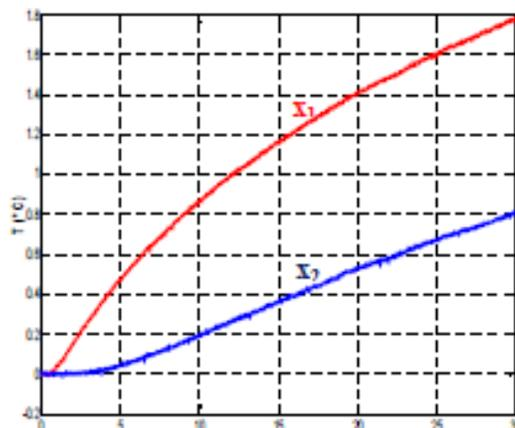
Figure 11 : Example of the thermograms at  $x_1$  and  $x_2$  distances
