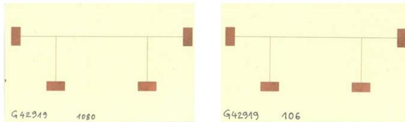
Figure 10: 106 and 1080 test samples for the transient fin method
