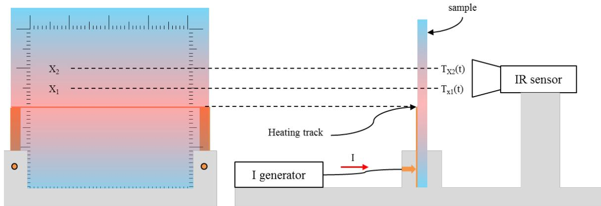
**Figure 7: Transient fin sample method apparatus example**
