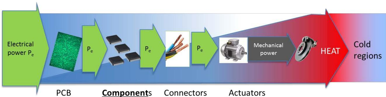
Heat is generated all along the chain. At the electronic system level, the main contributors are often components. The printed circuit board, supporting and interconnecting them, is also very helpful to avoid system excessive heating. Indeed, excessive temperatures degrade overall system performance, from speed to long term reliability. Therefore, electronic system designers take great care of operating temperatures. Equations managing thermal exchanges can be easily found in the literature.
