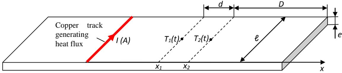
**Figure 4: Transient fin method principle**
