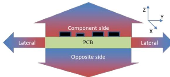
**Figure 2: Printed circuit board thermal management possibilities**
