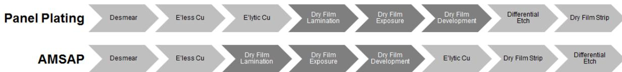
**Figure 3: Process flow comparison of Panel Plating and AMSAP technologies**
