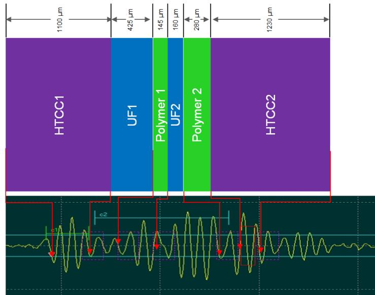
**Figure 6. Echo pulse-train of the multilayer sample impinged with 100MHz acoustic wave packet. The arrows indicate the timed locations of each interface. Waveform sampling rate is 4GHz, and time resolution is 0.5ns. Also note that HTCC and Polymers are multilayer stacked-ups.**
