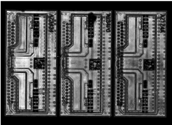
**Figure 7(f). C-scan image from Gate #6, top of HTCC2 at 100MHz probe frequency.**
