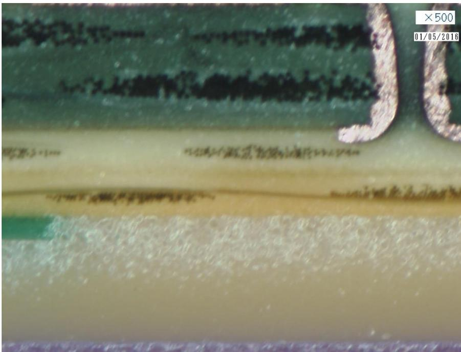
**Figure 9. Cross section image of center region with 500x optical microscope, the lower level delaminations are somewhat difficult to distinguish by optical cross sections.**
