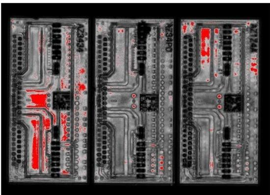
Figure 7(d). C-scan image from Gate #4, top of UF2 at 100MHz probe frequency. Both Left and Right units show significant delamination or less dense material regions as highlighted by red color. UF1 and some part of UF2 have flaws.
