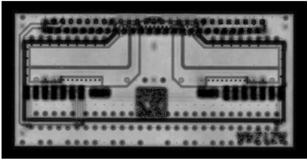
**Figure 2(a).** Image of Underfill layer 1 focused with a 50MHz probe frequency. This layer includes solder ball connections between adjacent layers. The big square shadow is laser marking and smaller rectangular shadows are surface mounted components.
