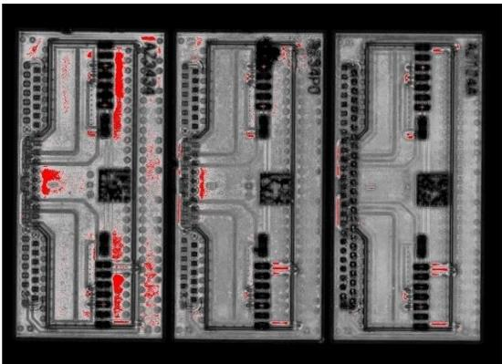
Figure 7(c). C-scan image from Gate #3, UF1 and polymer 1 Interface at 100MHz probe frequency. The inspection algorithm is set so that red color paint will highlight whenever a delamination or void is detected. Serious flaws can be seen in the left middle of the left most unit possibly from UF1.
