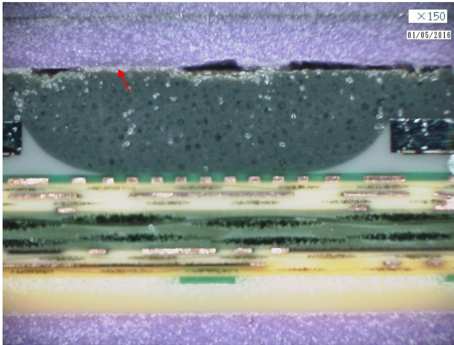
**Figure 8. Cross section image of center region with 150x optical microscope**
