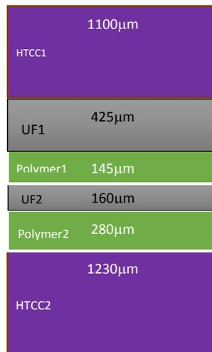
**Figure 1. Illustration of material structure of the sample and their thickness in micrometer. Outer layers are high temperature co-fired ceramics.**
