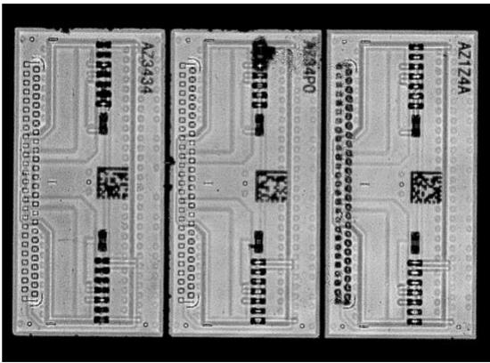
Figure 7(a). C-scan image from Gate #1 representing bottom layer of HTCC1 at 100MHz probe frequency. All 3 units show very similar images, except the shadow of misplaced surface mount condenser is seen differently at the center unit.
