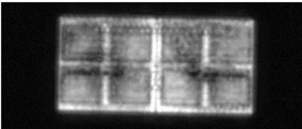
**Figure 5(a)** Through transmission scan with 15MHz
