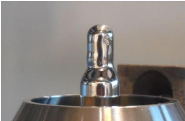
Smaller nozzles require high solder temperatures: Typical  $>300\text{ }^{\circ}\text{C}$
