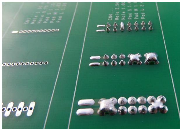
**Figure 11: pad diameters 2.4, 1.9 and 1.4 mm and its sensitivity for bridges.**
