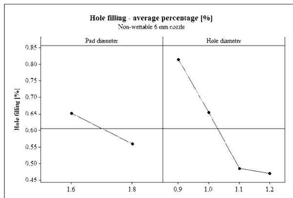
**Figure 7: Hole filling [%] for a 6 mm non-wettable nozzle**
