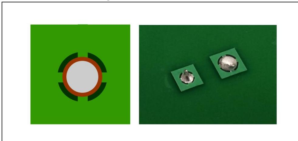
**Figure 9: Thermal relief and solder mask**
