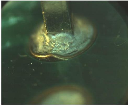
**Figure 8: Pad lifting**
