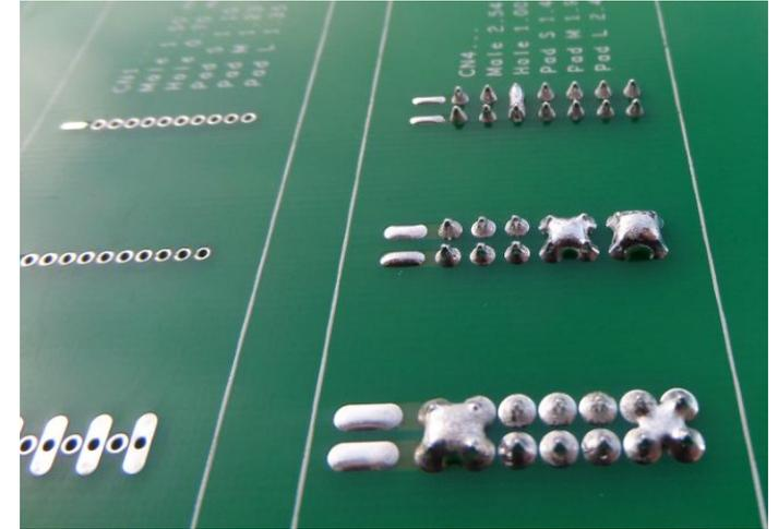
None of parameters has significant impact on bridging; only pad diameter
