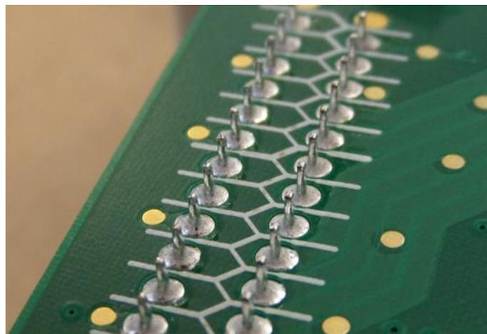
**Figure 12: Dedicated silkscreened lines break the capillary force of the solder and discourage bridging**
