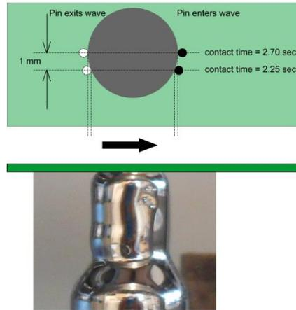
**Figure 2: The impact of soldering out of center: shorter contact time for the pins.**
