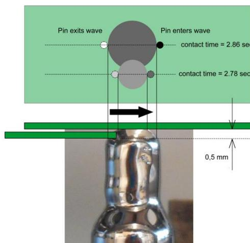
**Figure 3: The impact the immersion depth – deeper in the solder longer contact.**
