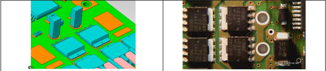
Figure 13: D-Pak with leads 0.5 mm from the barrel on the solder destination side
