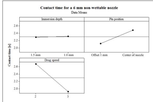
**Figure 4: Factorial Plot of 6 mm non-wettable nozzle, showing the effect of parameters on contact time.**
