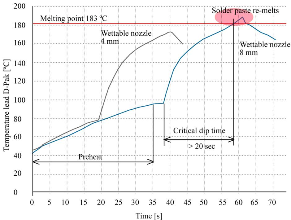
Figure 14: Even with an 8 mm wettable nozzle, it takes more than 20 seconds to re-melt the solder paste
