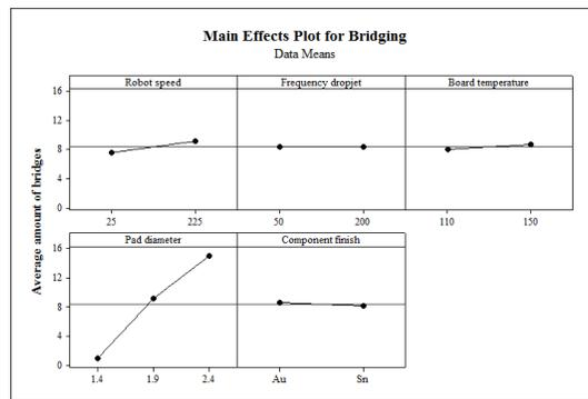
**Figure 10: The smaller the pad on the solder side, the less bridging**
