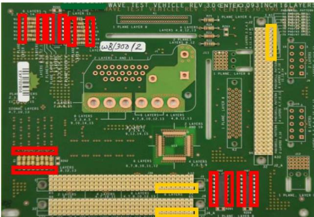
8 Layer FR4, 64 Pin connector, diameter 0.65 mm
