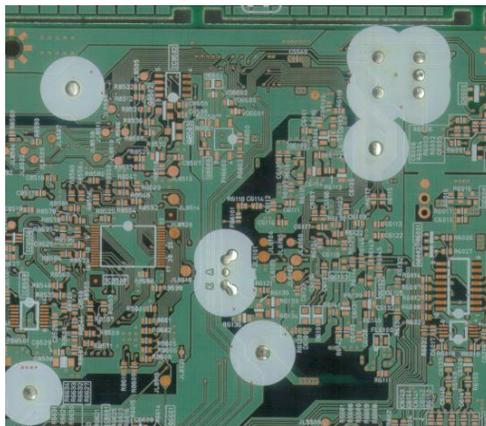
**Figure 1 – Selectively soldered PCB with white areas where solder joints are located.**
