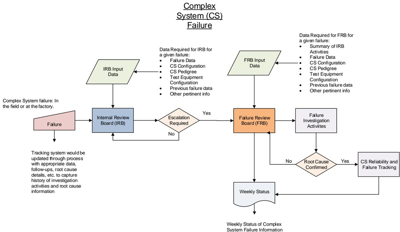
**Figure 1 - Complex System (CS) Failure Flow**
