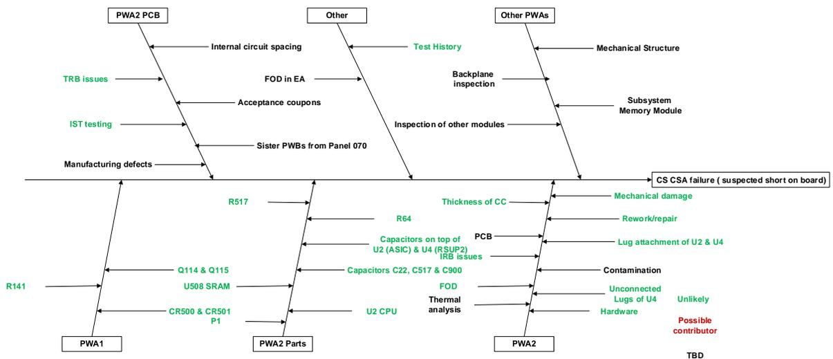
**Figure 7 - Fishbone Diagram for Computing Subassembly (CSA) Failure**
