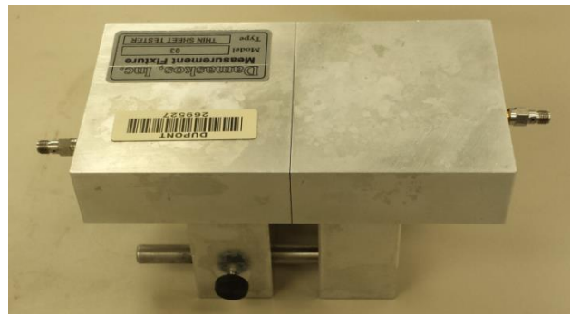
Figure 7 – Rectangular Cavity Resonator
