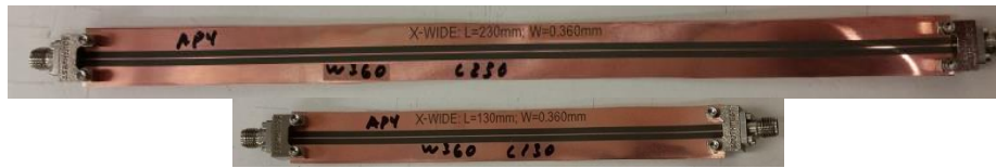
Figure 1 – Two Example Microstrip Transmission Lines for Impedance Extraction
