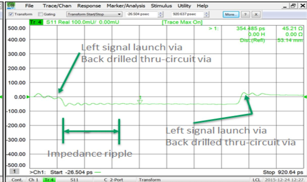
Circuit with back-drilled via for signal launch
