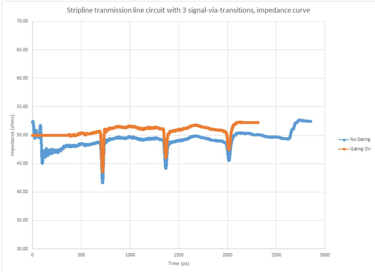
**Figure 7. Impedance curves for a stripline transmission line circuit with 3 signal-via-transitions and comparing the results with gating turn on and off.**
