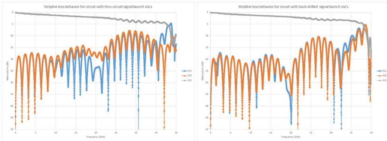
**Figure 6. Loss behavior for stripline transmission line circuits with different signal launch via configurations.**
