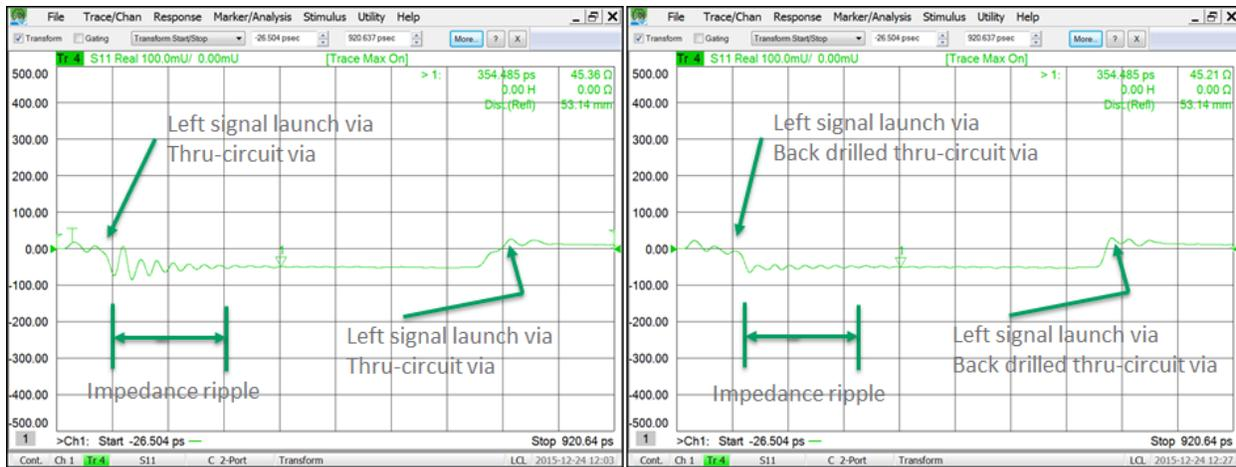
**Figure 5. Impedance curves (green curves) for a 2 inch stripline transmission line circuits with two different signal launch via constructions.**
