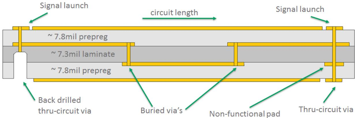
**Figure 1. Cross-sectional view of the test vehicle for this study with via definitions.**
