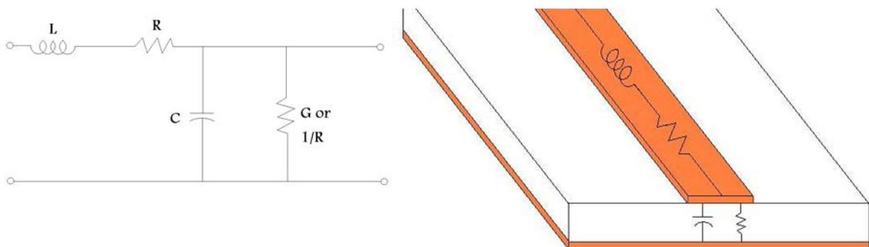
**Figure 2. Lumped element representation of a microstrip transmission line circuit.**
