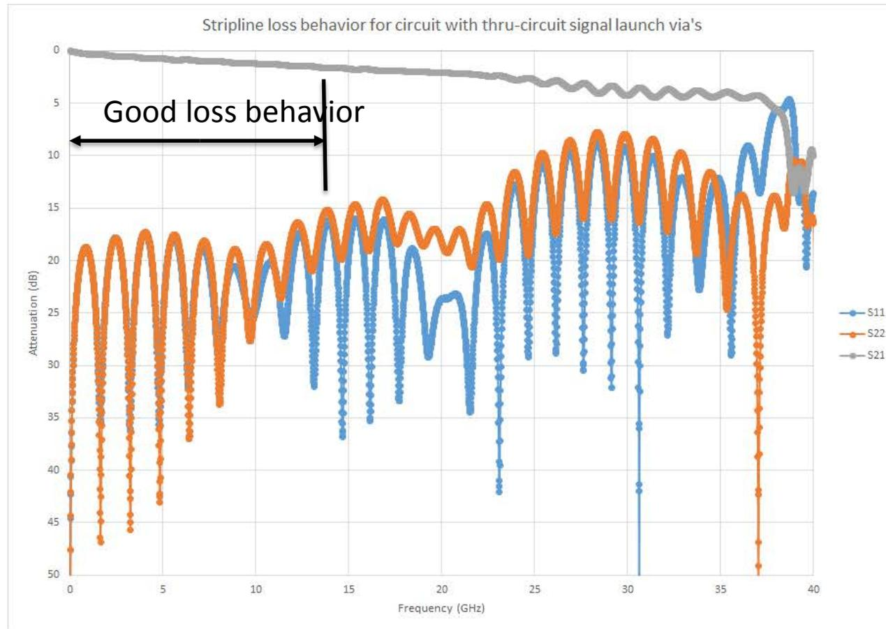
Circuit with thru-circuit via for signal launch
