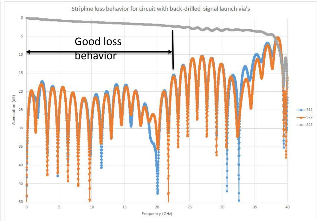
Circuit with back-drilled via for signal launch
