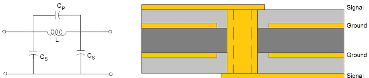
**Figure 4. An illustration of a PTH via per Wang, et al. [1]**
