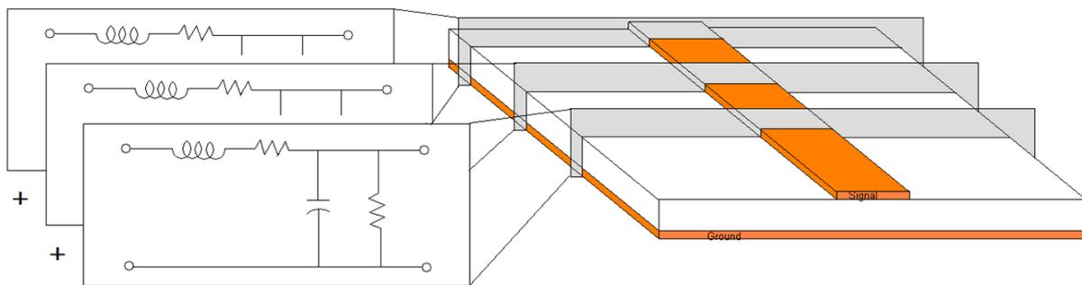
**Figure 3. Distributed representation of a microstrip transmission line circuit, as should be used for high frequency RF and high speed digital applications.**
