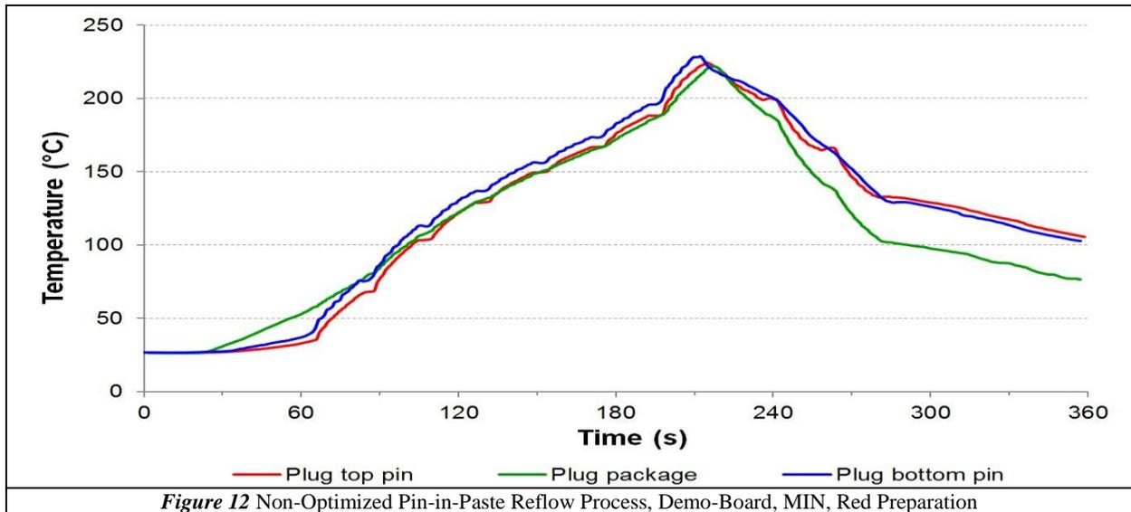
A time above liquidus of only  $t_L = 16$  seconds is achieved at the pin to be soldered at a maximum temperature of 229° C. Accordingly, the micrographs of the pins show soldered pins next to unsoldered pins (see **figures 13a, b, c**).
