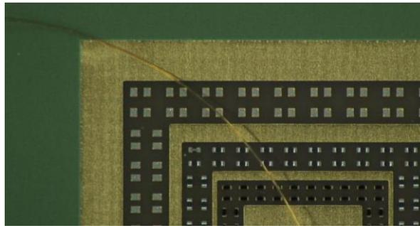
**Figure 0:** 0201 down to 03015(metric) compared to a human hair showing an example of miniaturization of components
