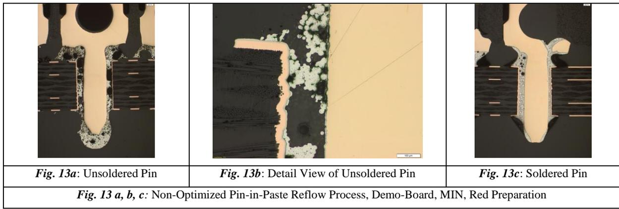
The detail view of the micrograph in *figure 13b* makes it apparent that only a few grains of the solder paste have melted, and that dwell time is too short for the production of a homogenous, molten solder phase.
