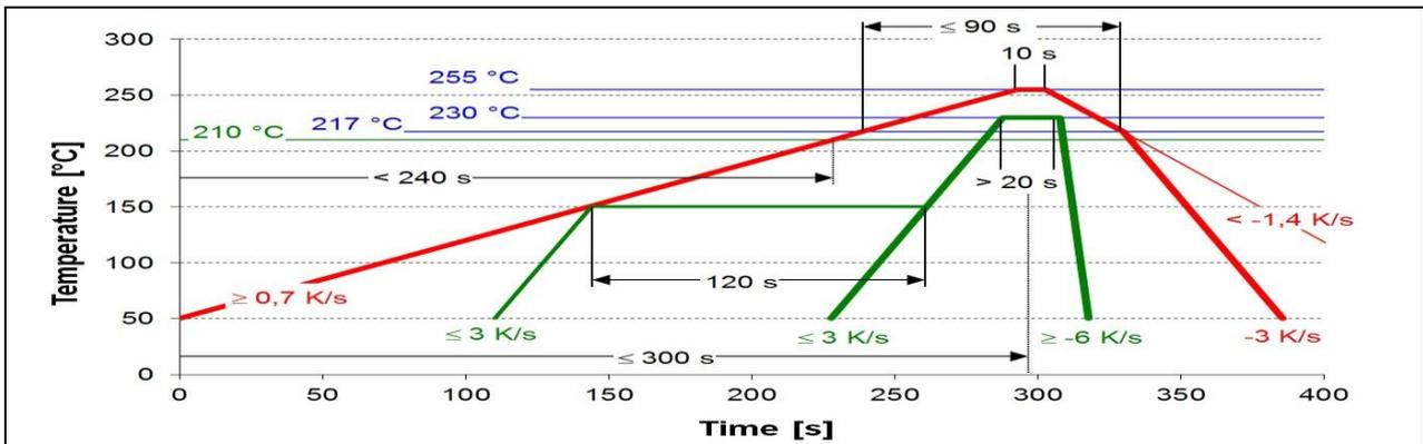
Figure 1: Target Reflow Profile for the company demonstrator board (reflow envelope profile [1])
