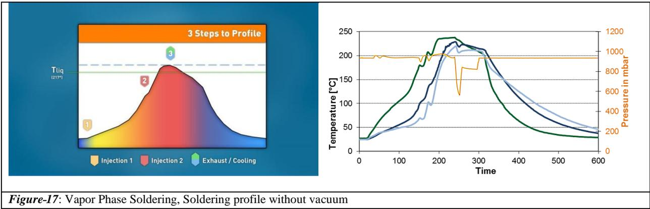
Figure-17: Vapor Phase Soldering, Soldering profile without vacuum
