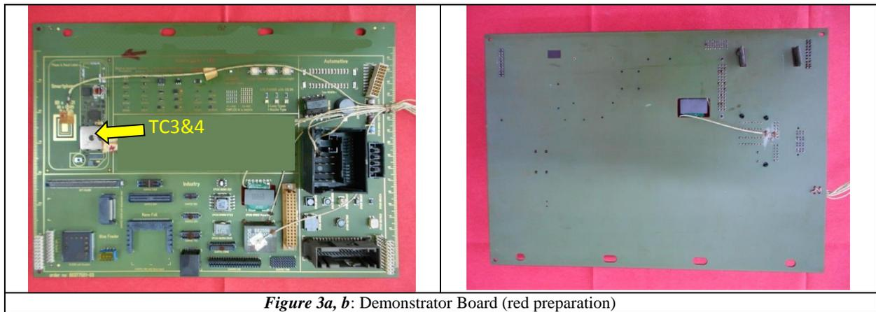
Figure 3a, b: Demonstrator Board (red preparation)
