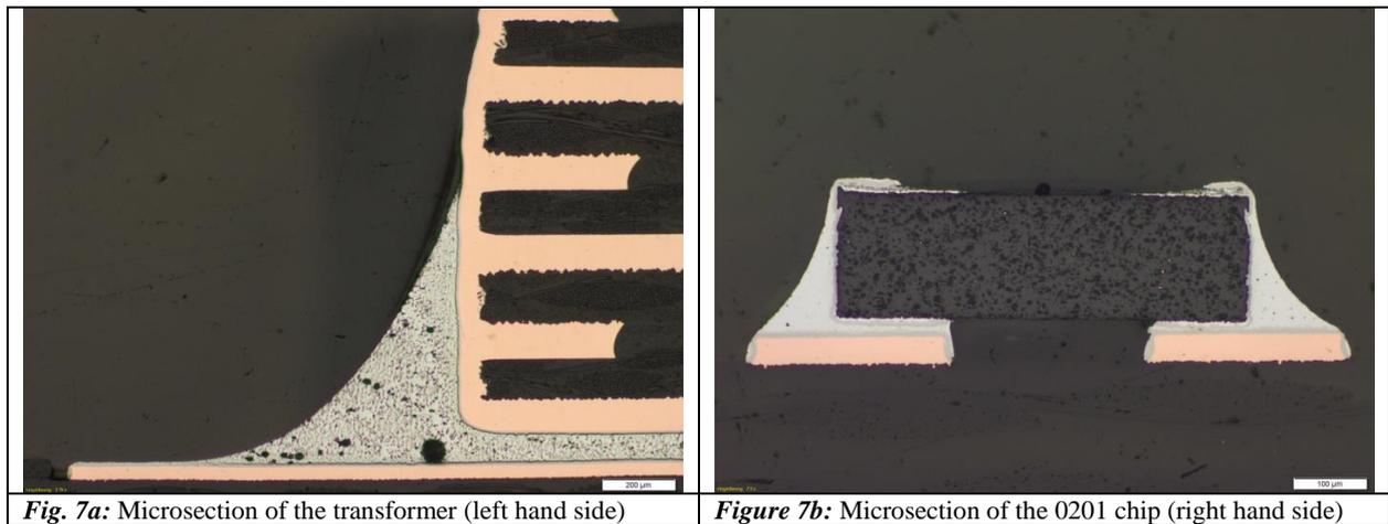
**Figure 7a:** Microsection of the transformer (left hand side)
