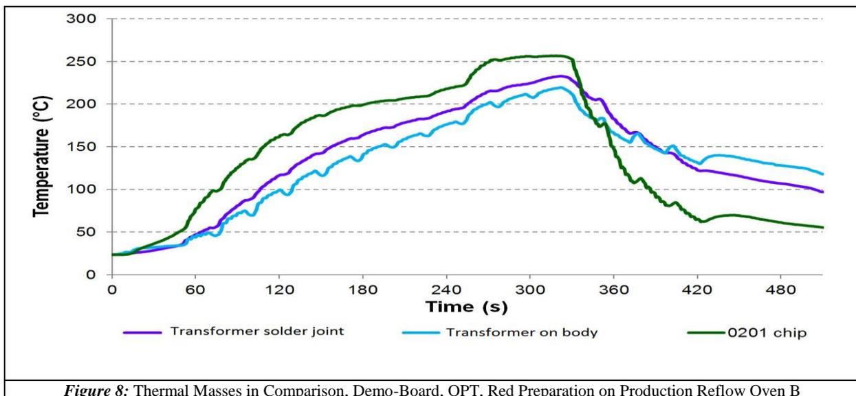
**Figure 8:** Thermal Masses in Comparison, Demo-Board, OPT, Red Preparation on Production Reflow Oven B
