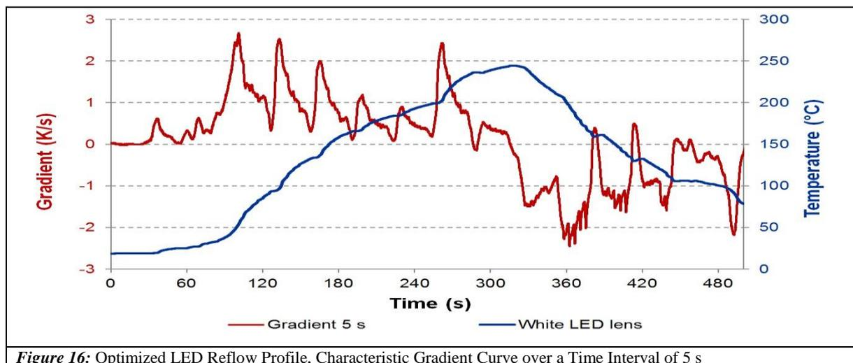
Figure 16: Optimized LED Reflow Profile, Characteristic Gradient Curve over a Time Interval of 5 s
