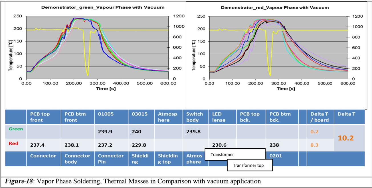
Figure-18: Vapor Phase Soldering, Thermal Masses in Comparison with vacuum application
