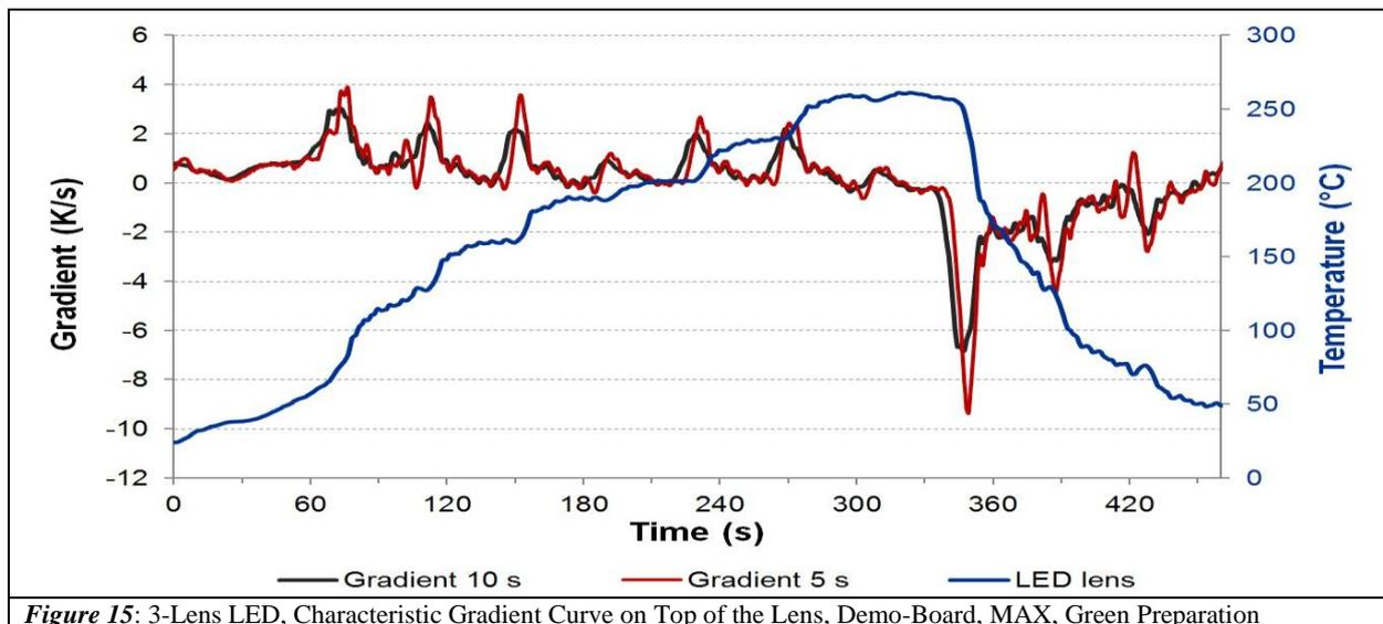
Figure 15: 3-Lens LED, Characteristic Gradient Curve on Top of the Lens, Demo-Board, MAX, Green Preparation
