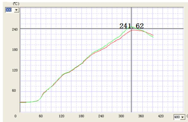
**Figure 15** Reflow profile used for QFN voiding test[1].
