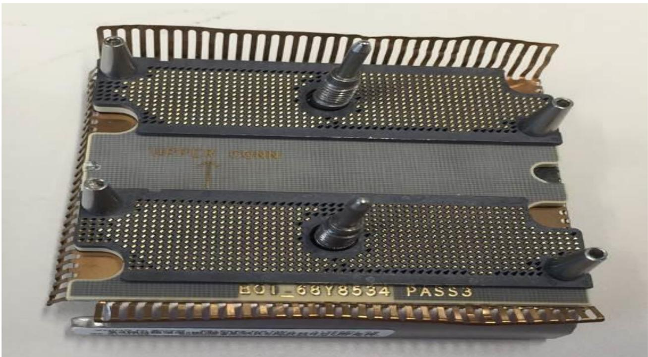
**Figure 27 – 2 Blade Server System Scalability Card**
