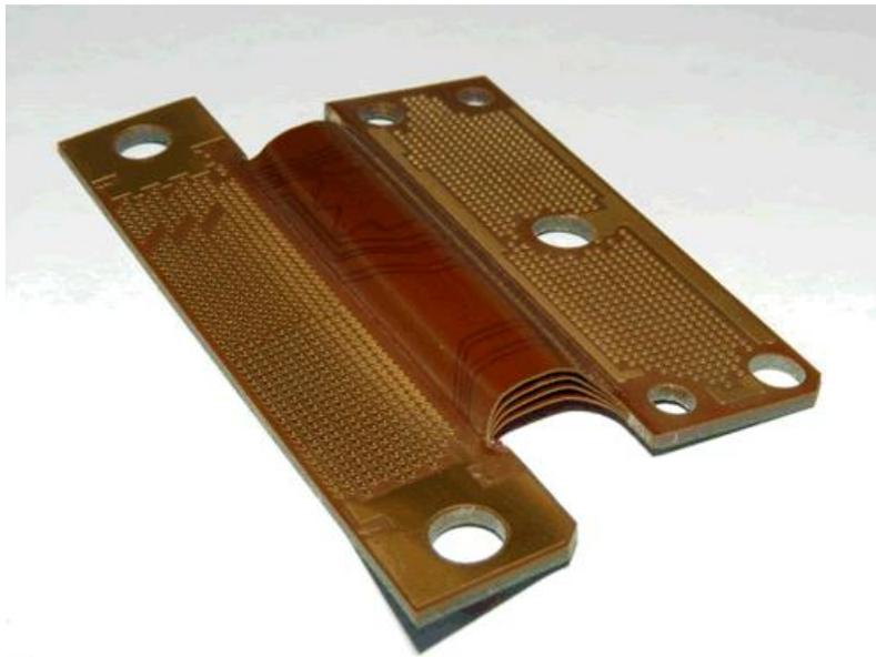
**Figure 22 – Rigid Flex with LGA Contacts Shown**
