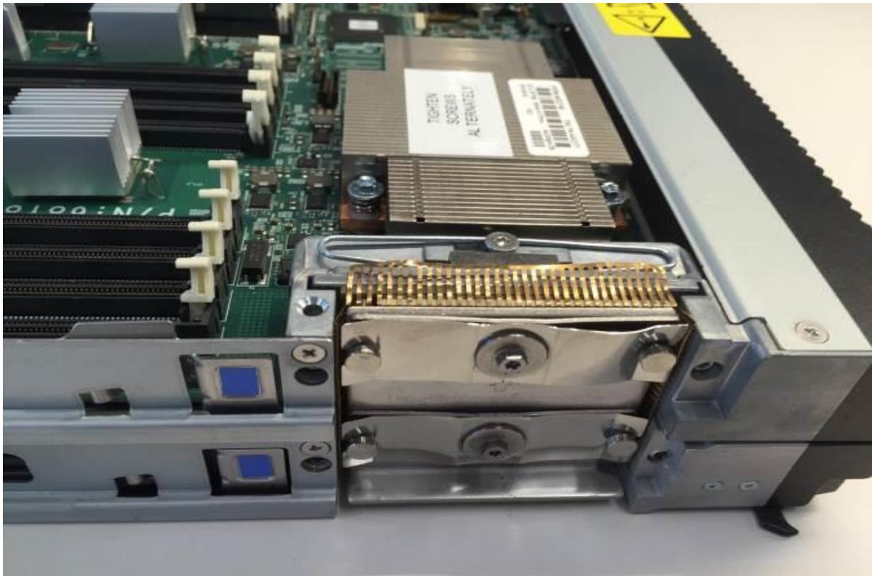
**Figure 29 – 2 Blade Server System with Scalability Card and Hardware Installed**
