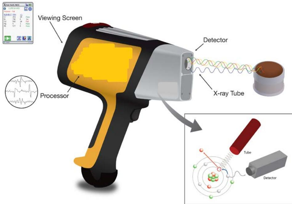
**Figure 1: Graphic Showing XRF Analyzer and Atom from the Sample.**
