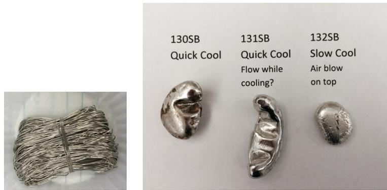
**Figure 8: Solder Buttons from Melted Bundles of Solder Wire (bundle example on left).**
