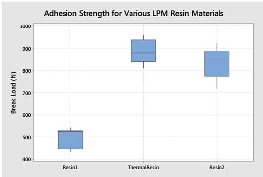
**Figure 7:** Chart comparing adhesion strengths of various LPM resins.
