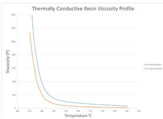
**Figure 6:** Viscosity comparison between standard LPM resin and thermally conductive resin.
