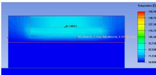
**Figure 4:** Thermal model of  $.6 \text{ W(mK)}^{-1}$  immediately after power cycle
