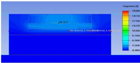
**Figure 5:** Thermal model of  $1.5 \text{ W(mK)}^{-1}$  immediately after power cycle
