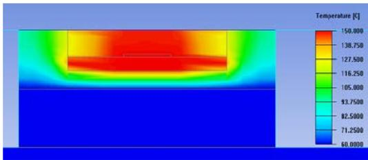
**Figure 3:** Thermal model of  $0.2 \text{ W(mK)}^{-1}$  immediately after power cycle.
