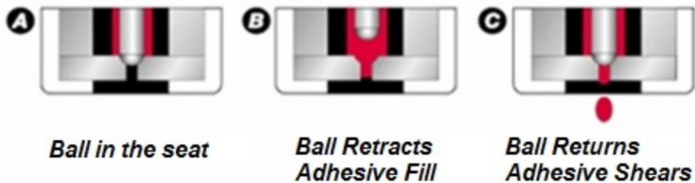
JET APPLICATOR CUTAWAY VIEW
