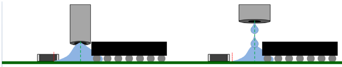
Figure 1 – KOZ: Needle Dispensing vs. Jet Dispensing
