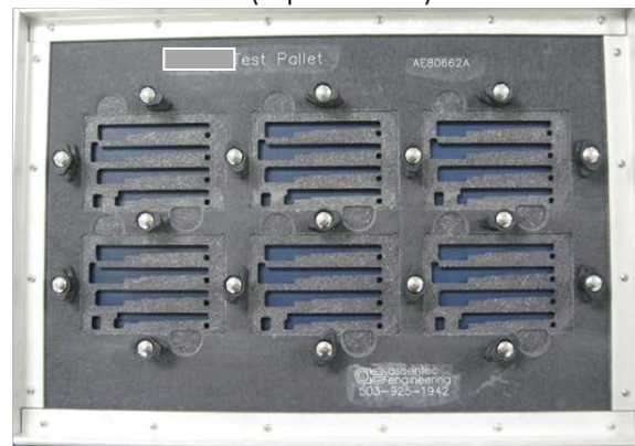
Selective wave solder fixture (Top side view)
