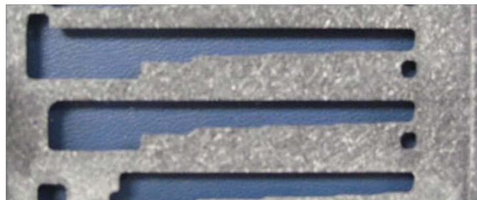
Figure 16 – Open and Selective Wave Soldering Pallet Designs
