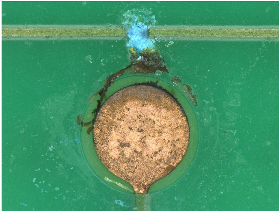
Figure 3: Electrochemical Migration from a Power Trace not covered with Solder mask and the Ground Pad
