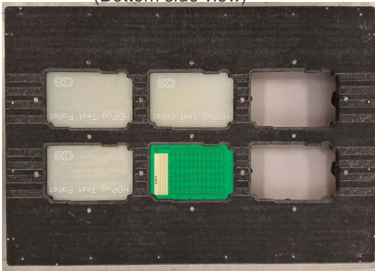
Full open wave solder fixture (Bottom side view)
