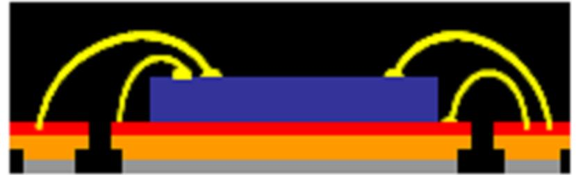
(b) Saw Singulated, Lead Pullback
