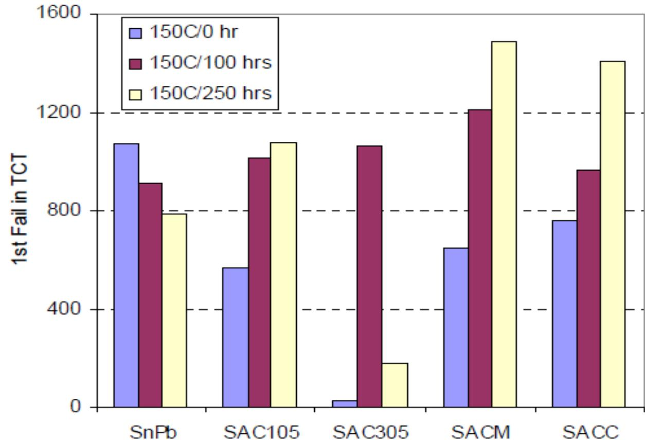
**Fig. 14** First failure of TCT for TFBGA (NiAu) on PCB (OSP).
