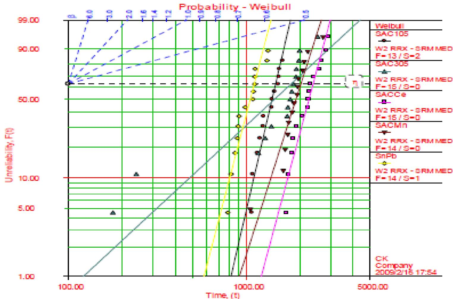
**Fig. 12 Weibull plot for TCT performance for TFBGA (NiAu) with various sphere alloys assembled on PCB (OSP). Prior to TCT, the device was aged at 150C for 250 hrs.**
