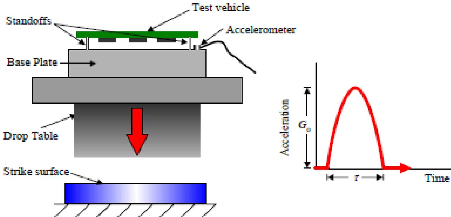
Fig. 1 Schematic for JEDEC board-level drop test.
