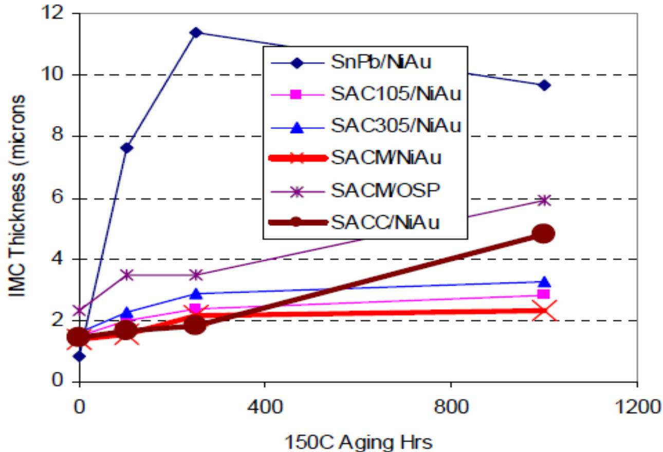
**Fig. 28** IMC thickness of TFBGA joints at packaging side mounted on PCB (OSP).
