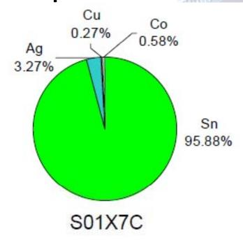
Low Silver alloy (Koki S01X7C- Sn0.1Ag0.7Cu0.03Co) reduces cost compared with Sn3Ag0.5Cu
