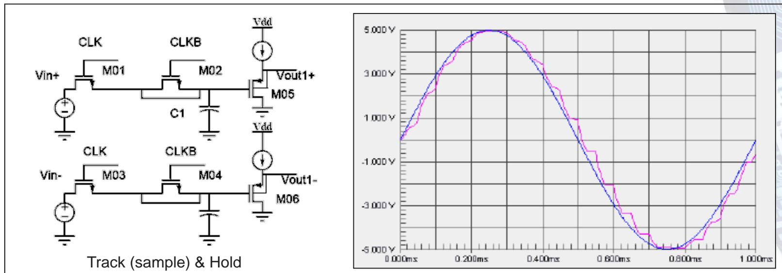
Transistor stress state analysis on Track and Hold functional group
