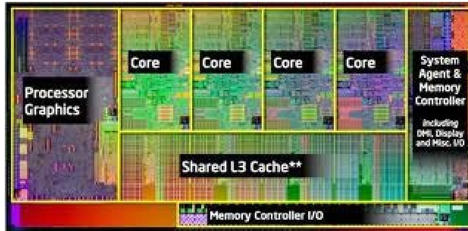
Graphic and overlay of Intel Core i5 Processor
