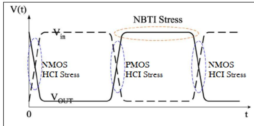
Transistor stress states relating to HCI/NBTI damage ( $V_{in}/V_{out}$  curve)
