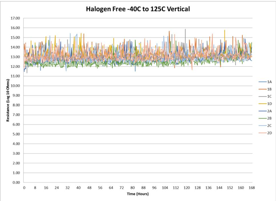
Figure 22 – Halogen-Free -40°C to 125°C Vertical SIR Results
