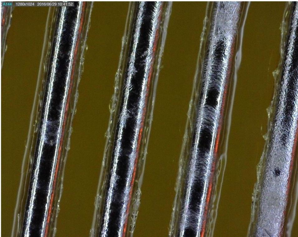
**Figure 10 - Halogen-Containing -  $-40^{\circ}\text{C}$  to  $+125^{\circ}\text{C}$  Thermal Cycling – Horizontal Orientation**
