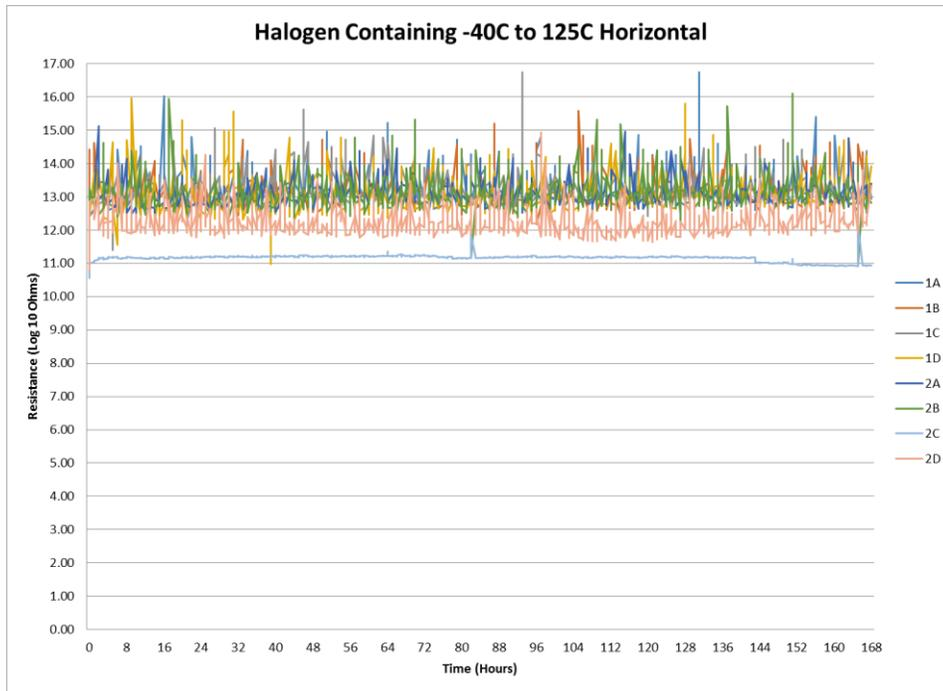
Figure 26 – Halogen-Containing -40°C to 125°C Horizontal SIR Results
