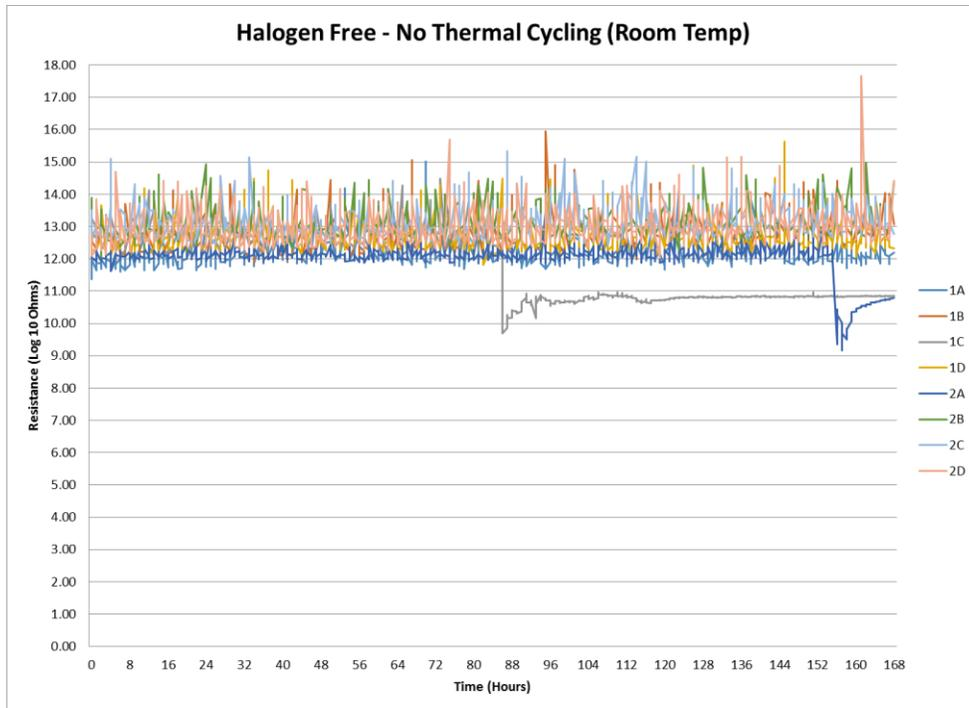
Figure 20 – Halogen-Free – No Thermal Cycling (Room Temperature) SIR Results
