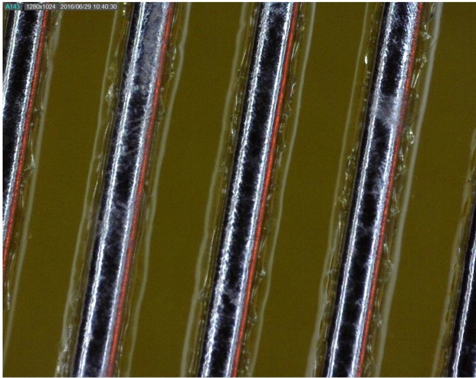
**Figure 11 - Halogen-Containing - -40°C to +125°C Thermal Cycling – Vertical Orientation**
