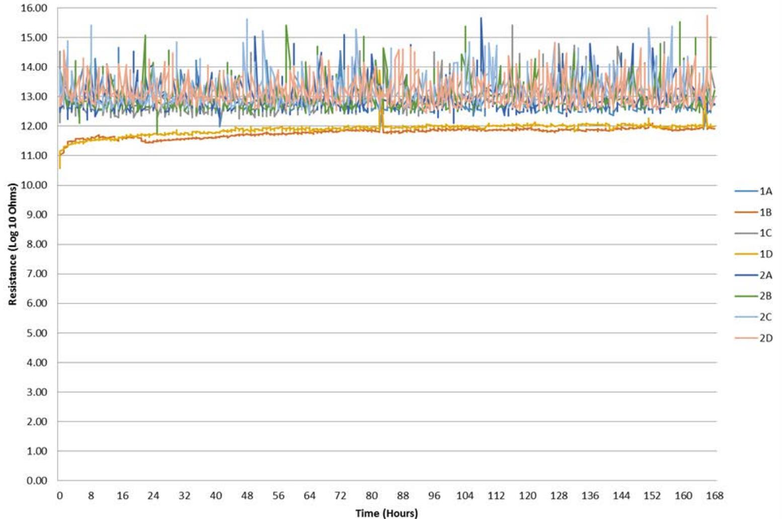
**Halogen Containing - No Thermal Cycling (Room Temp)**
