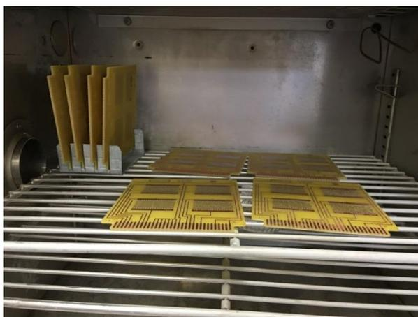
**Figure 2 - Orientation of the Boards in the -40°C to +125°C Chamber**
