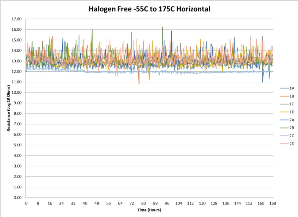
Figure 23 – Halogen-Free -55°C to 175°C Horizontal SIR Results
