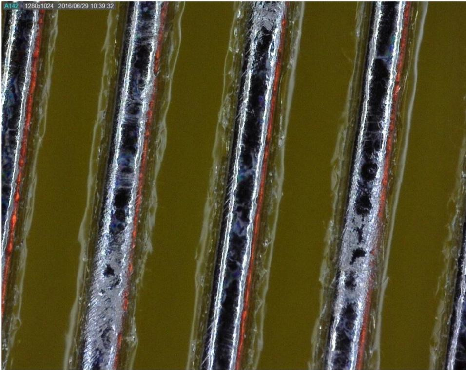
**Figure 9 - Halogen-Free -  $-40^{\circ}\text{C}$  to  $+125^{\circ}\text{C}$  Thermal Cycling – Vertical Orientation**
