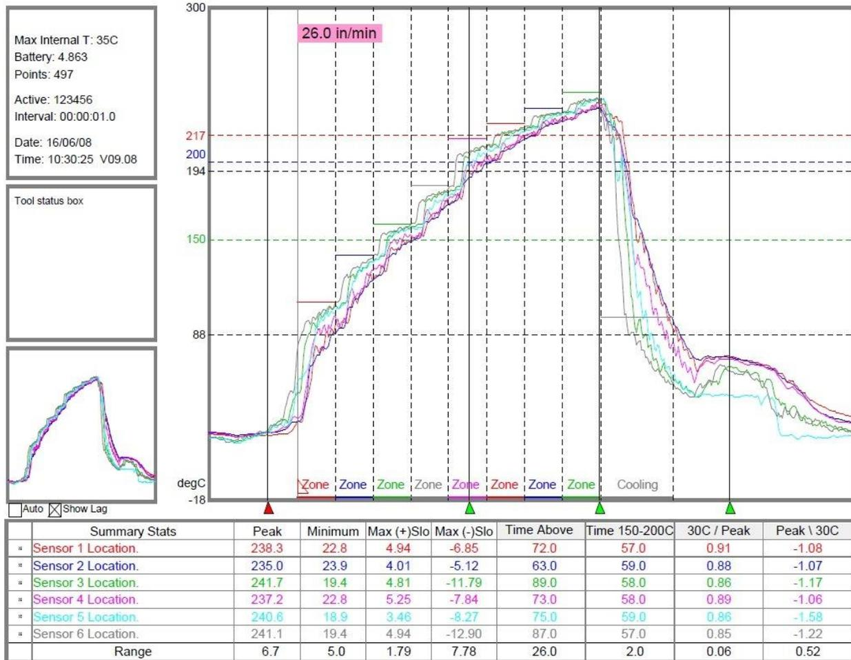
Figure 1 – Air Reflow Profile
