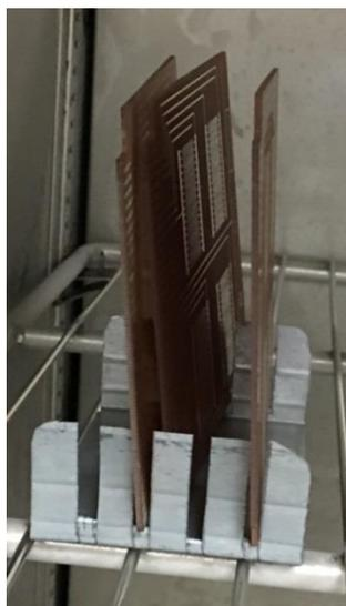
**Figure 4 – Disturbed Vertically-Orientated Boards in the -55°C to +175°C Chamber**
