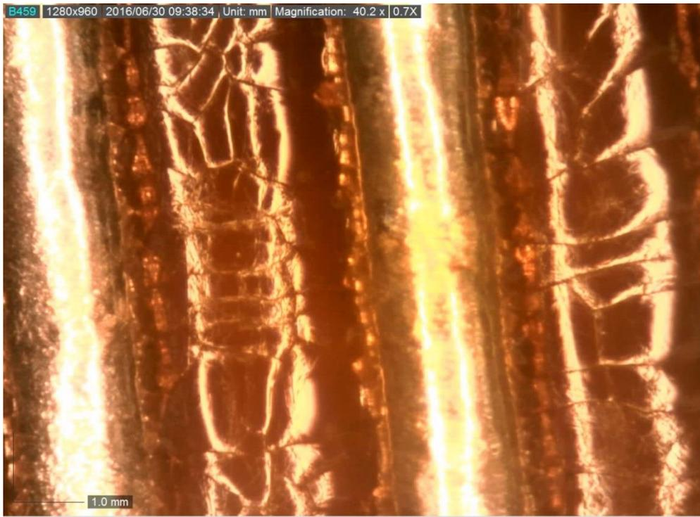
**Figure 16 - Flux Cracking - -55°C to 175°C Thermal Cycling**
