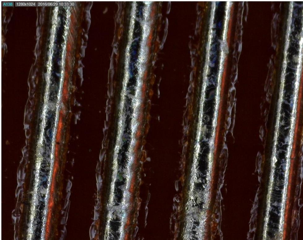
**Figure 12 - Halogen-Free - -55°C to +175°C Thermal Cycling – Horizontal Orientation**
