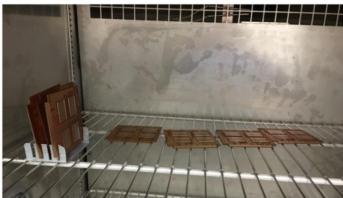
**Figure 3 - Orientation of the Boards in the -55°C to +175°C Chamber**
