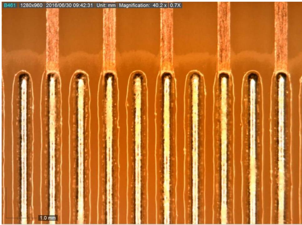
**Figure 17 - Flux Migration -  $-40^{\circ}\text{C}$  to  $+125^{\circ}\text{C}$**
