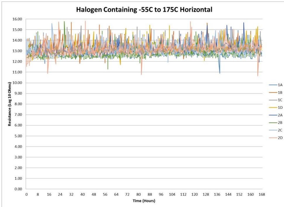
**Figure 28 – Halogen-Containing -55°C to 175°C Horizontal SIR Results**
