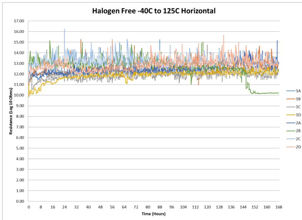
Figure 21 – Halogen Free -40°C to 125°C Horizontal SIR Results
