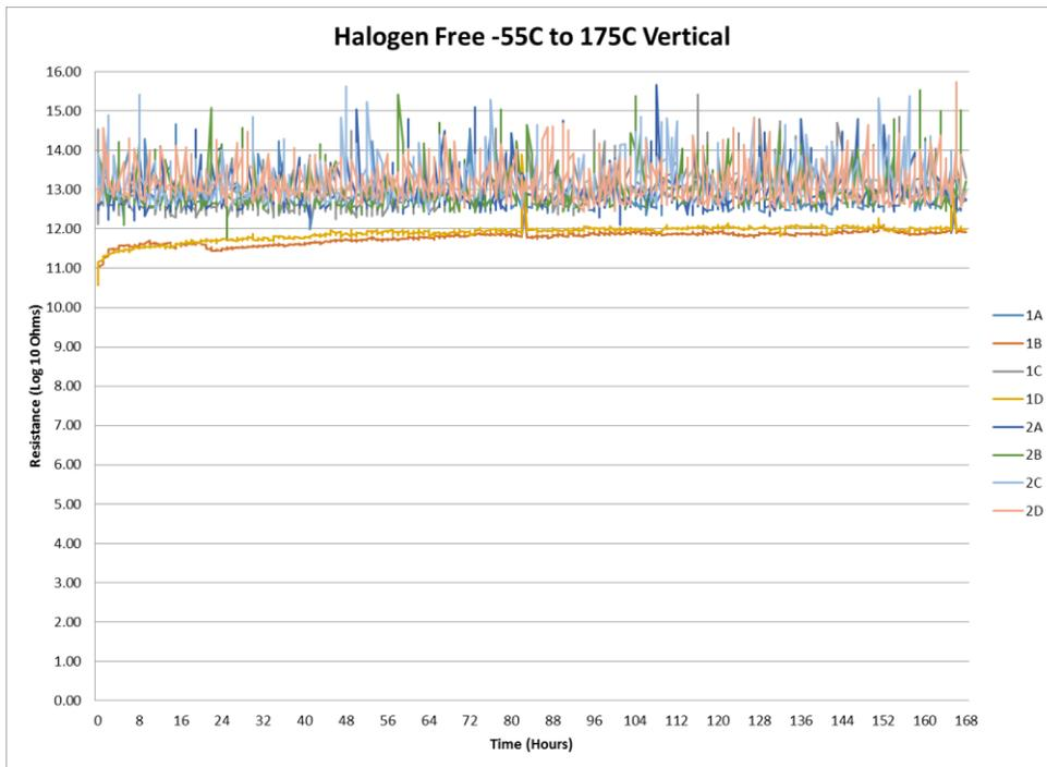
Figure 24 – Halogen-Free -55°C to 175°C Vertical SIR Results
