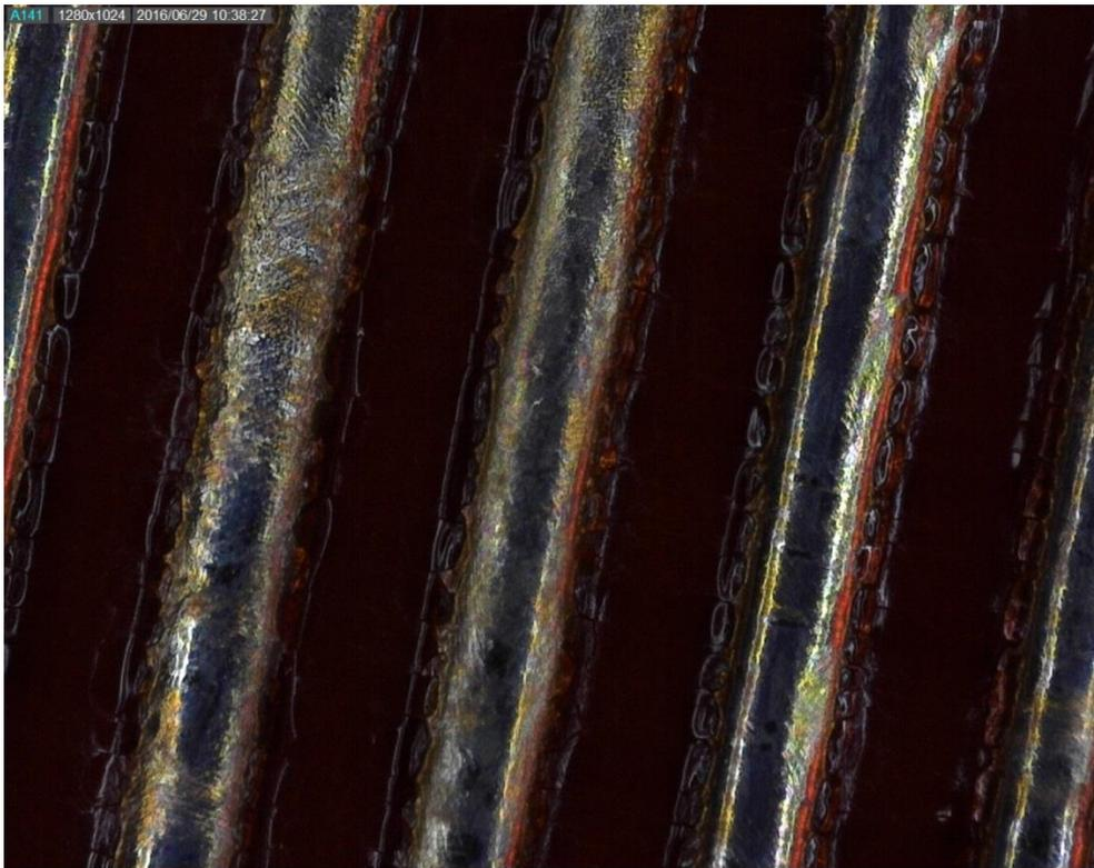
**Figure 15 - Halogen-Containing - -55°C to +175°C Thermal Cycling – Vertical Orientation**
