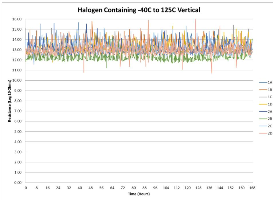
Figure 27 – Halogen-Containing -40°C to -125°C Vertical SIR Results
