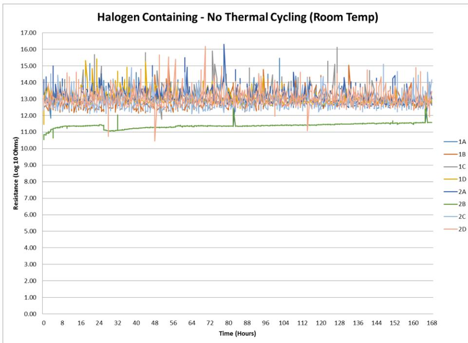
Figure 25 – Halogen-Containing – No Thermal Cycling (Room Temperature) SIR Results
