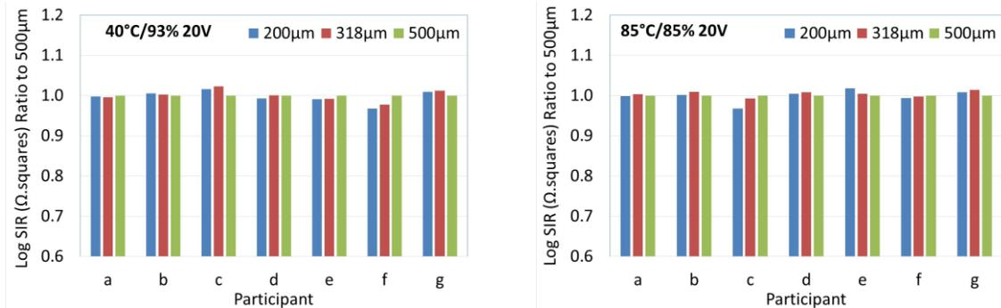
**Figure 27: Ratio of the log Ω-square value to the 500μm pattern**
