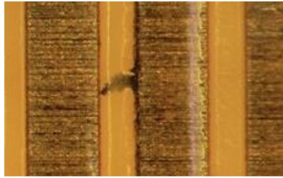
**Figure 19: Participant E and evidence of corrosion shorting across the gap**
