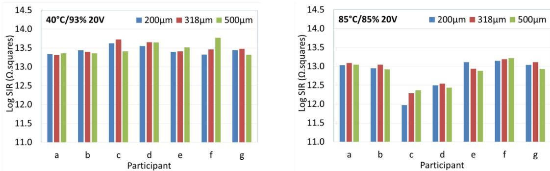
**Figure 26: Final SIR plotted as Ohm.Squares**
