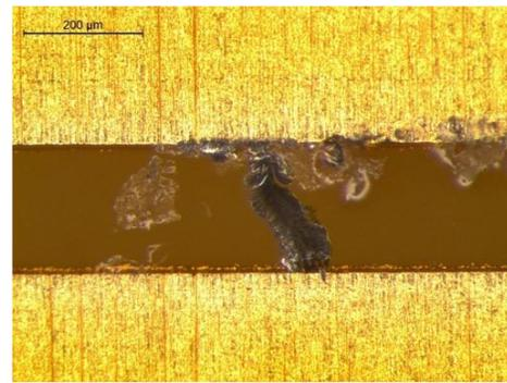
**Figure 21: Participant G and a corrosion defect probably from flux residue**
