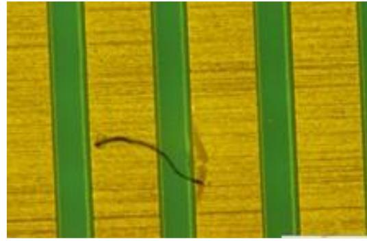
**Figure 18: Participant D, and evidence of a fibre and the effect on the SIR**
