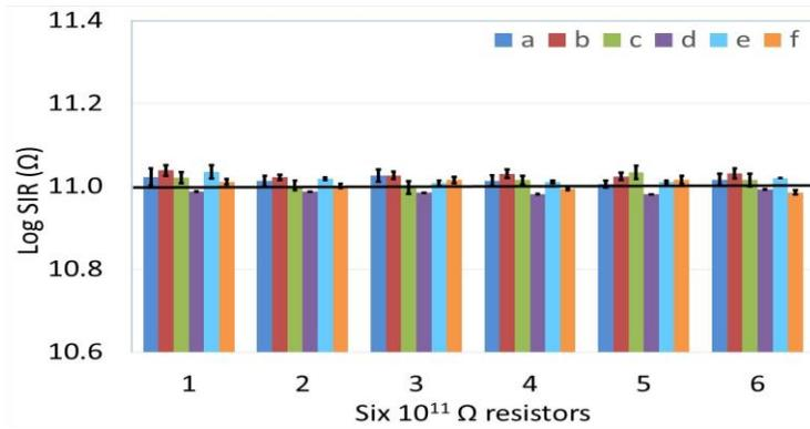
**Figure 3: Participants (a to f) resistance measurements for the six resistors on the checker board**
