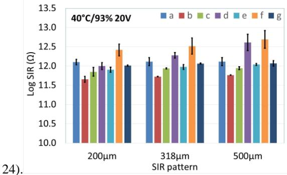
**Figure 23: The average final SIR value for the control boards**
