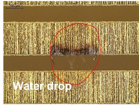
**Figure 20: Participant G and evidence of a water droplet and the resulting drop in SIR and dendrite like failure**
