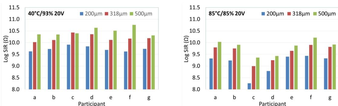
**Figure 25: The average final SIR for flux loaded patterns by participant**
