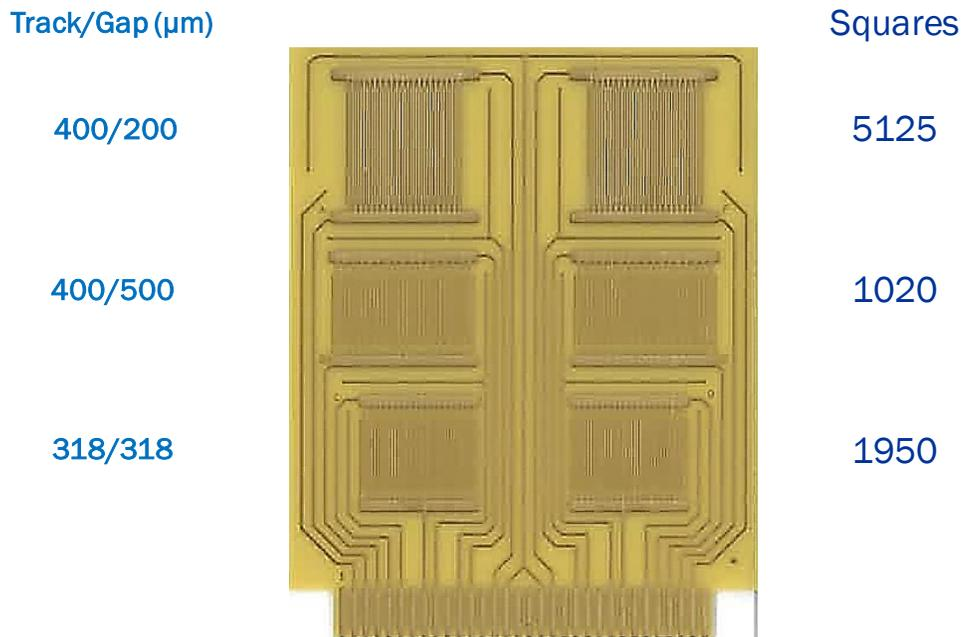
**Figure 1: The test PCB, TB144**
