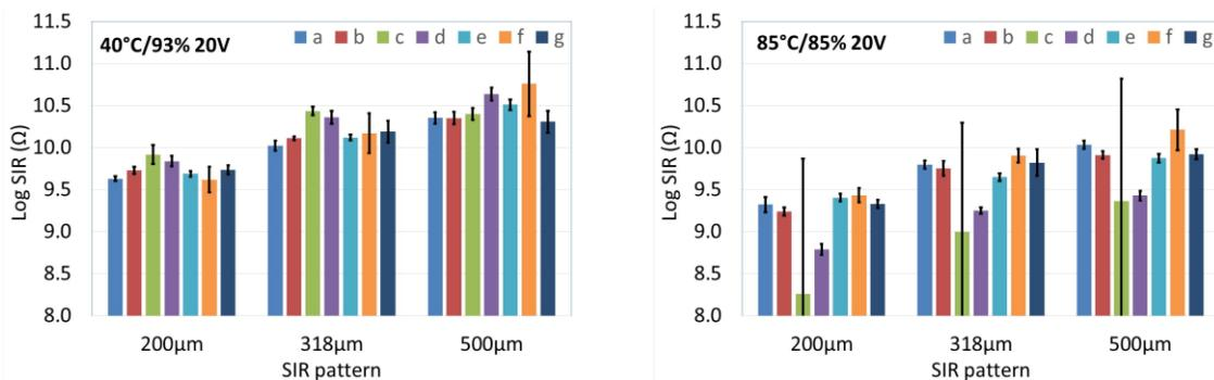
**Figure 24: The average final SIR value for the flux loaded boards**
