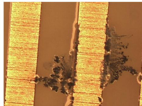
**Figure 22: Participant C dendrites and corrosion formed on all SIR patterns of all fluxed samples tested at 85°C/85%RH**
