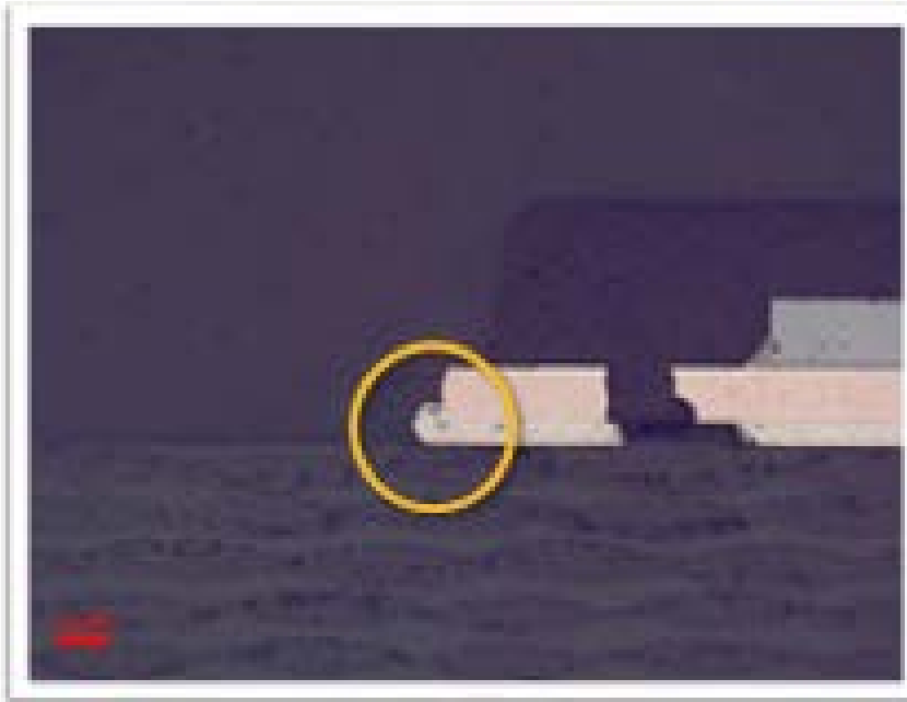
No Overprint Typical Solder Fillet
