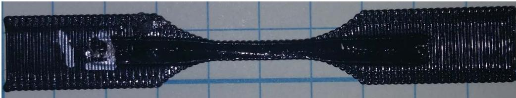
90° Tensile Specimen after Laser Reflow
