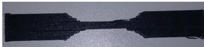
**Figure 4: 0° Printed Tensile Specimen Using 0.4mm Nozzle**
