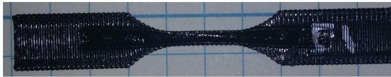
*Figure 11: Laser "Reflowed" Tensile Part*
