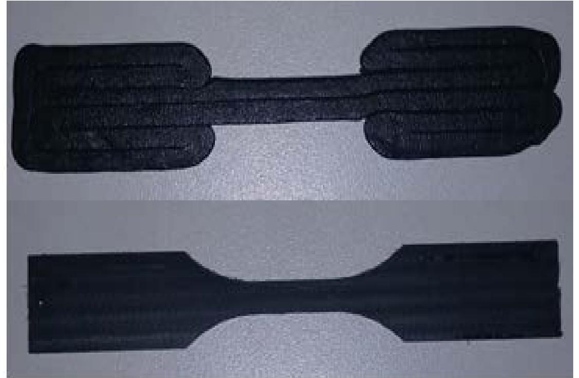
90° Printed and Milled Tensile Specimen
