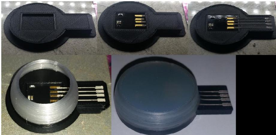
**Figure 6: Steps of a Printed USB Device**
