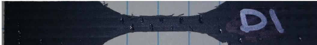
0° Printed and Milled Tensile Specimen
