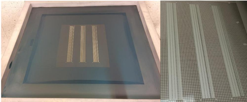
**Figure 6 Test vehicle screen (left) and printed (right)**
