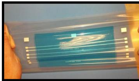
Figure 12. Silver and Insulator on TPU Film under Stretch
