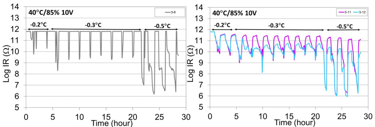
Figure 13: SIR measurements for condensing environments for paste C with QFP160 (left) and QFN40 (right)
