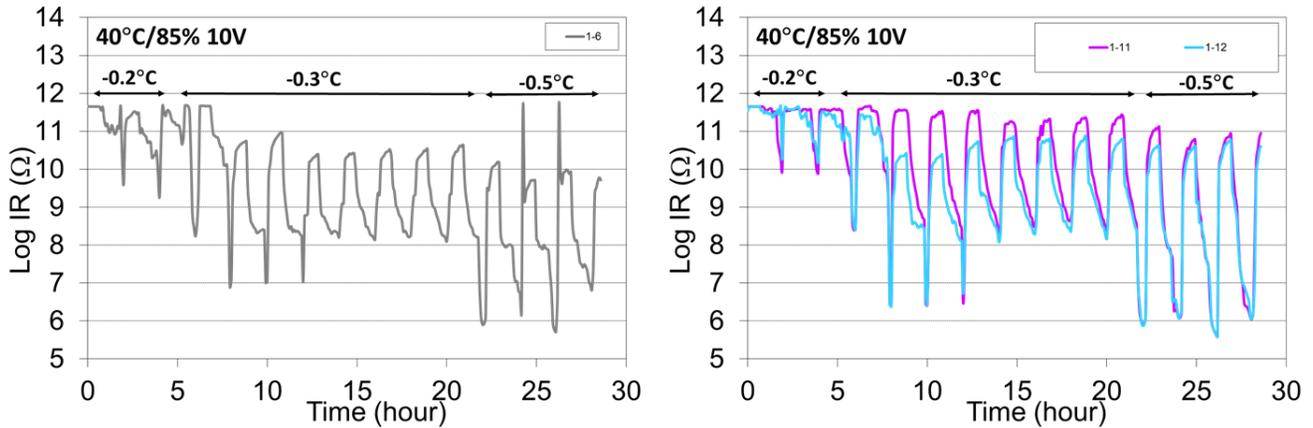
Figure 11: SIR measurements for condensing environments for paste A with QFP160 (left) and QFN40 (right)
