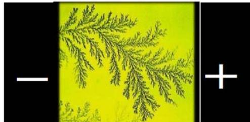
Dendrite short two conductors
