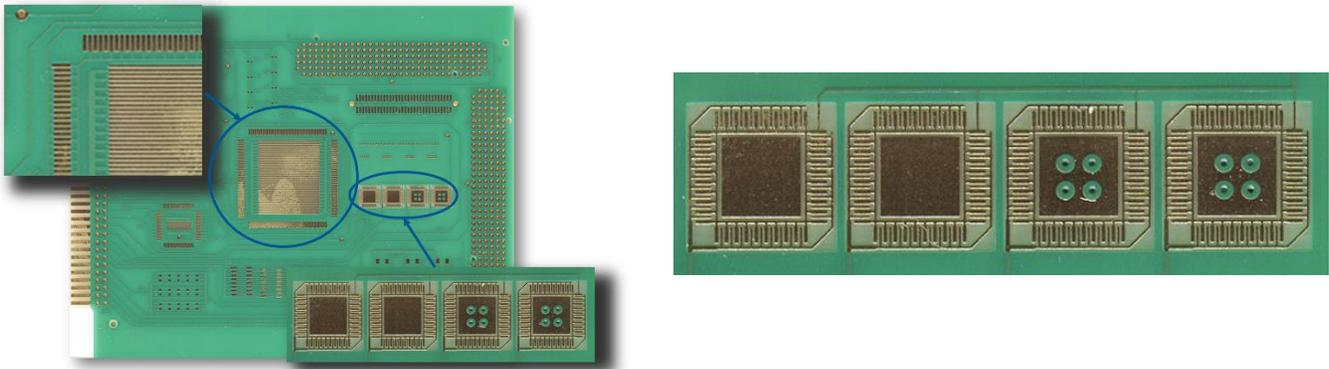
Figure 1: Modified B52 test vehicle (Left). Close-up of the SIR test pattern (right) added to the IPC-B52 board.
