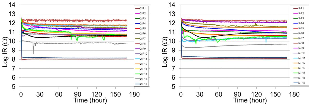
Figure 7: Example SIR measurements for paste A
