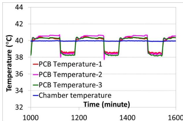
Figure 5: PCB temperature profile during platen thermal cycling
