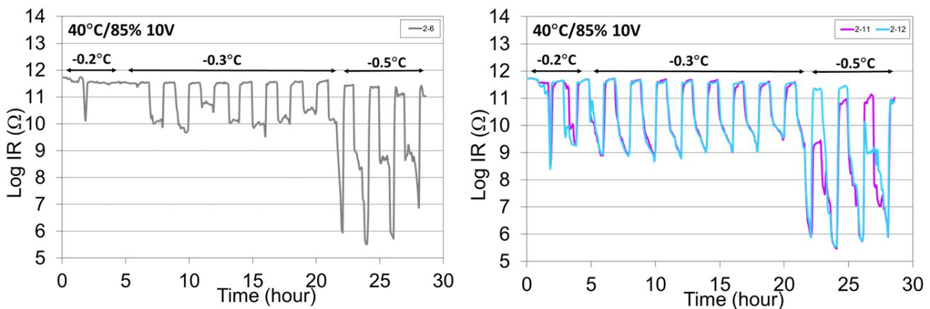
Figure 12: SIR measurements for condensing environments for paste B with QFP160 (left) and QFN40 (right)
