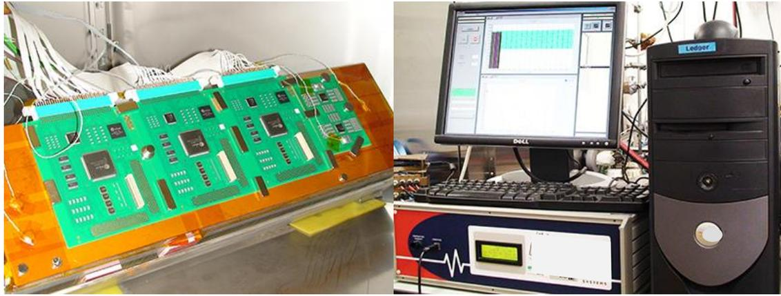
Figure 4: SIR test boards mounted on the specially designed test platen for condensation testing and the system for continuous monitoring of the test boards
