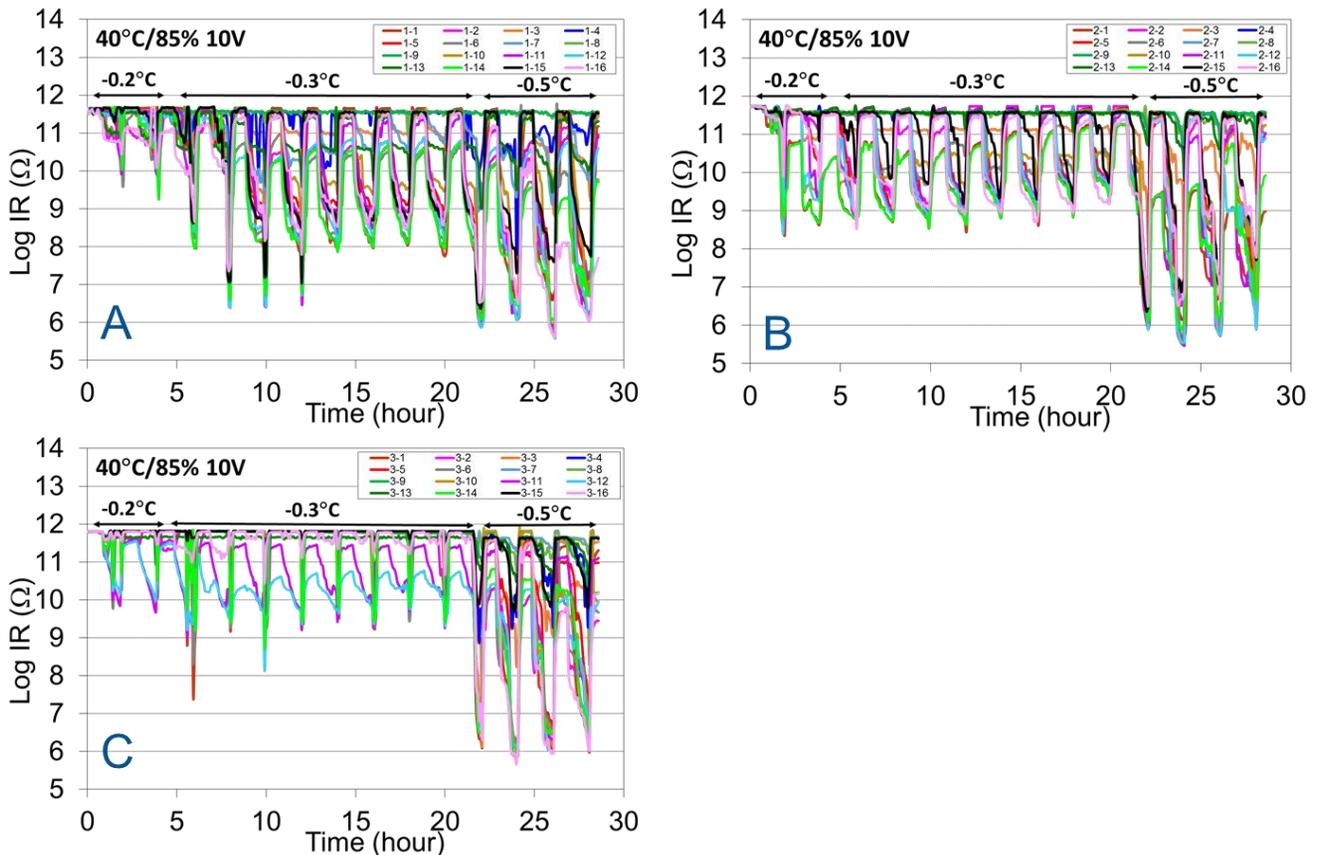
Figure 10: SIR measurements for condensing environments for each of the three pastes
