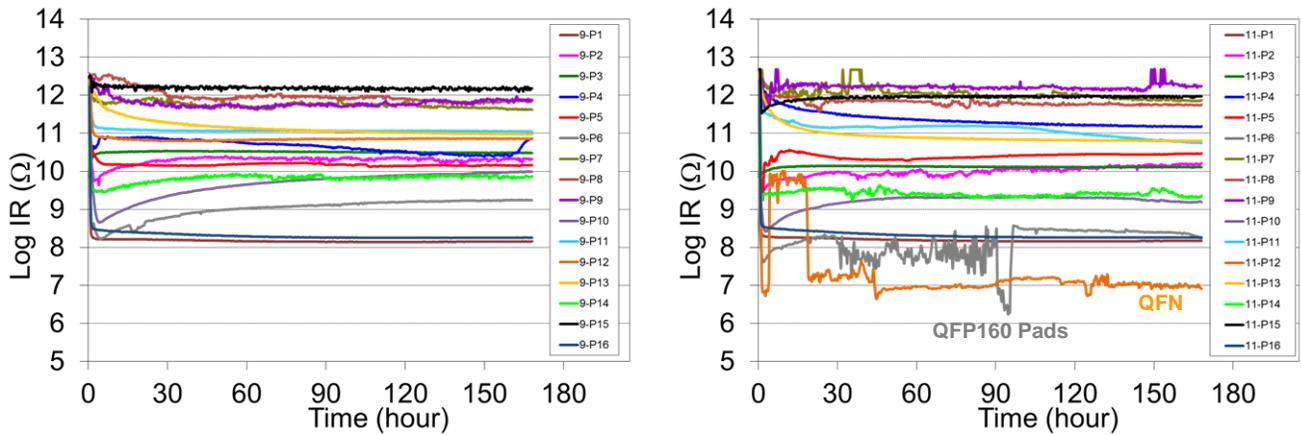
Figure 9: Example SIR measurements for paste C
