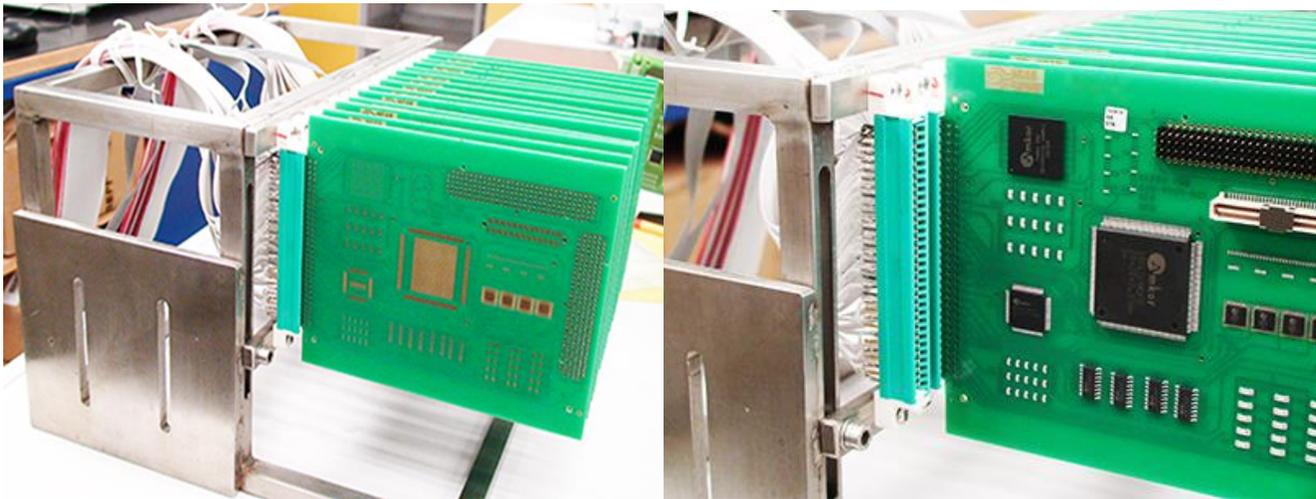
Figure 3: Sample boards mounted ready for conventional SIR testing in a temperature and humidity test chamber
