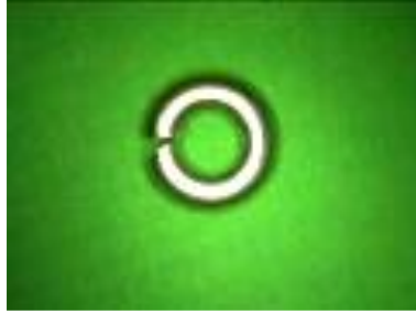
Figure 5: Solder ring for spreading test
