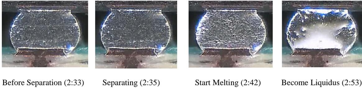
Figure 6 Solder Joint Images from Reflow Simulator
