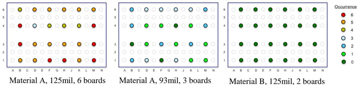
Figure 3 Frequency of Separated Solder Joint Location Analysis
