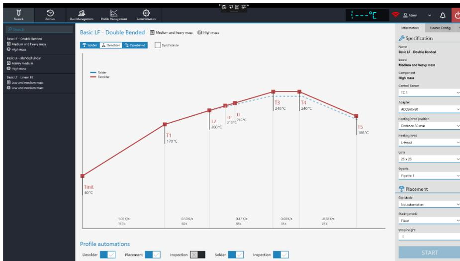
Figure 4 Clearly structured profile selection for a rework process
