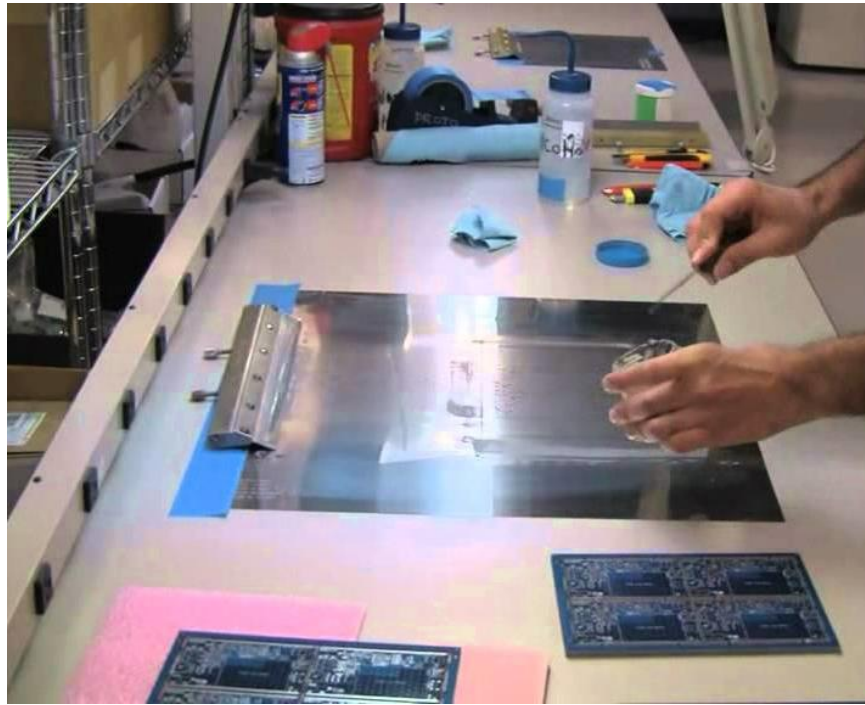
Figure 4 – Typical manual stencil printing set- up
