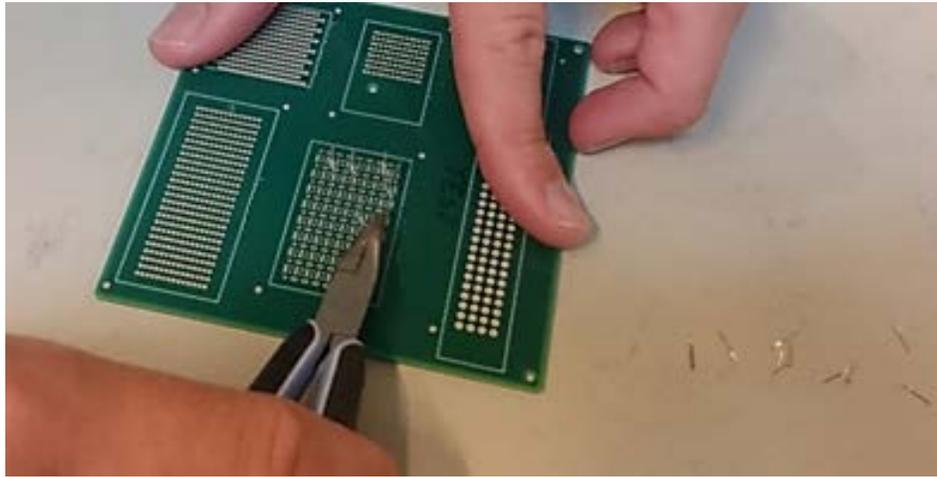
**Figure 34 –Removal of remaining pins on connector E.**
