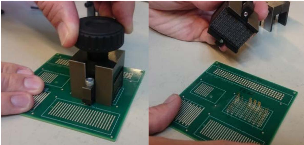
**Figure 33 –Removal of connector E.**
