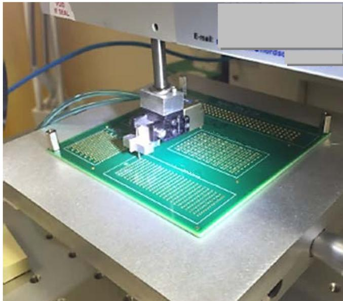
**Figure 40 –Equipment for insertion and retention test.**
