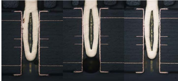
**Figure 56 – Vertical cross sectioning of connector A, ENIG plating – maximum specified hole diameter (left), nominal diameter (middle) and minimum diameter (right).**
