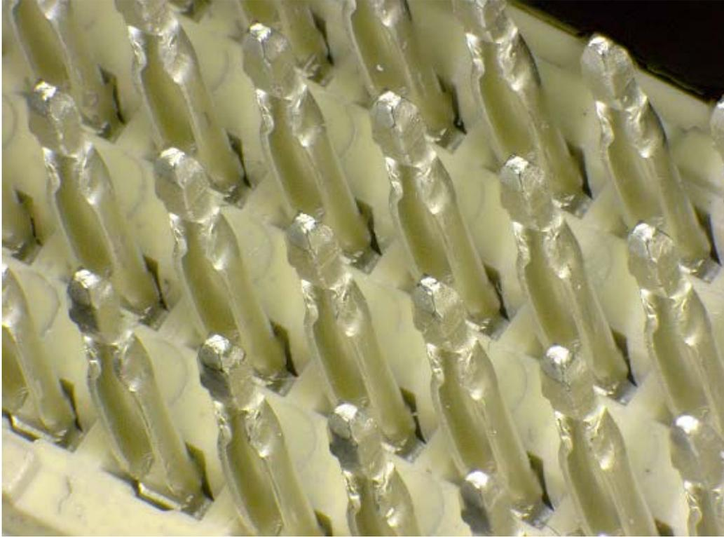
**Figure 9 – Press fit pins for reference connector D.**
