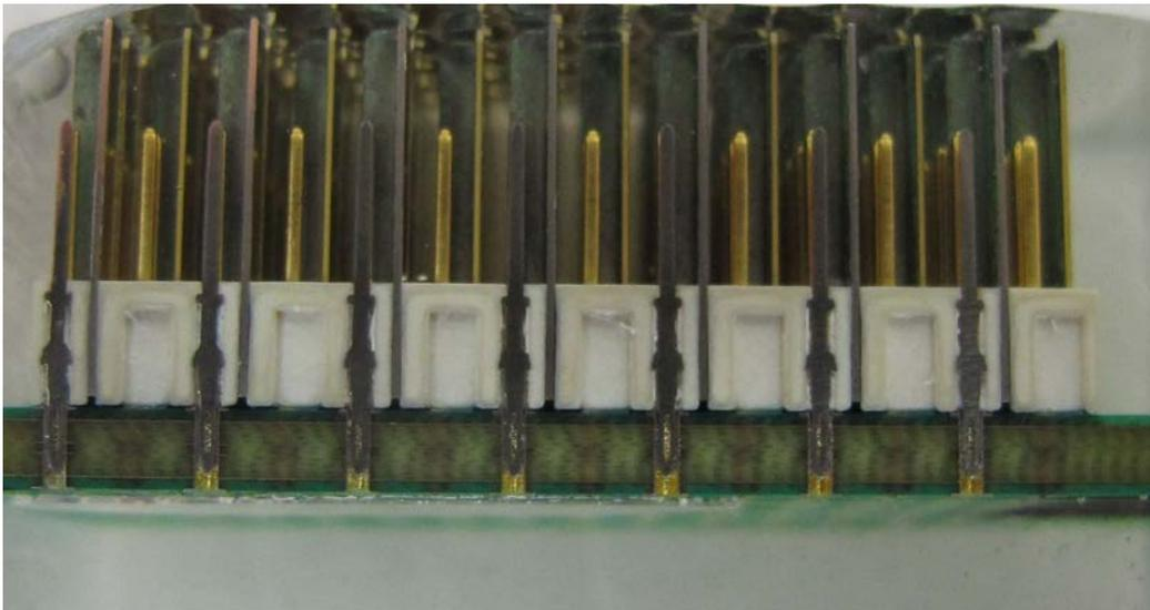
**Figure 55 – Vertical cross sectioning of connector A.**
