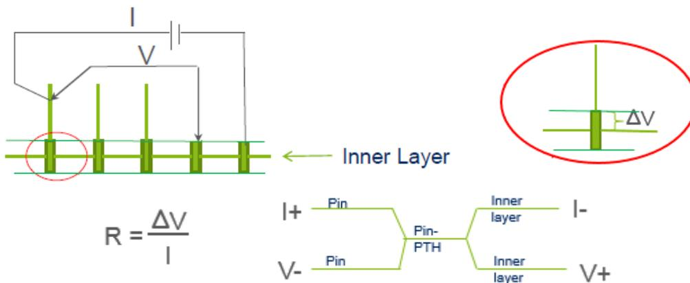
**Figure 50 – Contact resistance measured by using an inner layer (when no protruded pins are available)<sup>6</sup>.**
