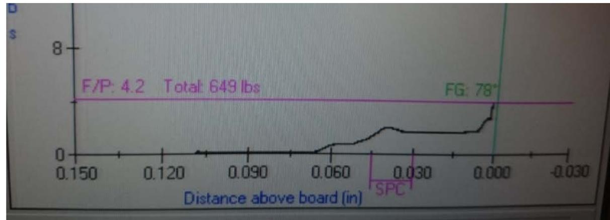
Force-time curve for connector C
