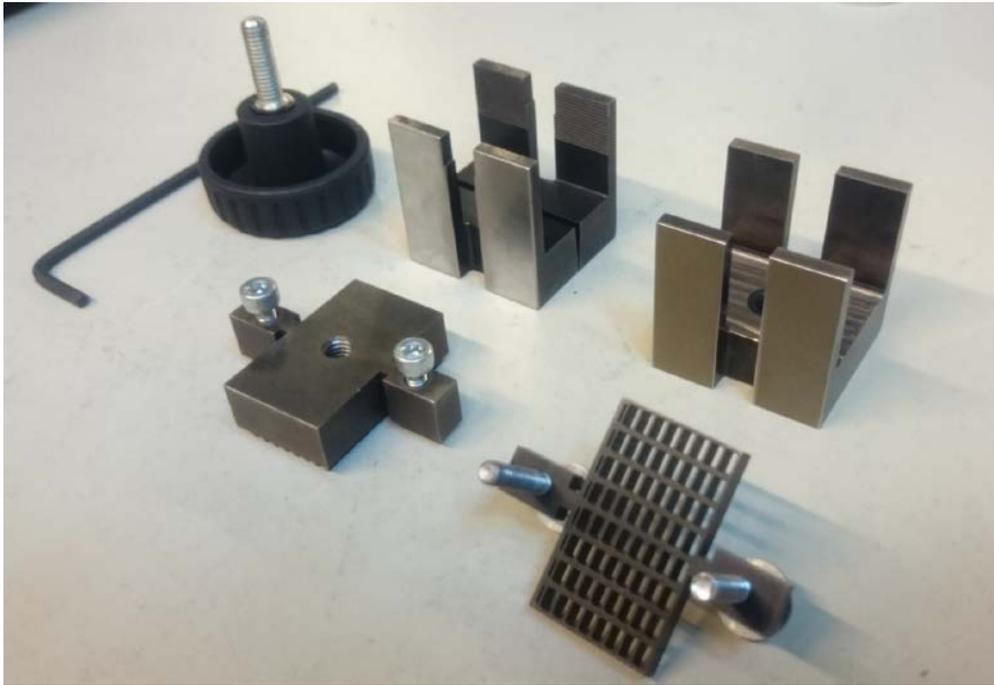
**Figure 32 –Tooling for removal of connector E.**
