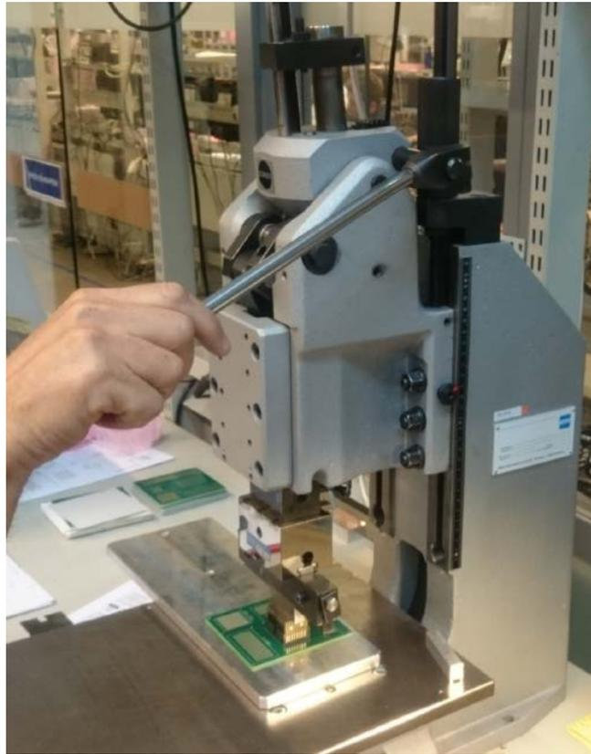
**Figure 26 –Manual press in of connector E.**
