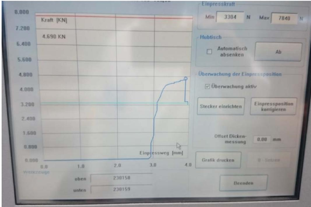
**Figure 25 –Press in force graph for connector A.**
