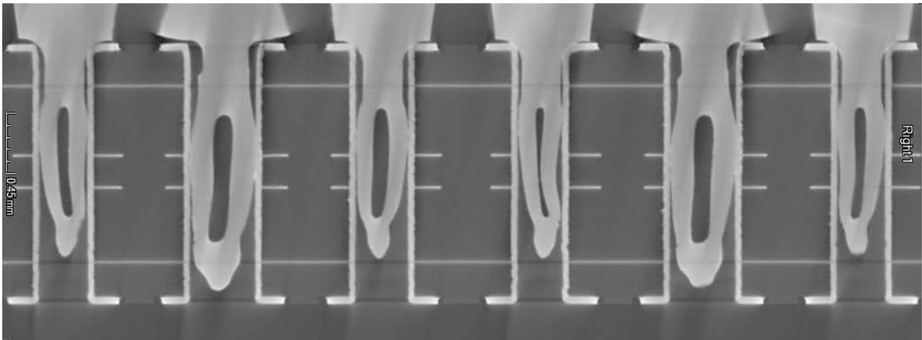
Figure 1 –3D CT x-ray image of deformed high speed pressfit connection pins<sup>1</sup>.
