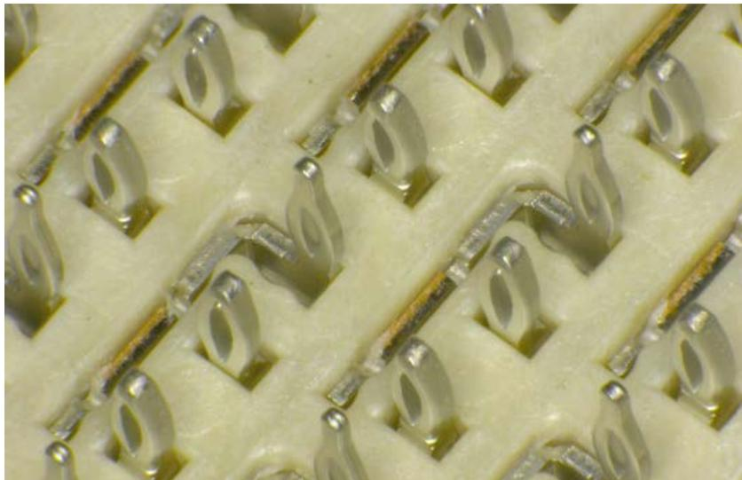
**Figure 2 – Press fit pins for high speed connector A<sup>2</sup>.**
