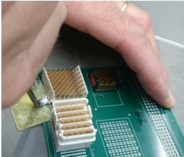
**Figure 28 –Removal of connector A.**
