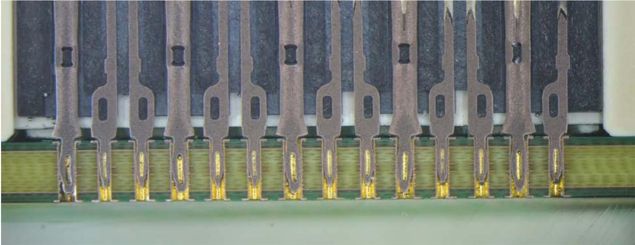
**Figure 54 – Vertical cross sectioning of connector B.**
