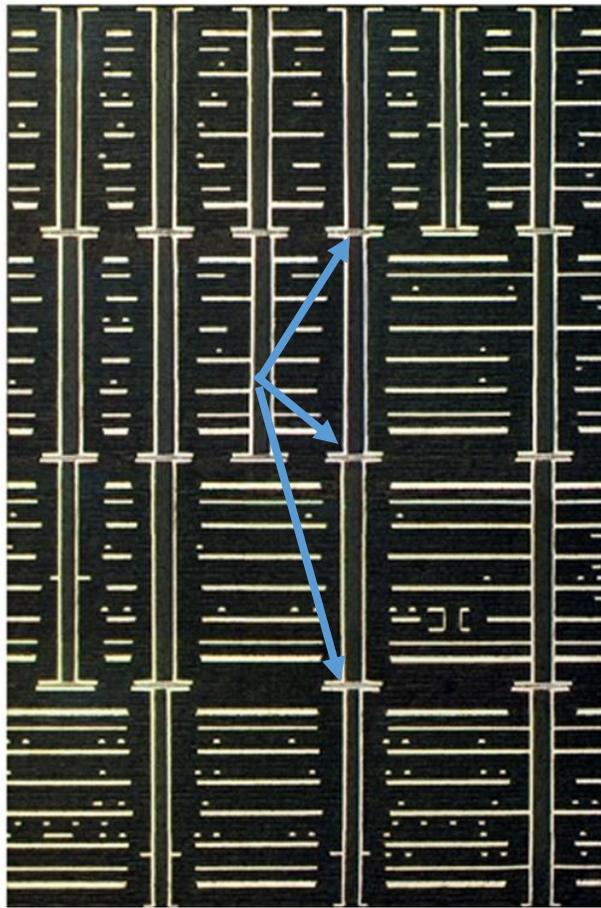
*Figure 9: A high-layer-count PCB broken into four cores and joined with sintering paste interposers [3]*
