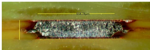
*Figure 17: Close up of a double via used to connect the two sides in the daisy chain pattern*
