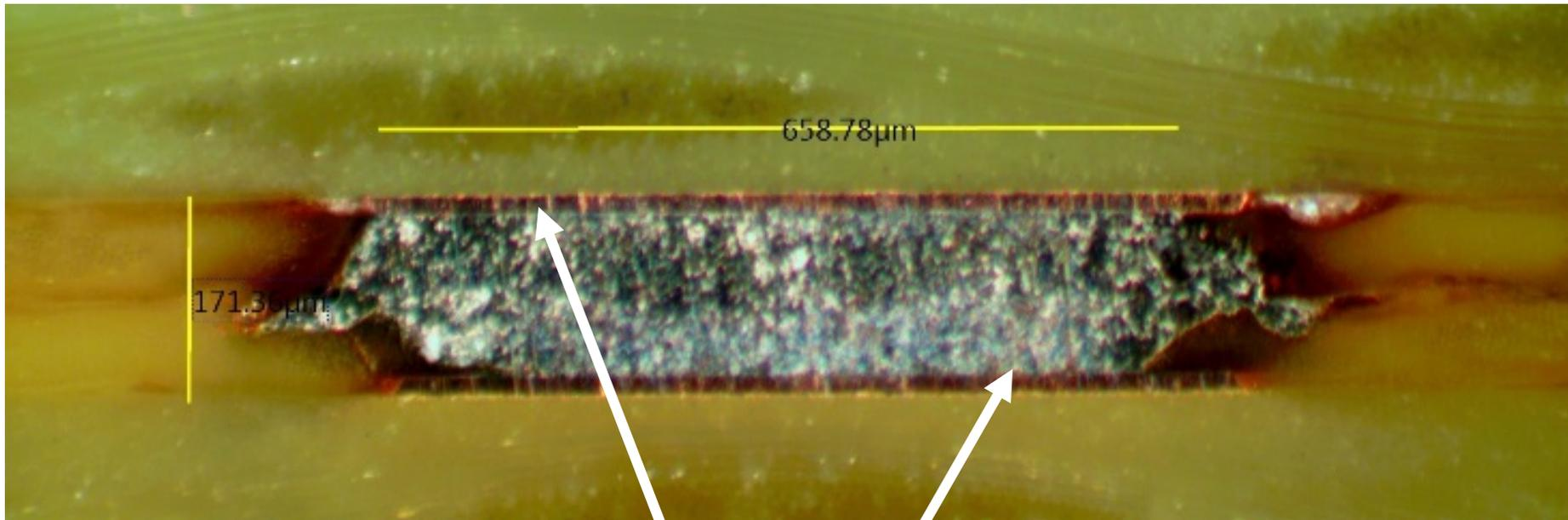
Good retention of via shape, consistent sintering throughout and to both interfaces
