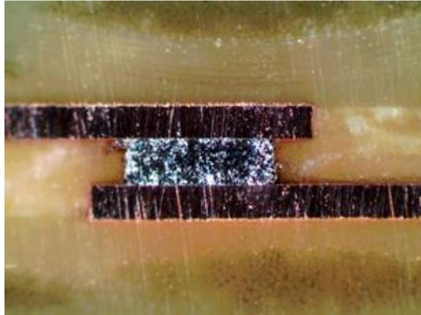
Figure 7: Detailed view of the sintered paste interconnect between copper pads on two cores
