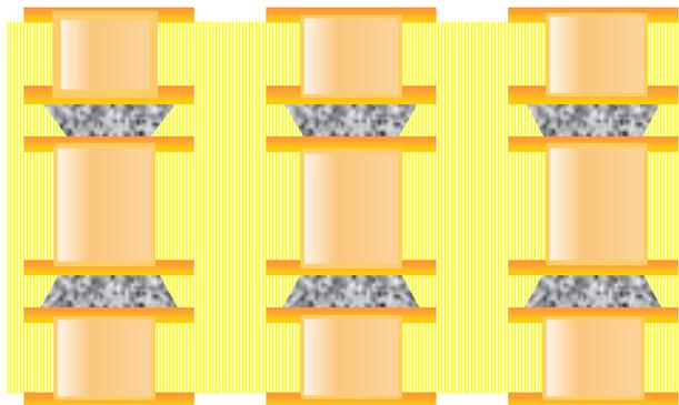
Figure 8: Illustration of core-to-core joining with sintering paste
