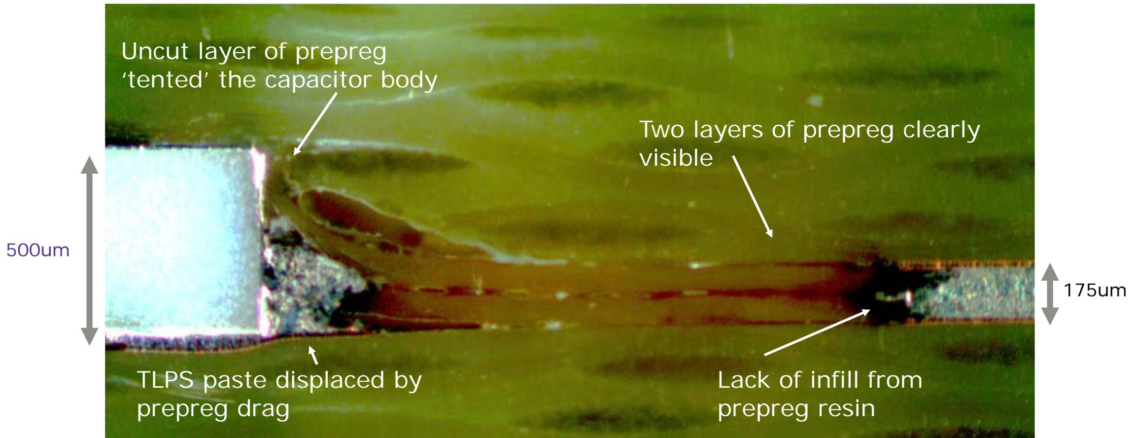
The TLPS paste installed into vias in opposing layers joined to form monolithic structures
