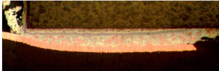
*Figure 16: Close up of the interconnection between a capacitor terminal and a copper pad*
