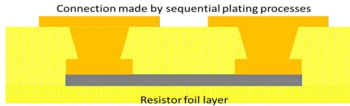
Figure 2: Concept of an embedded foil resistor
