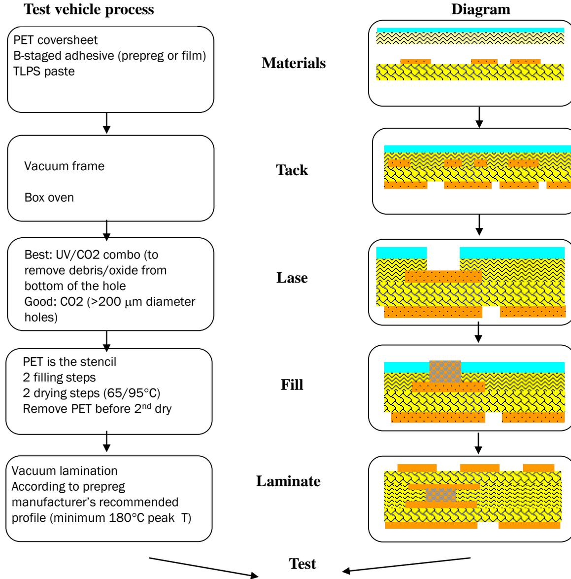
A typical process flow for implementing TLPS paste vias using the daisy chain test vehicle
