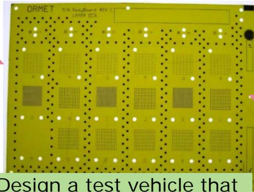
Design a test vehicle that captures the key features of the application.
