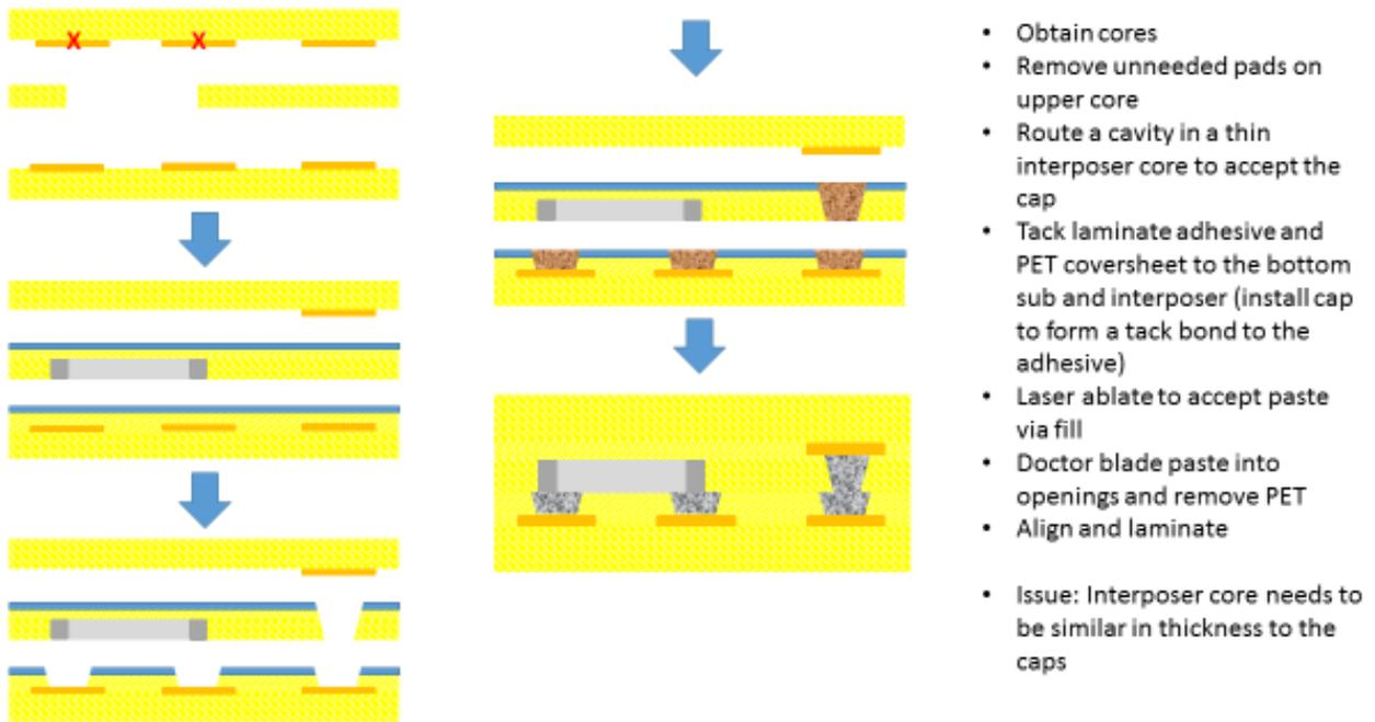
Figure 18: Revised test vehicle for embedding components in a PCB with TLPS paste joining layers
