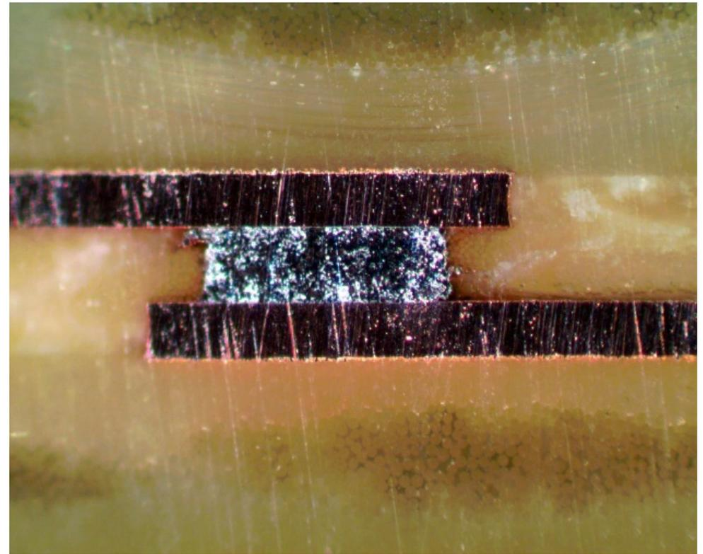
A ductile phase is built into the joint to manage the high CTE in the z-axis
