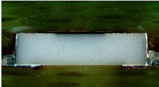
*Figure 1: 0805 capacitor embedded and interconnected with TLPS paste*
