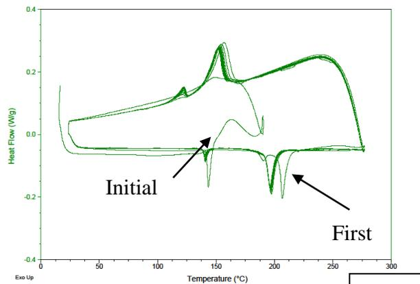
Figure 6: DSC signature of a TLPS reaction
