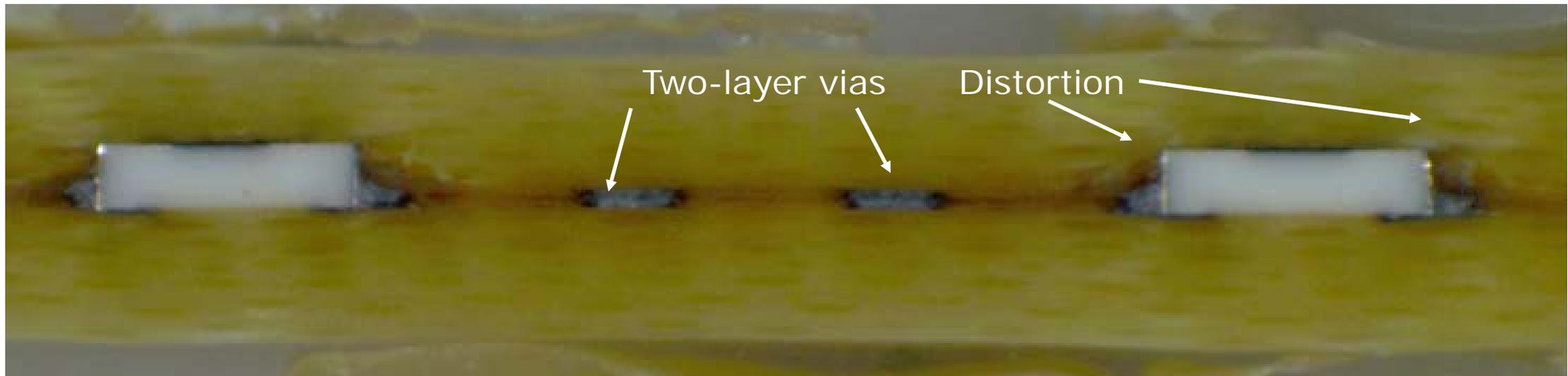
Despite the distortion and lack of in-fill of the prepreg resin, the TLPS joints maintained integrity and sintered well
