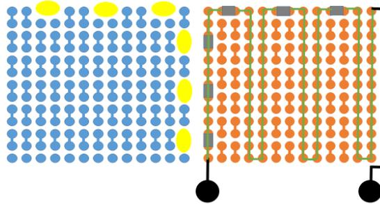
*Figure 13: Modified daisy chain for the test vehicle*
