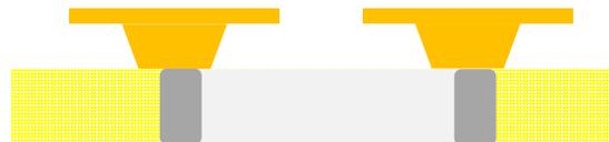
Figure 3: Discrete embedded capacitor concept
