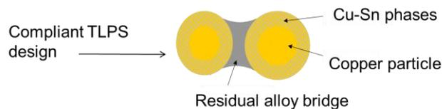
Figure 4: Conceptual view of a sintered TLPS interconnect
