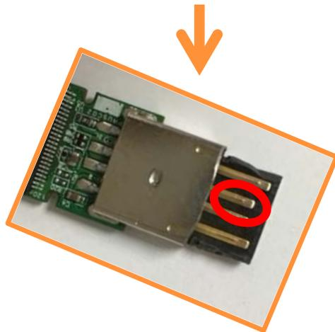
Water Contact Angle (WCA) measured in circled area
