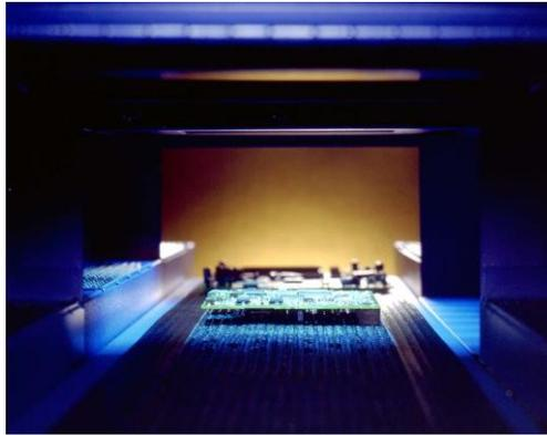
**Figure 3. Light Curing of Coatings in a UV-Conveyor**
