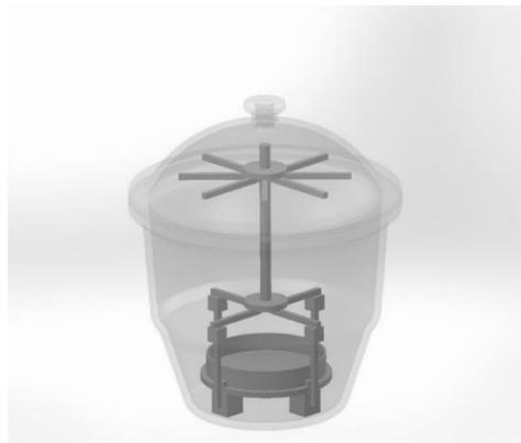
**Figure 4. Representation of a Flowers of Sulfur Test Chamber**
