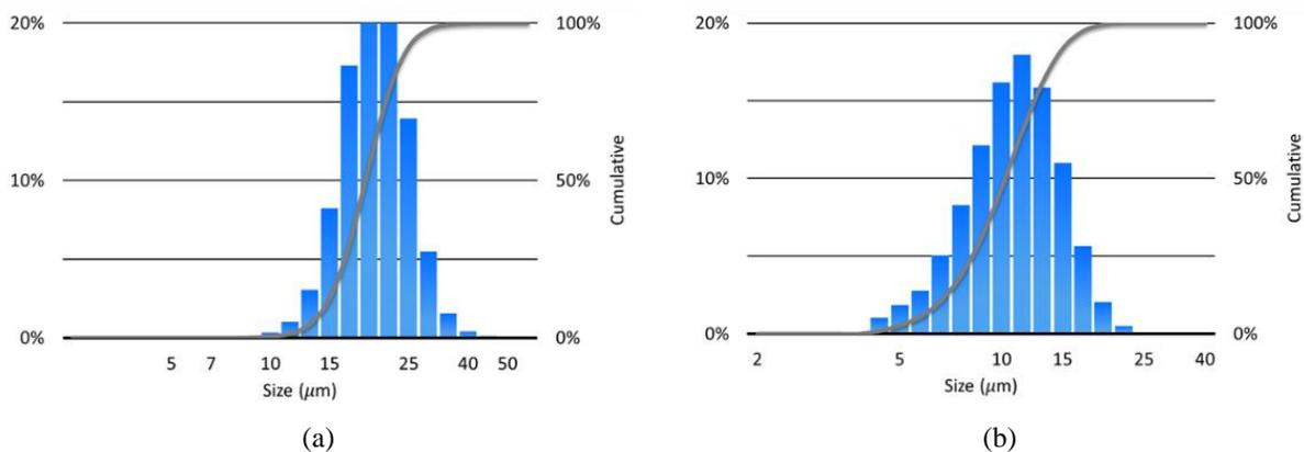
**Figure 2: Particle size distribution of powders: (a) Type 5, (b) Type 6.**
