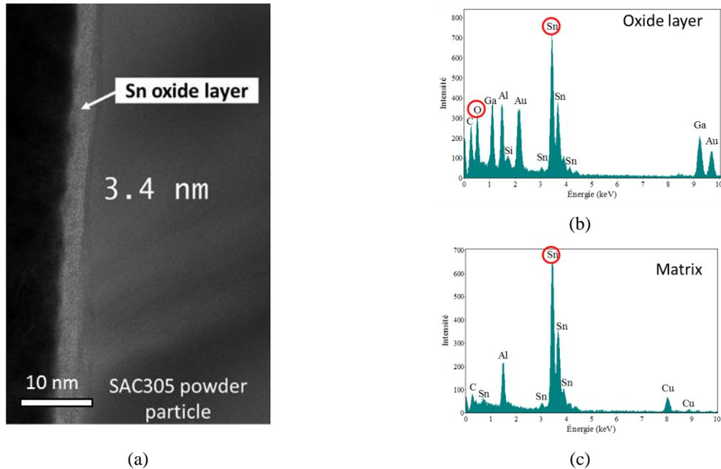
**Figure 4: TEM and EDS on the cross section of SAC305 powder, (a) the picture shows the oxide layer formed at the surface of powder, (b) EDS on the oxide layer, (c) EDS on the powder matrix. Presence of some elements are related to the sample preparation.**
