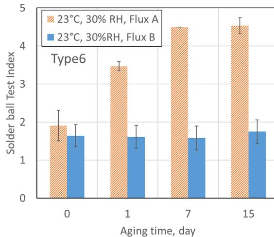
Figure 7: Solder Ball Test Index; SAC305 Type 6 powder with NC ROL0 fluxes: Flux A and Flux B.
