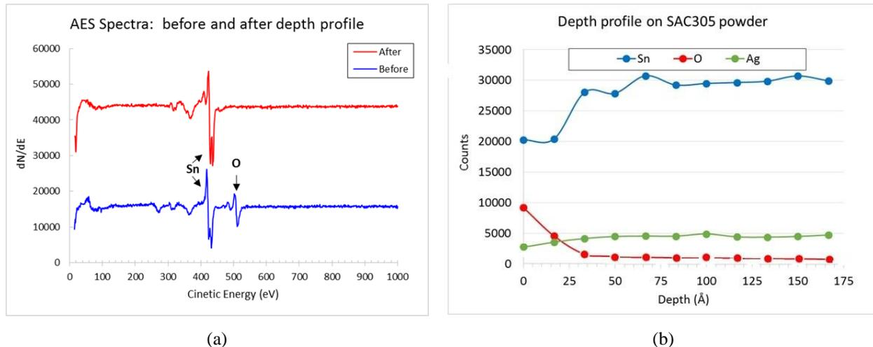
**Figure 3: Auger Electron Spectroscopy (AES) technique is used to characterize the surface oxide layer: (a) Auger spectra, (b) peak-to-peak height vs. depth which shows depth profile of elements. Depth=0 is the position at the surface of powder.**
