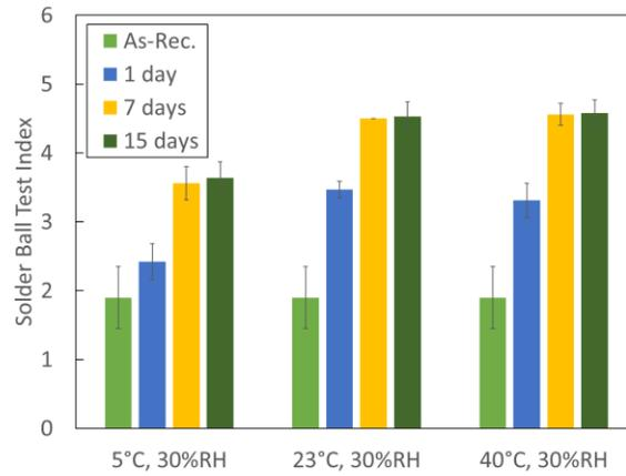
Figure 6: Effect of powder aging temperature on the reflow performance of the paste, Type 6, Flux A.
