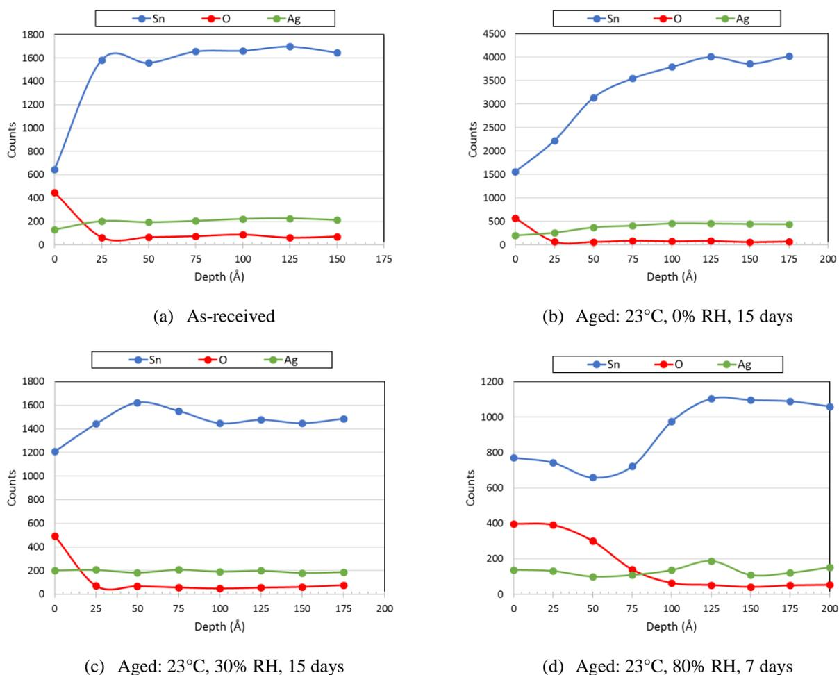
**Figure 8: Depth profile of elements by Auger Spectroscopy, oxygen curve is indicative of the oxide layer thickness at SAC305 T6 powder. (a) as-received, (b) Aged: 23°C, 0% RH, 15 days, (c) Aged: 23°C, 30% RH, 15 days, (d) Aged: 23°C, 80% RH, 7 days.**
