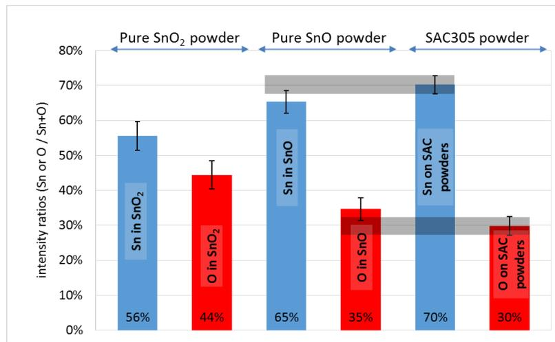
**Figure 10: Chemical composition of oxide measured using AES spectrum; the vertical bars show Sn and O concentrations estimated by peak-to-peak height in the AES spectrum. The first four bars show Sn and O concentrations in pure SnO<sub>2</sub> and pure SnO powders; the last two bars show Sn and O concentrations at the surface of SAC305 powder. SAC305 powder data are the average of measurements performed on powders aged under various aging conditions.**
