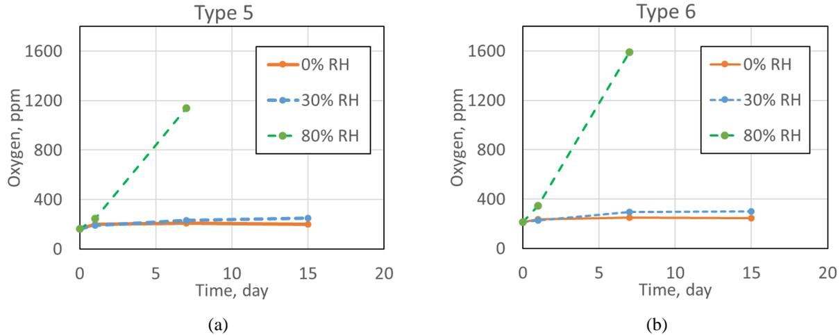
**Figure 9: Oxygen content of SAC305 powder aged at room temperature, (a) Type 5, (b) Type 6.**
