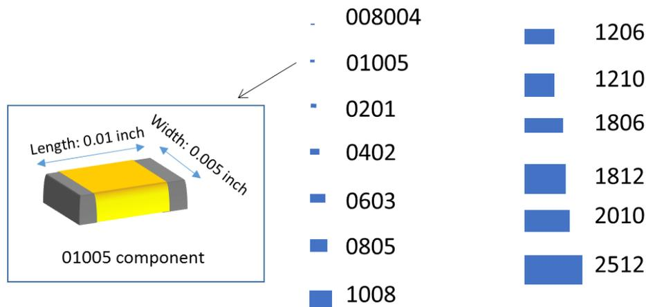
**Figure 1:** Example of component sizes and imperial codes.
