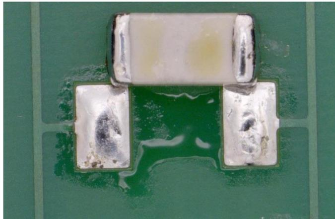
**Figure 3: Desoldering Components can cause flux residue to flow under the component termination**
