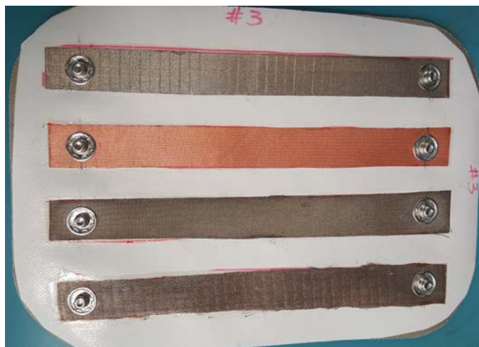
Conductive fabric laminated to denim patch
