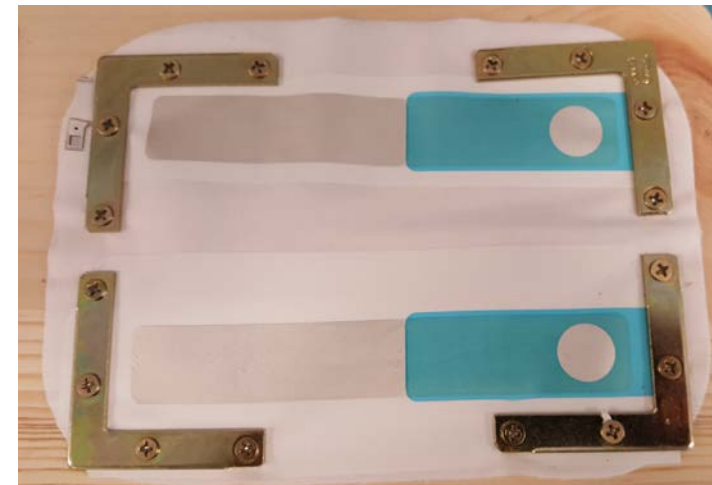
Conductive ink printed on TPU/laminated on denim, clamped on rigid board
