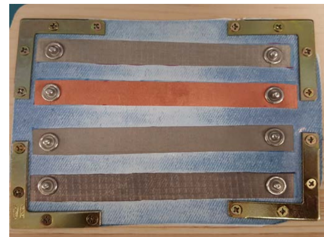
Conductive fabric laminated to denim patch then clamped on rigid board
