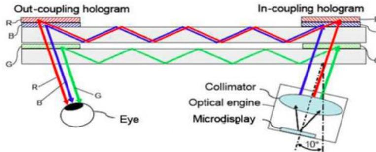
**Figure 2 - An illustration of a waveguide [1]**
