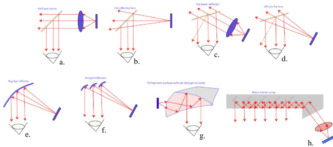
Figure 1 - Various types of combiners: a. Half tone mirror, b. Flat reflective lens, c. Flat beam deflector, d. Off-axis lens, e. Bug-Eye reflector, f. Arrayed reflectors, g. TIR free form surfaces with see through corrector, h. Micro-mirrors array [1]
