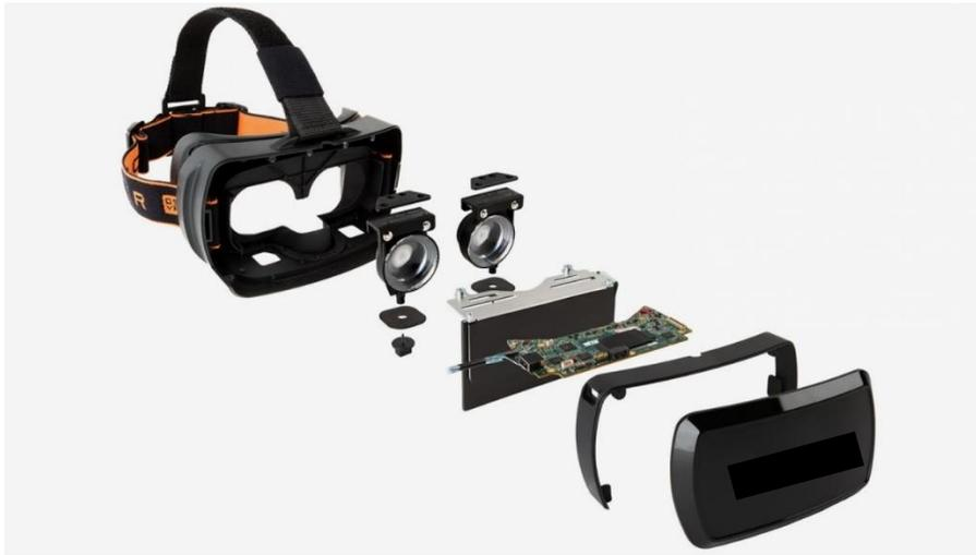
**Figure 4 - Various components of a Virtual Reality headset [3]**
