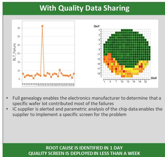
**Figure 2 – Data sharing dramatically improving time to identify root cause of issues**
