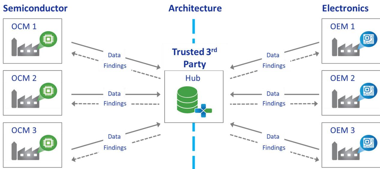
**Figure 3 – Concept of a quality protection service 3<sup>rd</sup> party solution**
