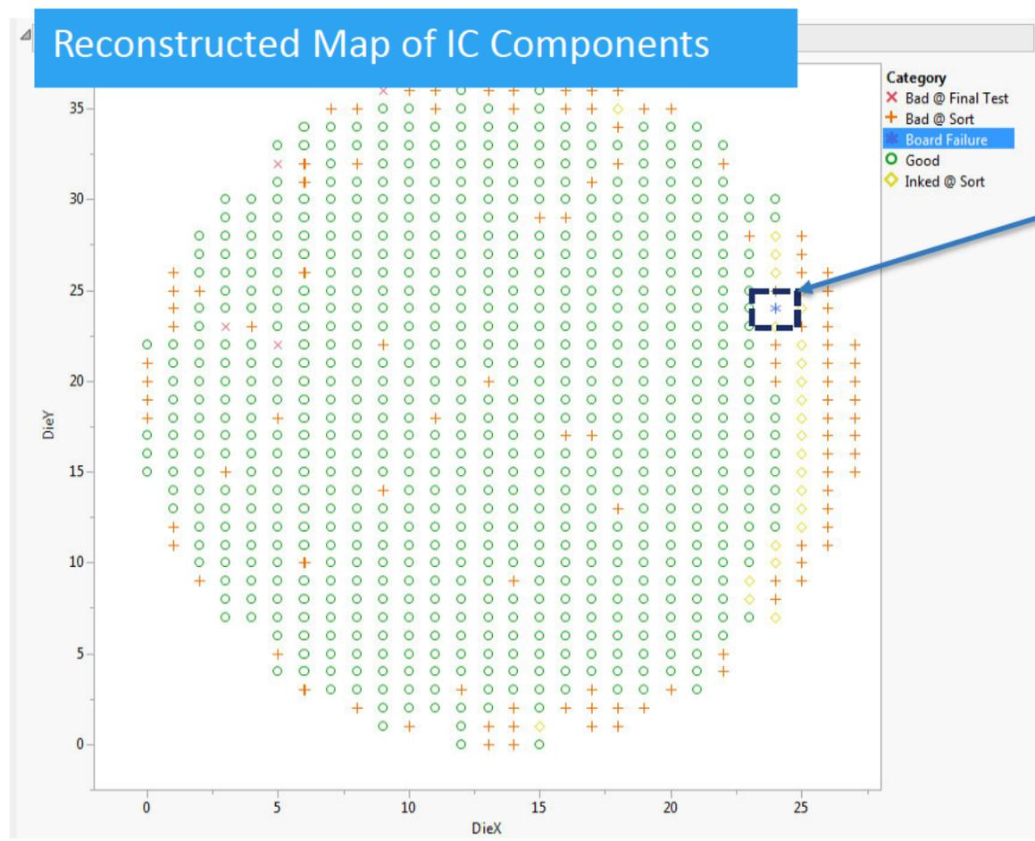
Board failure found adjacent to failing cluster at WS
