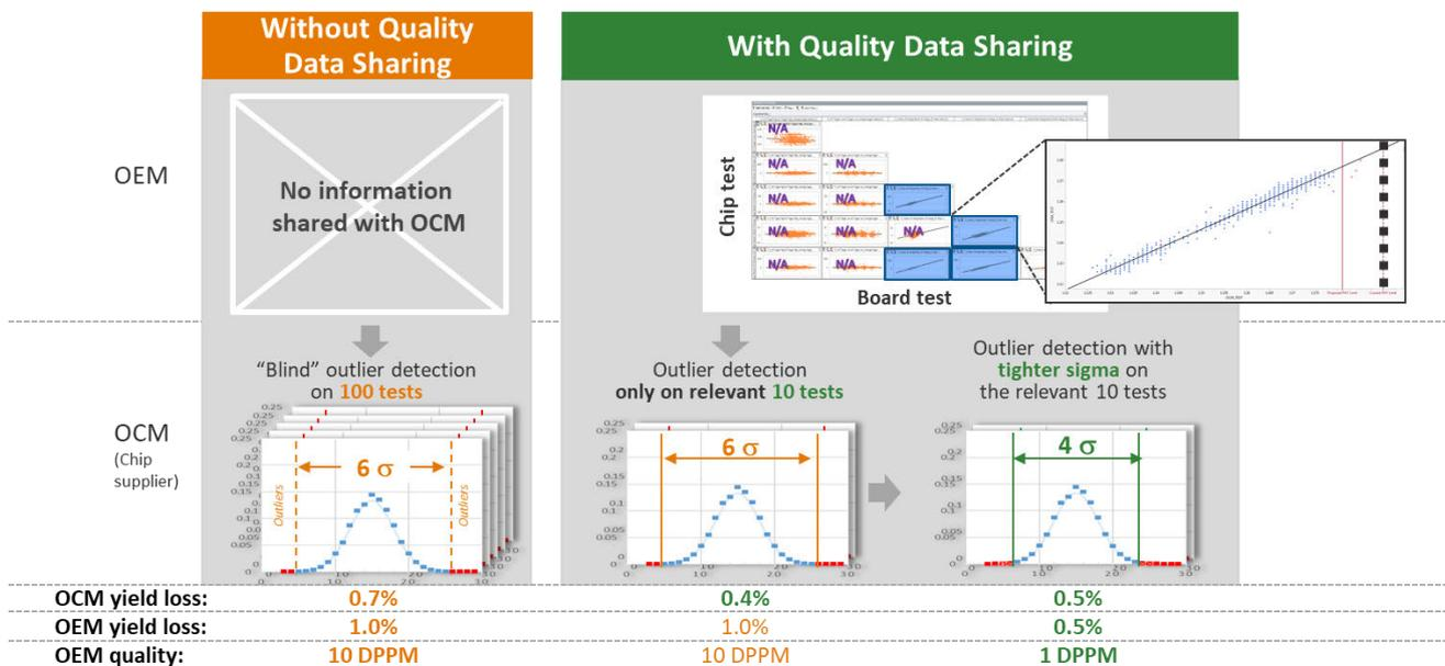
**Figure 4 – Win-Win for Supplier and Customer →Single Board Type per IC**
