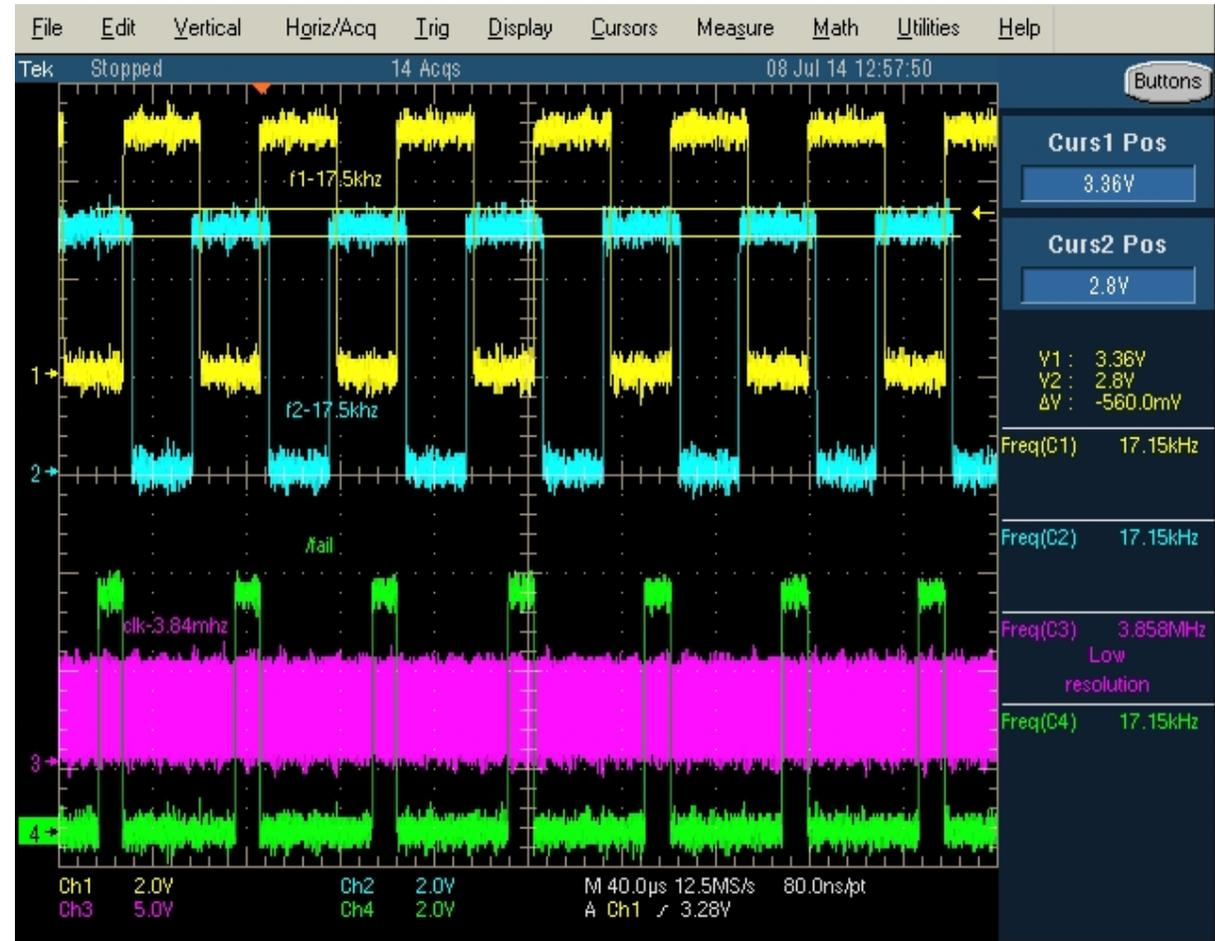
EPLD TIMING FAILURE
