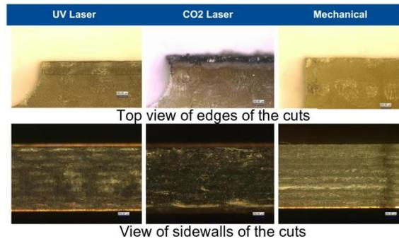
Figure 19 – Comparing cutting edges using various cutting methods
