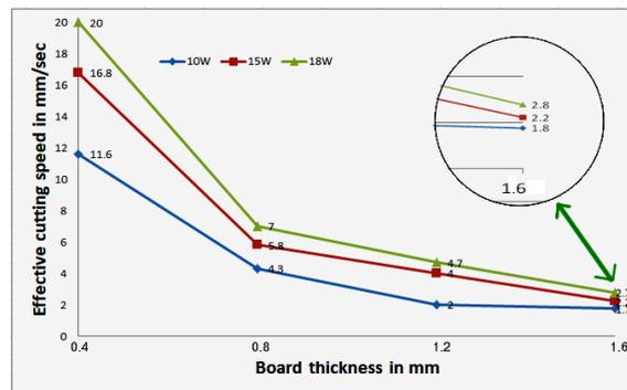
Figure 20 – Effective cutting speed for different FR4 thicknesses
