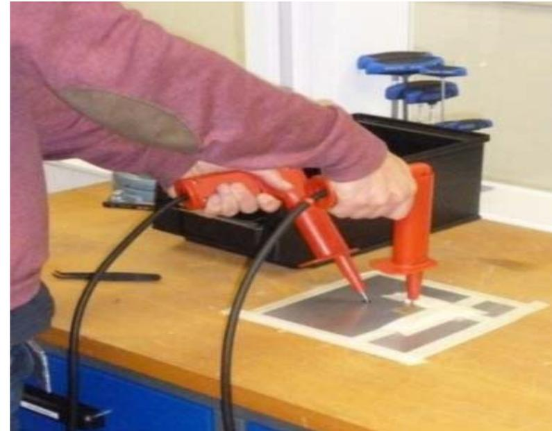
Measuring voltage breakdown
