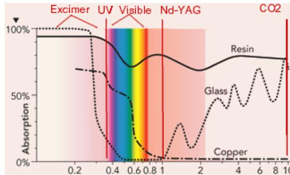
**Figure 1 - Energy absorption of common circuit board materials**
