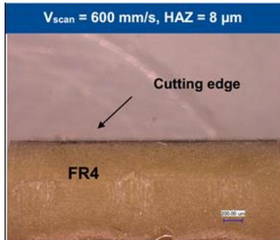
**Figure 17 – Sidewall showing virtually no charring**
