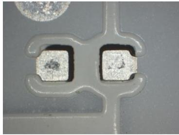
**Figure 12 – Coating with no fissures/cracks after 500 cycles -40/+125°C**
