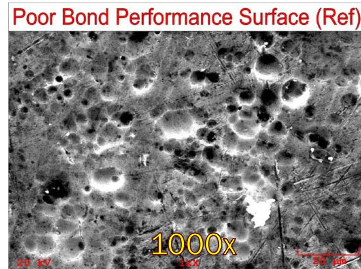
Deficient surface on right shows smoothed features at 1000x magnification (possibly due to chemical polish)
