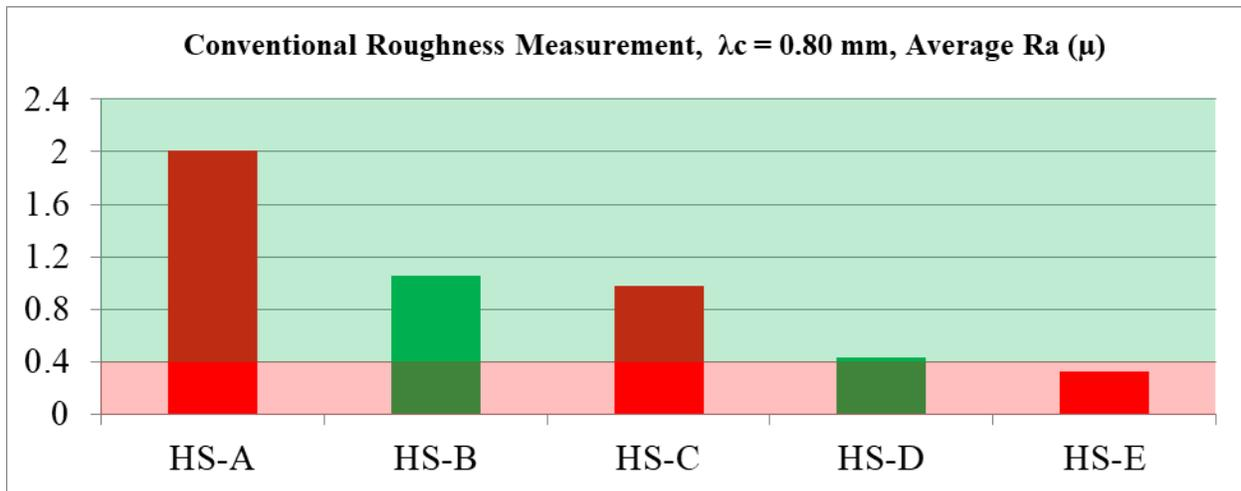
**Figure 2:** Standard Roughness Measurements for Heatsinks with Good / Poor Bond Performance
