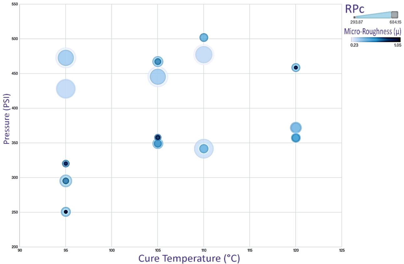
**Figure 17:** Interaction between Roughness and Cure Temperature
