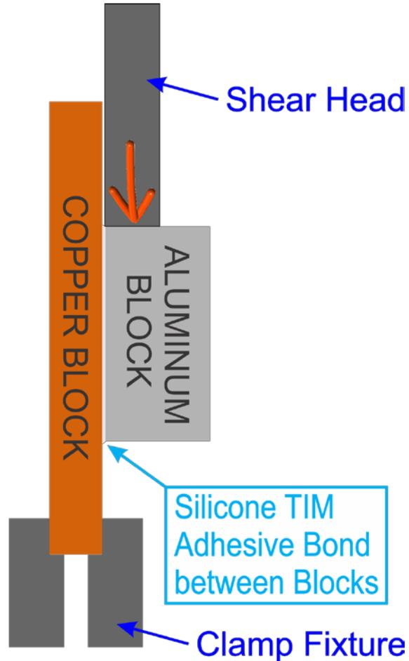
Shear test configuration
