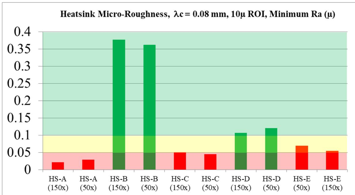
**Figure 1:**Micro-roughness Measurements for Heatsinks with Good / Poor Bond Performance
