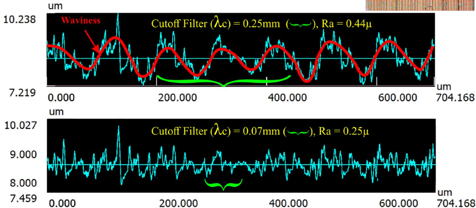
Top chart [ $\lambda_c = 0.25\text{mm}$ ] has substantial waviness, Lower chart ( $\lambda_c = .07\text{mm}$ ) shows roughness only
