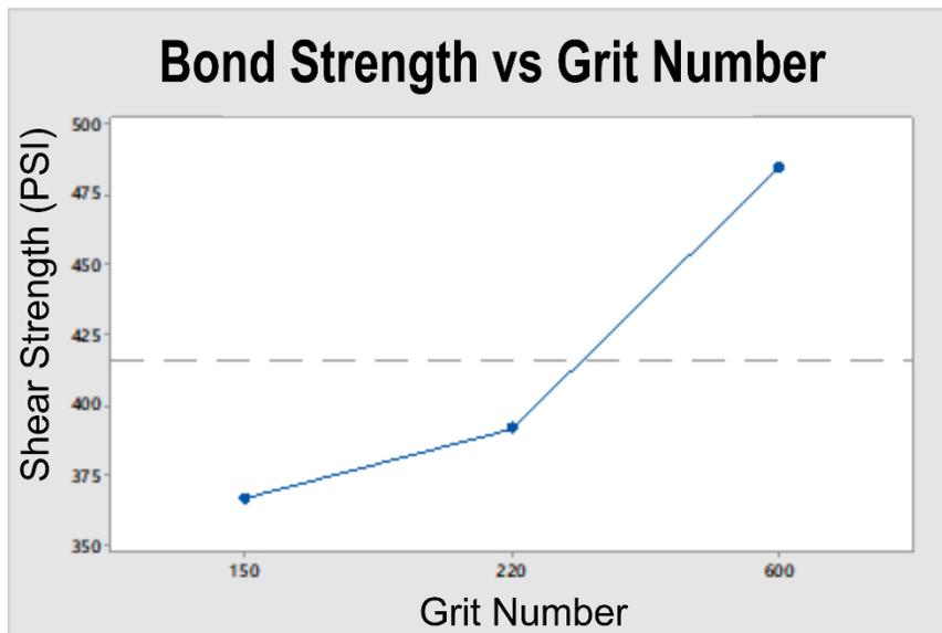
Figure 15: Bond Strength as Function of Grit
