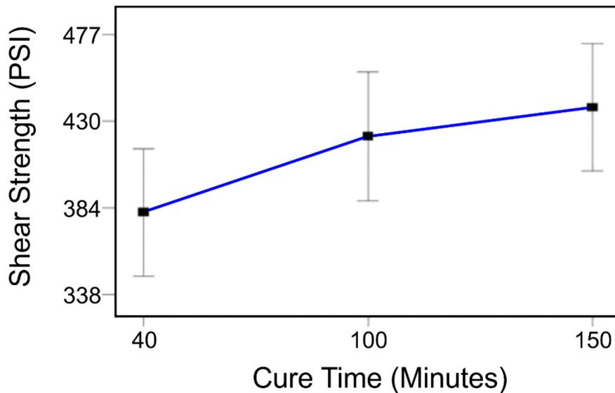
**Figure 13:** Bond Strength as a Function of Cure Time
