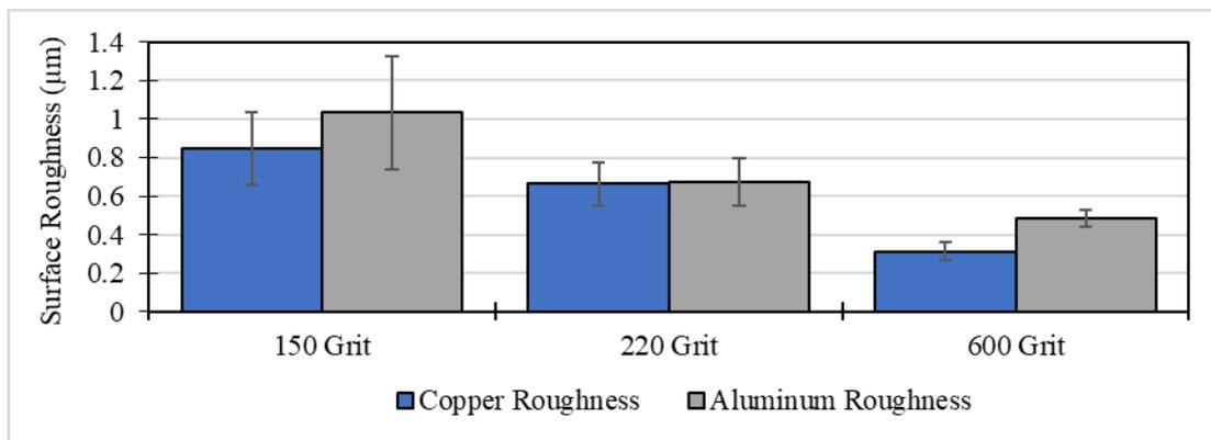
**Figure 3:** Histogram of Average Surface Roughness for Each Metal Sample
