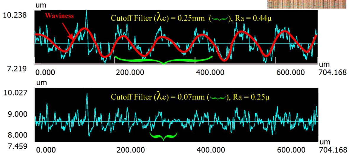
**Figure 4:** Examples of Waviness and Roughness Profiles
