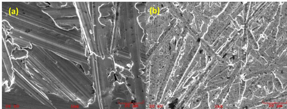
Figure 9: SEM Images of (a) 150 Grit Copper and (b) 600 Grit Copper
