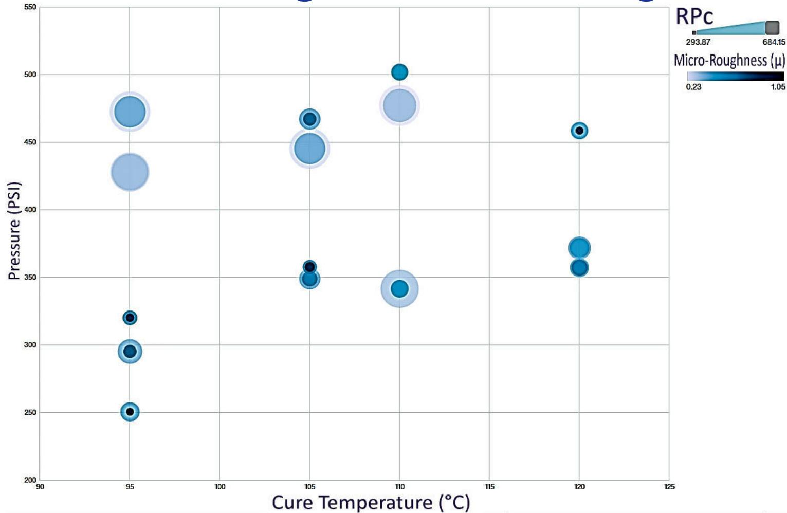
At lower cure temperature (95°C), Higher RPC maintains high shear strength
