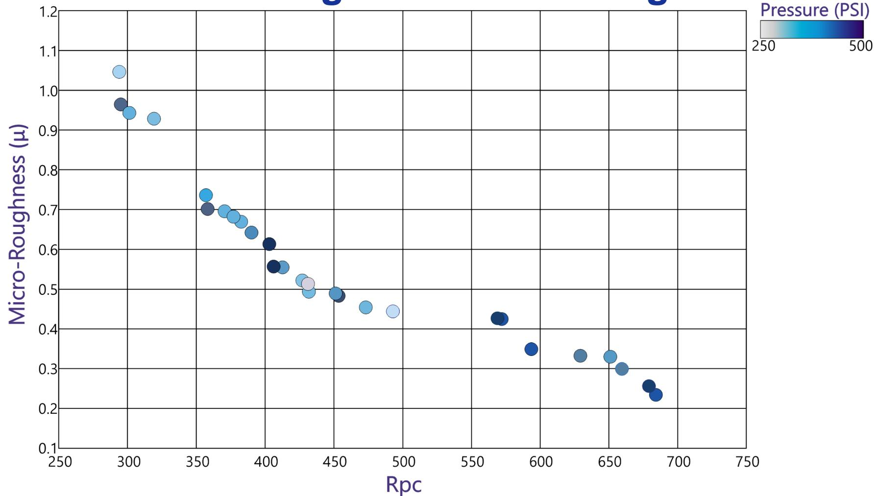
Higher R<sub>Pc</sub> and lower Roughness (Ra) tended to produce highest shear strength
