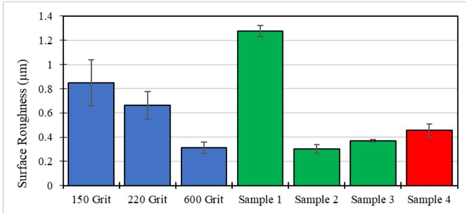
**Figure 10:** Histogram Comparing Surface Roughness between Each Grit Level and the Heatsink Samples
