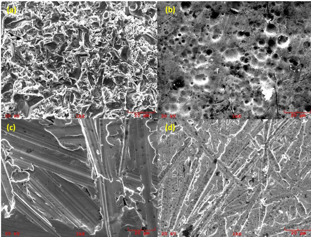
**Figure 12:** SEM Images at 1000x Magnification of (a) Heatsink Sample 1 (b) Heatsink Sample 4 (c) 150 Grit Cu Sample (d) 600 Grit Cu Sample
