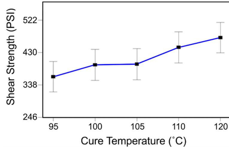
Higher grit number, higher cure temperature and higher cure time improved shear strength
