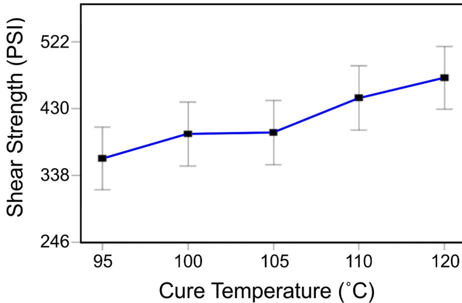
**Figure 14:** Bond Strength as a Function of Cure Temperature
