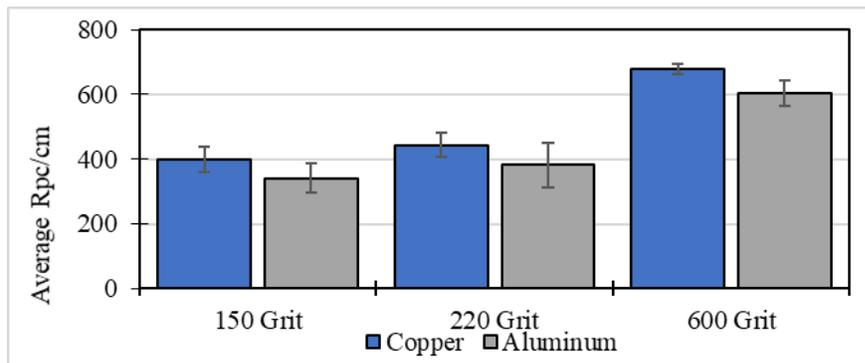
**Figure 7:** Histogram of Average Peak Count for Each Metal Sample
