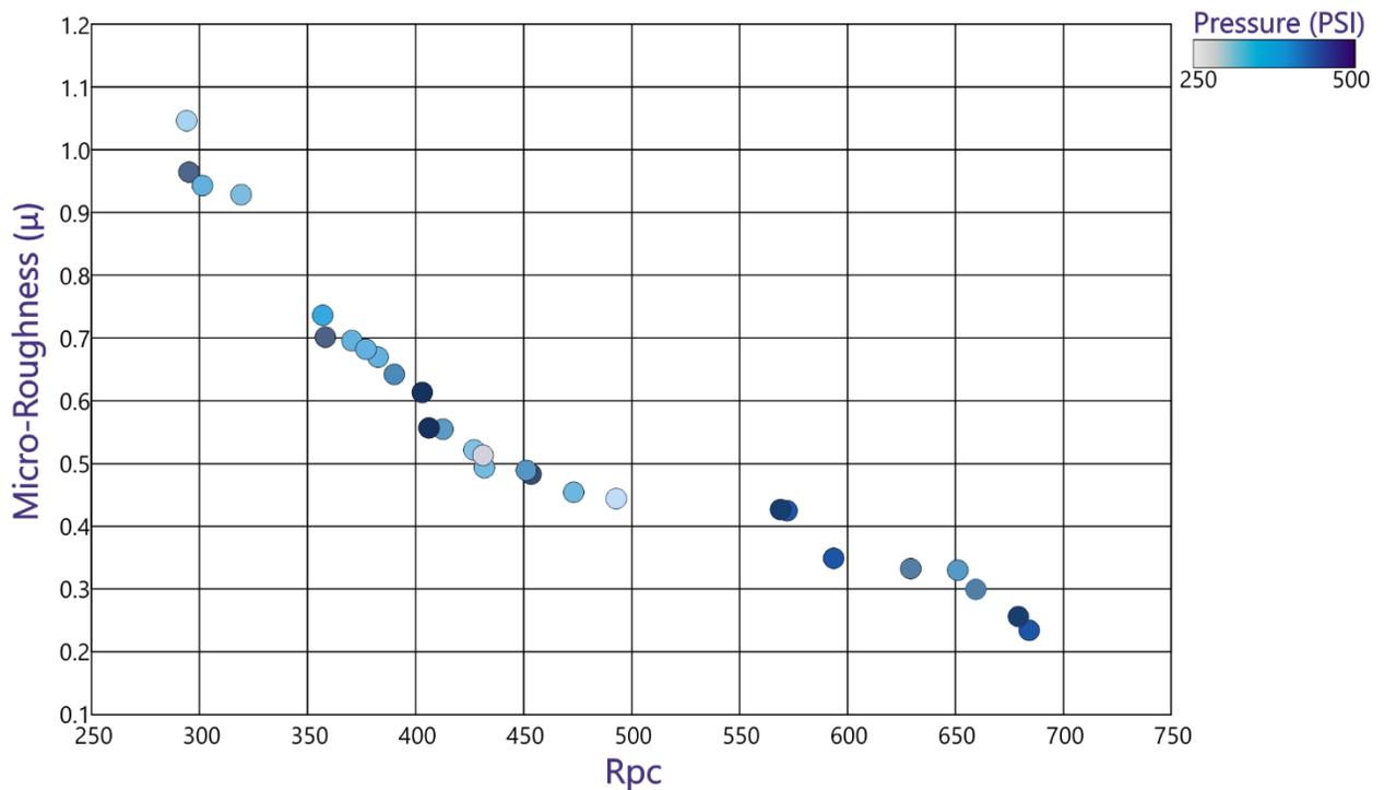
Figure 16: Pressure as a Function of Micro-Roughness and Peak Count
