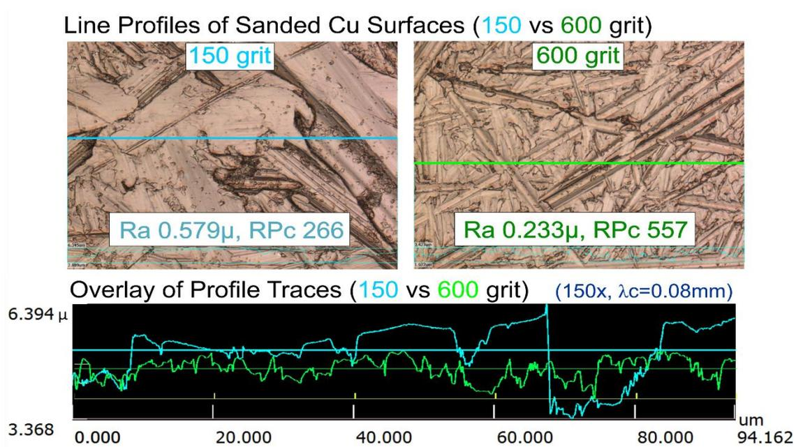
**Figure 6:** Line Profiles (150x Magnification) Showing Higher Number of Peaks and Valleys with Higher Grit Number
