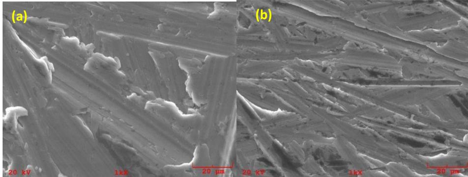
Figure 8: SEM Images of (a) 150 Grit Aluminum and (b) 600 Grit Aluminum
