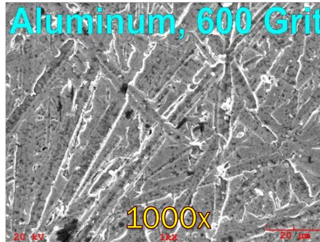
Courser grit shows large scale surface deformation, with higher smearing / fold-over
