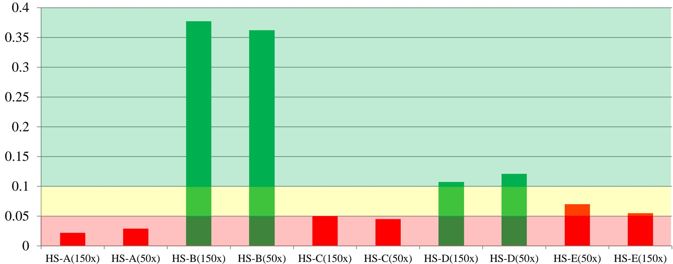
Poor performing heatsinks (Red Bars) had micro-roughness between .02 and .08 $\mu$
