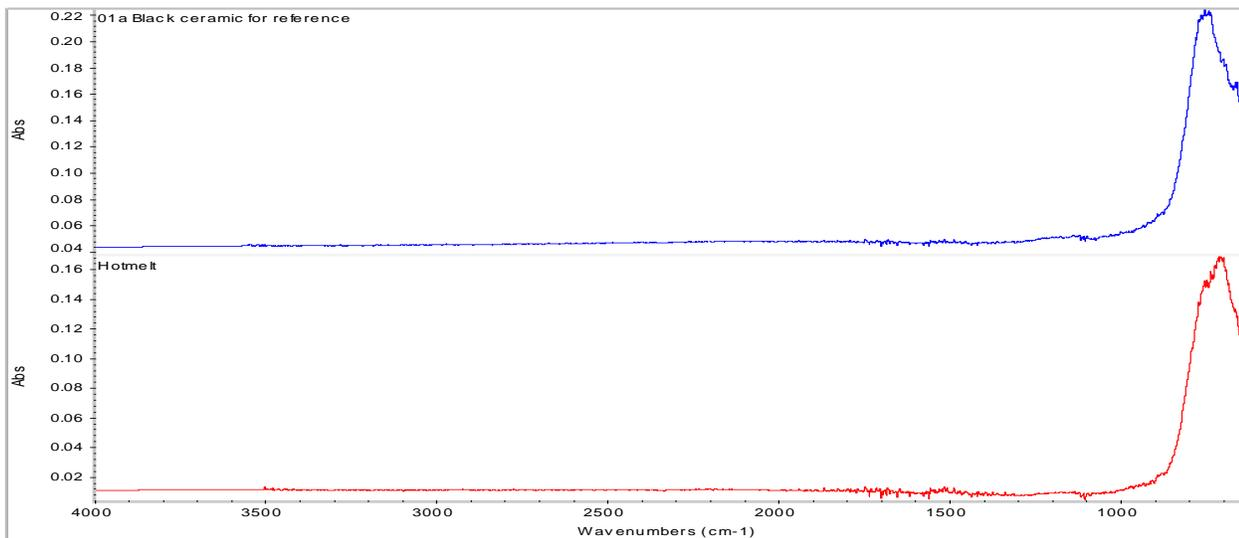
**Figure 11- FTIR Spectrum of Hotmelt**
