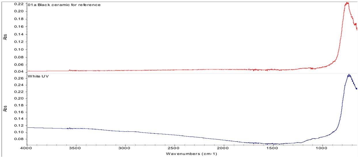
Figure 9- FTIR Spectrum of UV White
