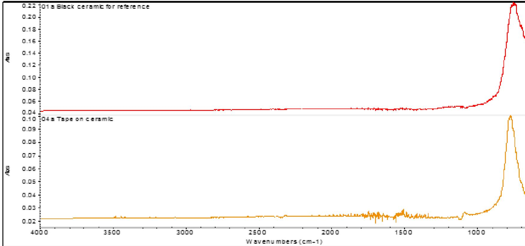
Figure 7- FTIR Spectrum of Tape
