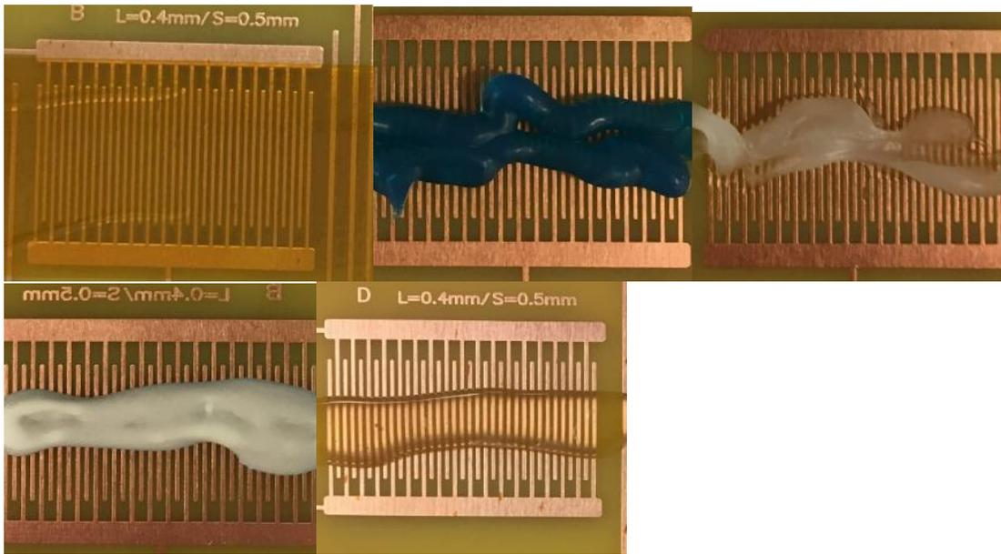
**Figure 2-Masking Material Applied to Bare SIR boards**
