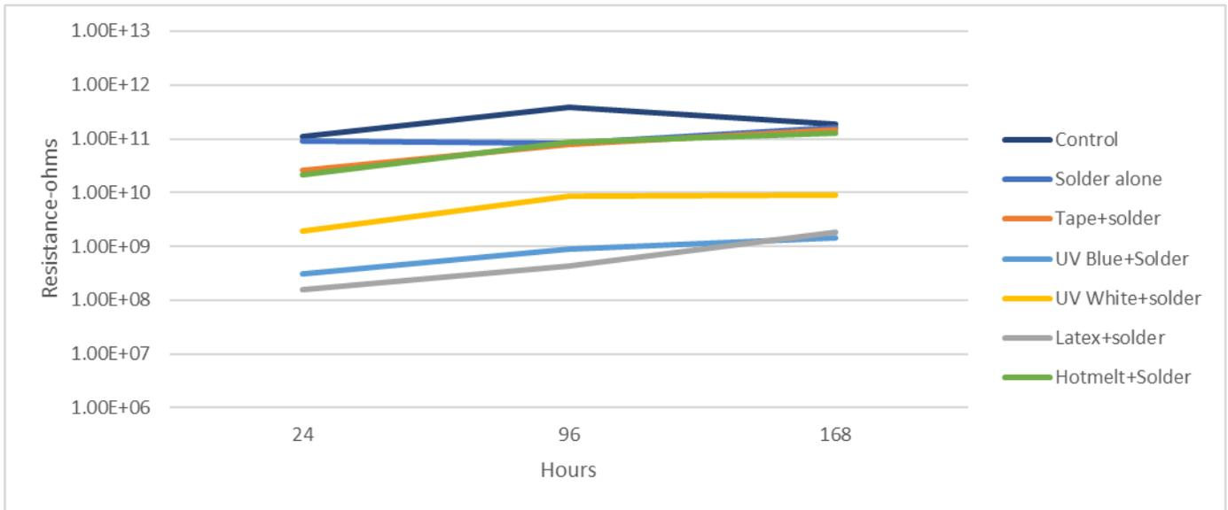
Figure 6-Mask Material and Solder Paste Residue on SIR Board
