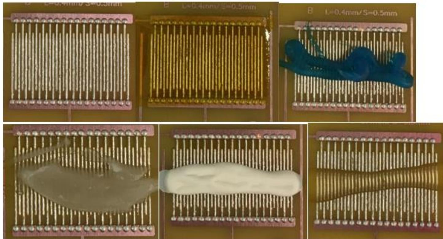
Figure 3- Masking Material Applied to Soldered SIR Boards
