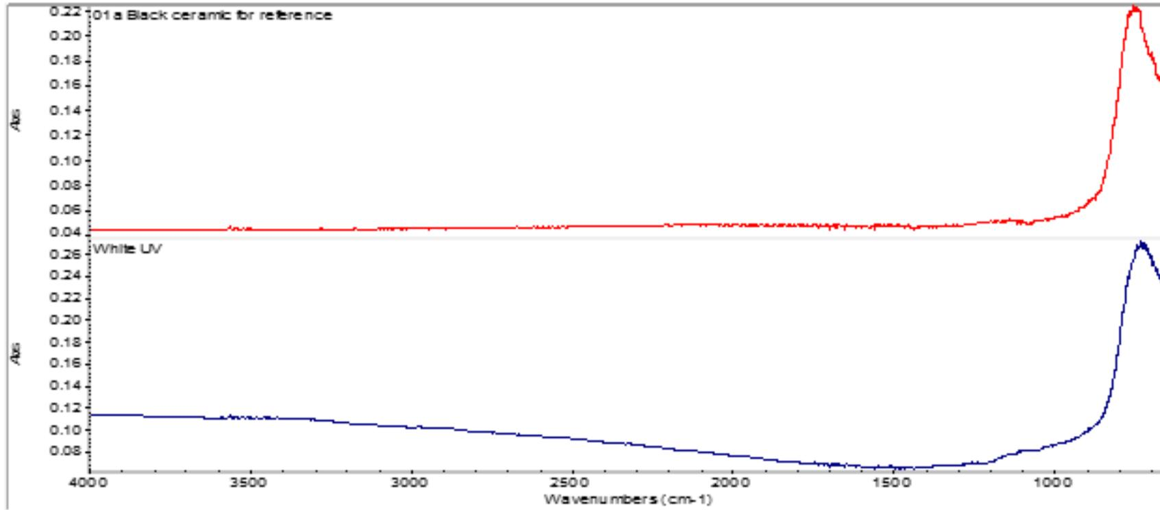
Figure 9- FTIR Spectrum of UV White
