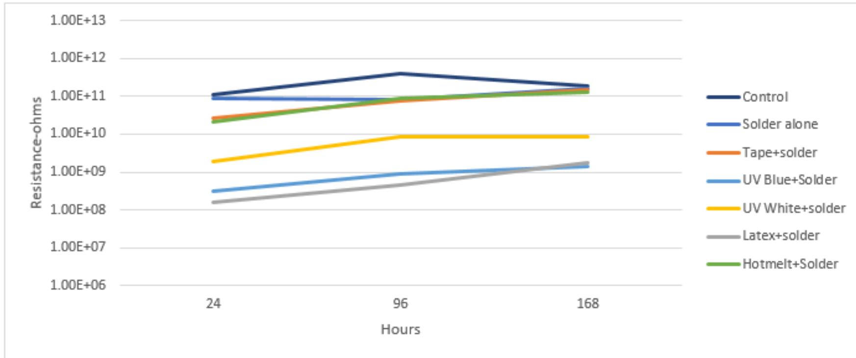
Figure 6-Mask Material and Solder Paste Residue on SIR Board
