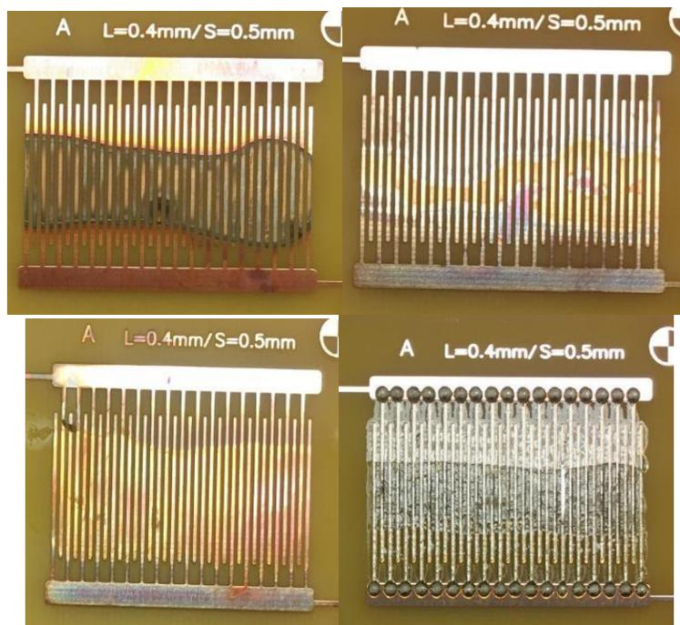
**Figure 12- Test Patterns after SIR testing of Latex (upper left), UV Blue (upper right), UV White (lower left) and Latex+Solder (lower right)**
