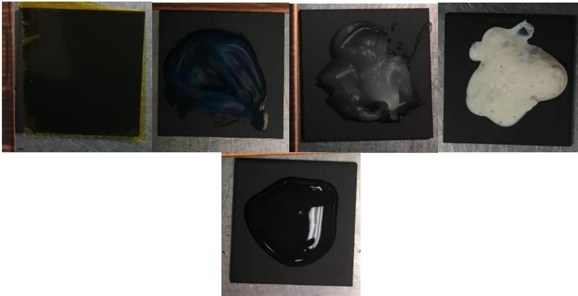
**Figure 4- Masking Material Applied to bare ceramic**
