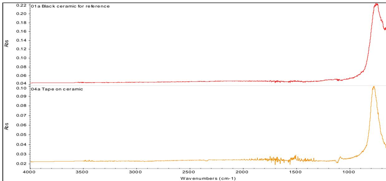
Figure 7- FTIR Spectrum of Tape
