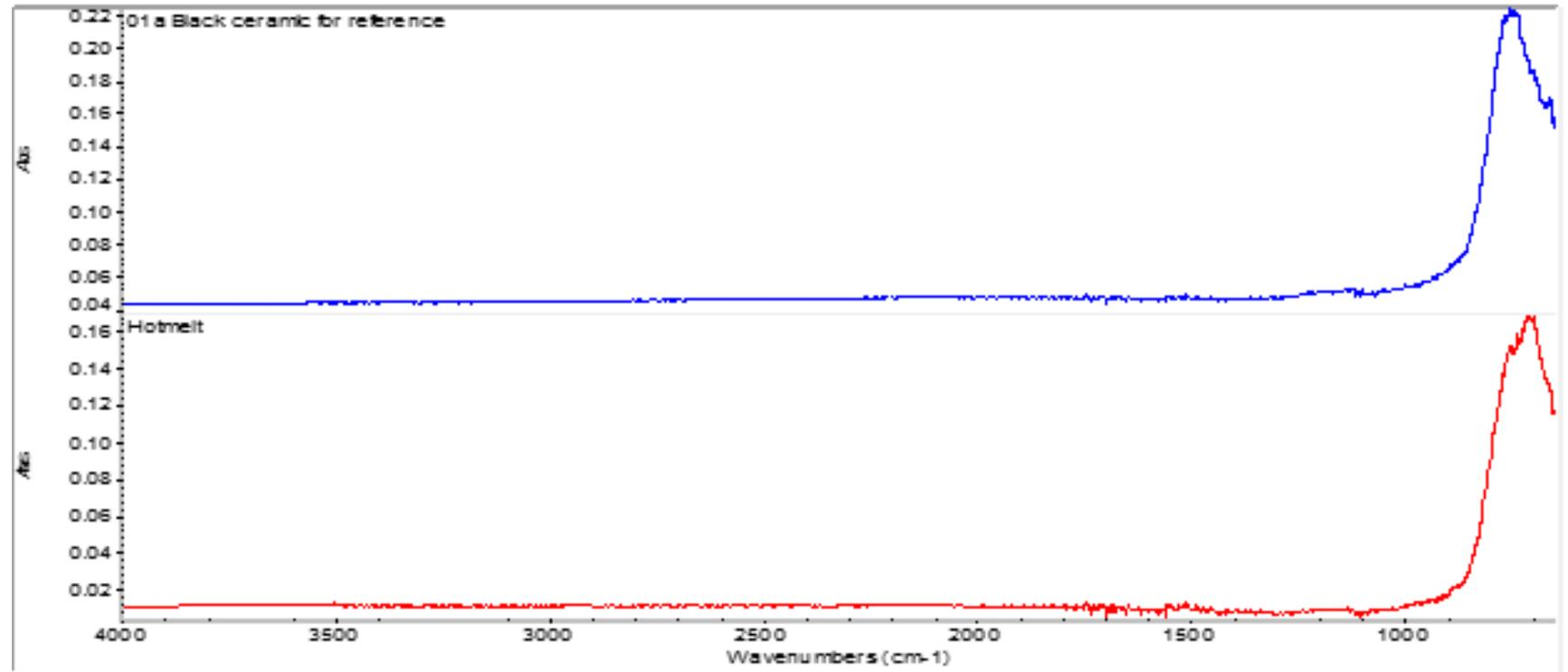
Figure 11- FTIR Spectrum of Hotmelt
