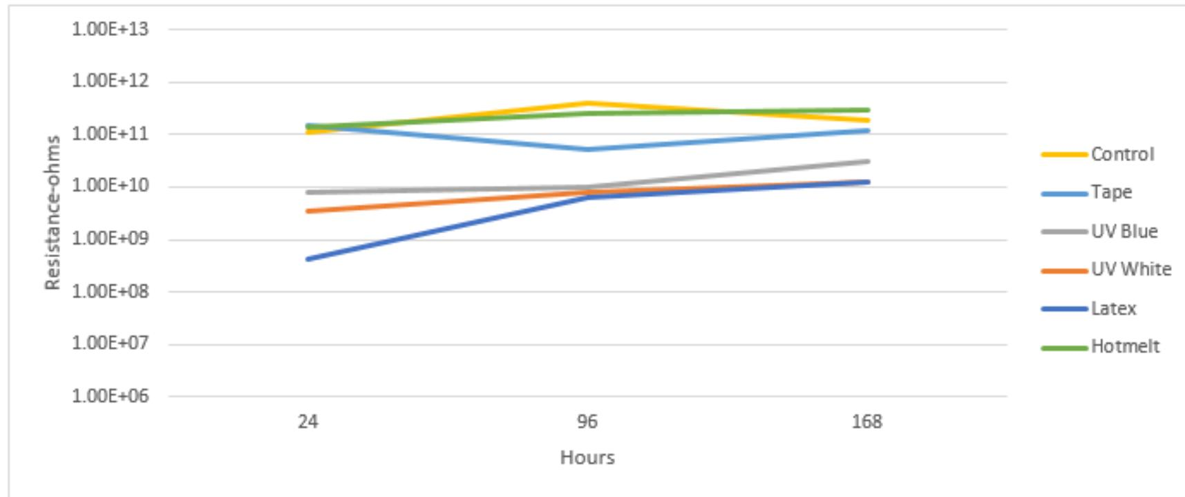
Figure 5- Mask Material on bare SIR board
