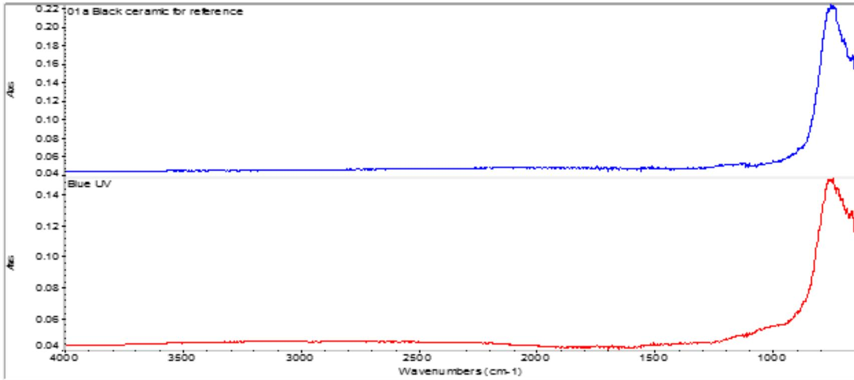
Figure 8- FTIR Spectrum of UV Blue
